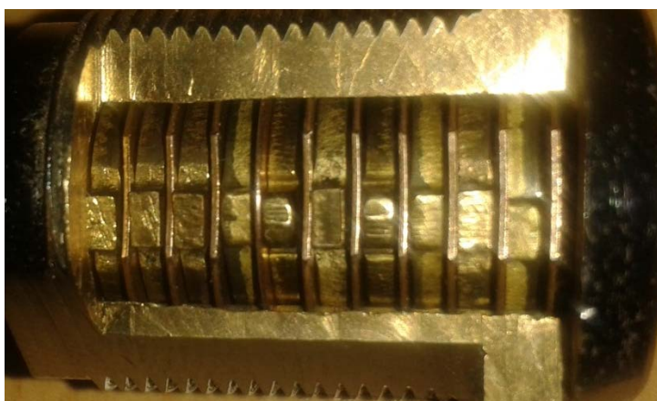
Fig 2.3 The disc pack, their tabs and washers.
