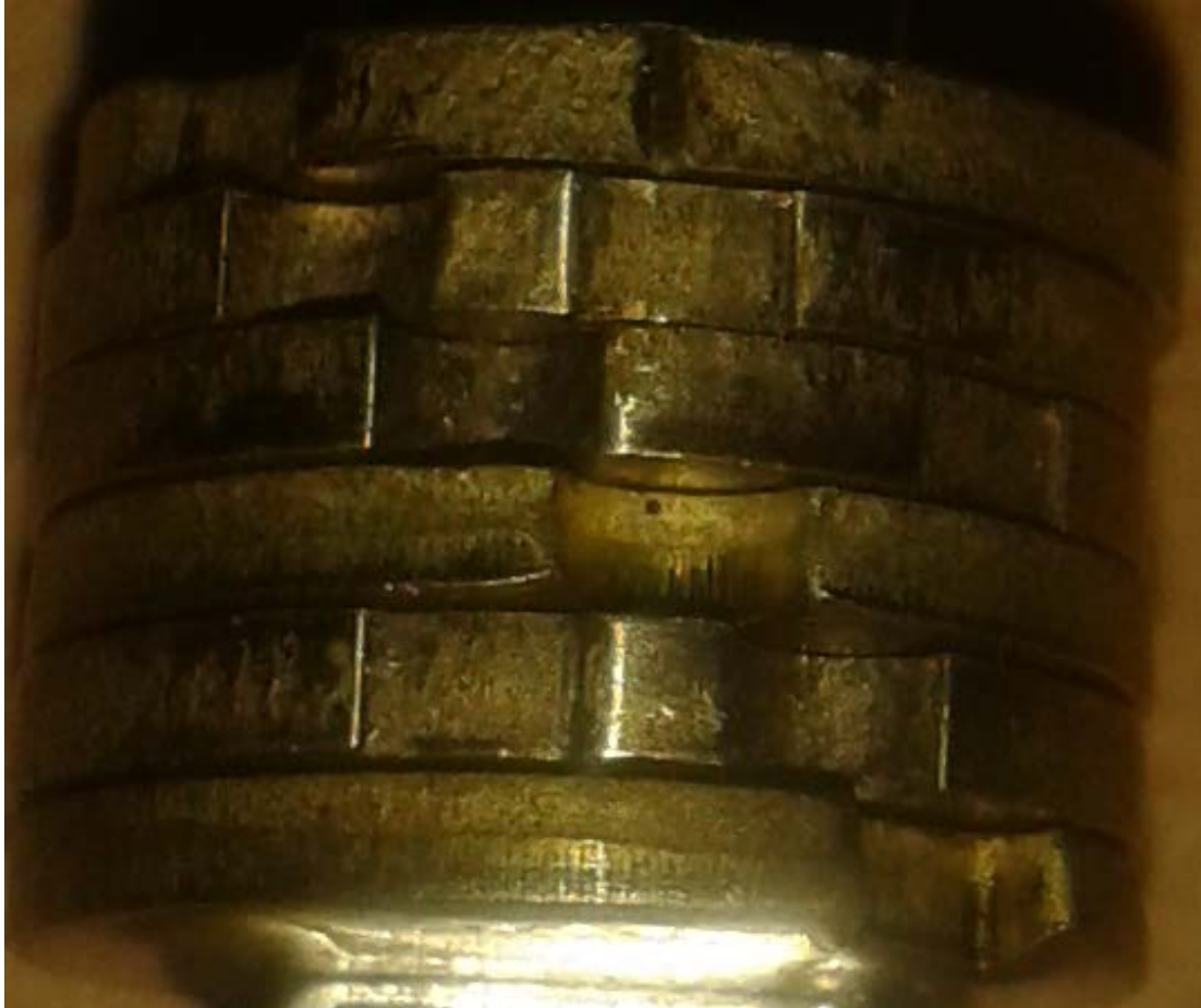
Fig 2.7 A close up showing real and false gates.
