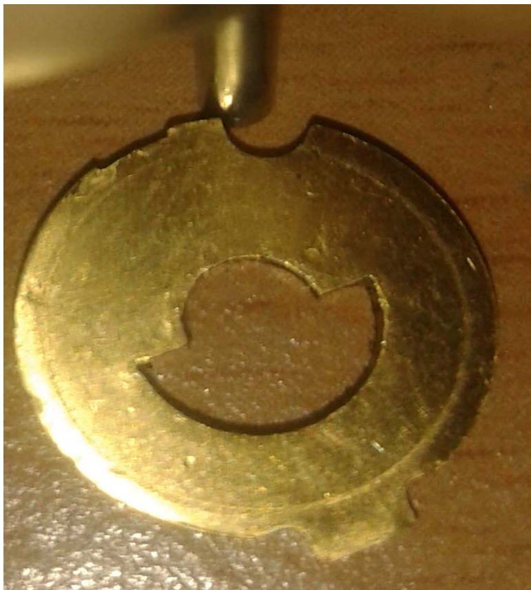
Fig 3.4 Round sidebar misaligned with round gate.
