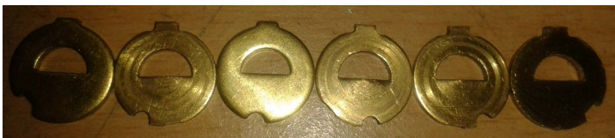
Fig 2.2 The six possible Classic gate positions.
