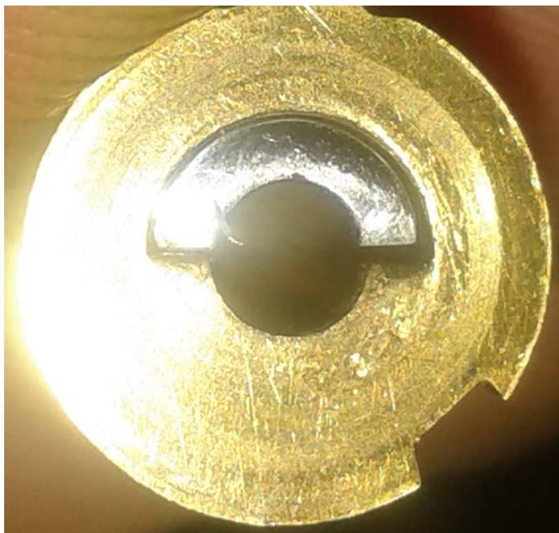
Fig 3.3 The picking head profile of the 'Ablator'- The Abloy Classic pick- avoiding the anti-pick discs.
