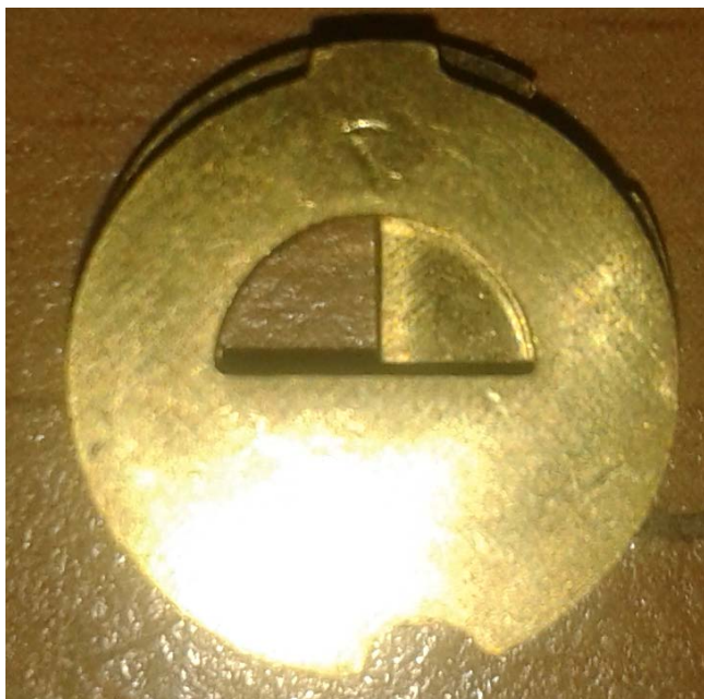
Fig 2.11 The maximum range of travel allowed for the Abloy Classic.
