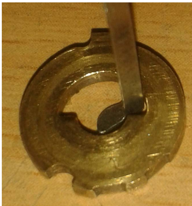
Fig 2.10 The tip of the H&H tool being defeated by an anti-pick disc. 16
