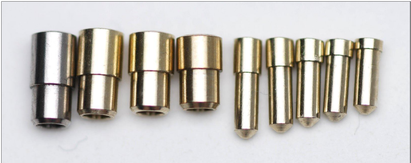
FIGURE 7.14: MT5/MT5+ key pins, sizes A-D (left) and 1-5.
