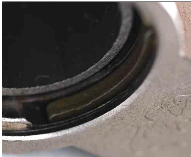
FIGURE 7.19: Anti-drill disc placed in the MT5/MT5+ cylinder, above the plug.
