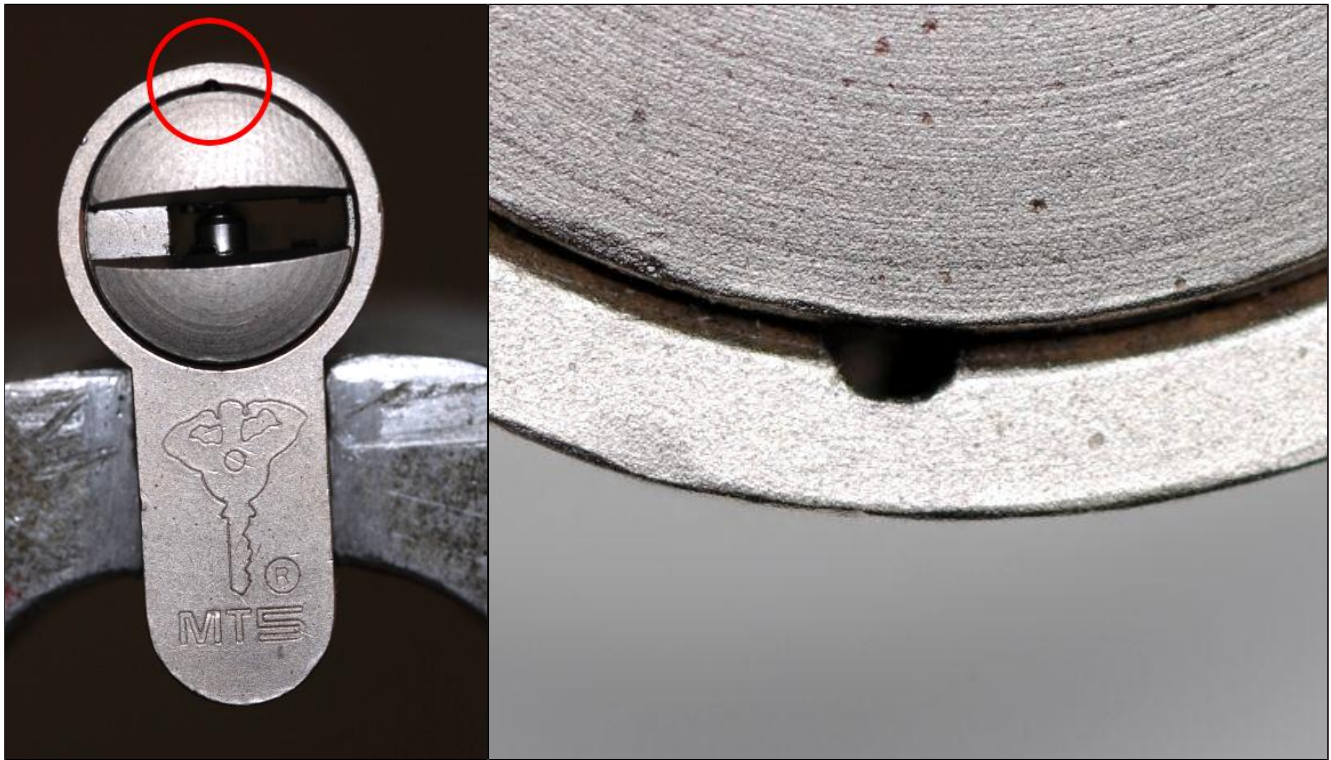
FIGURE 8.8: Normal and close-up views of the extended sidebar slot on European profile cylinders.
