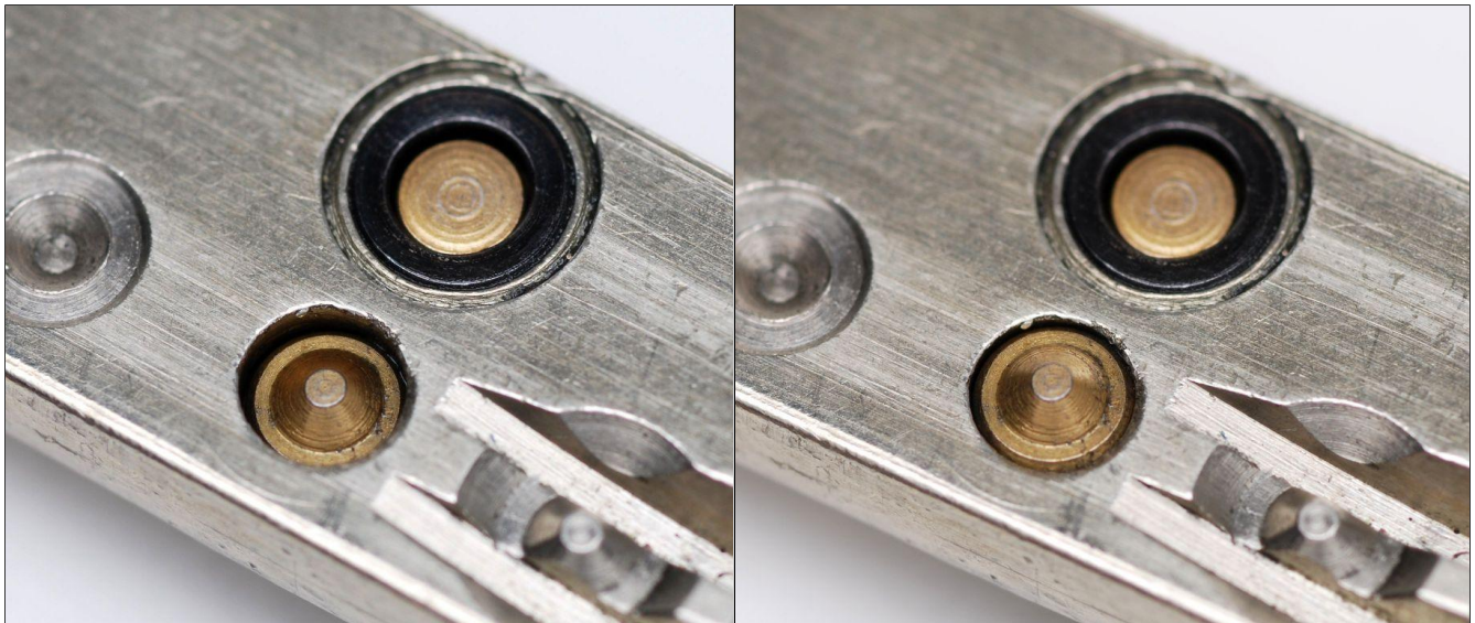
FIGURE 4.3: The key's Interactive moving element in the default (left) and raised (right) positions.
