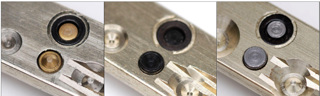
FIGURE 4.5: Left to right – Gold, Black, and Silver moving elements.
