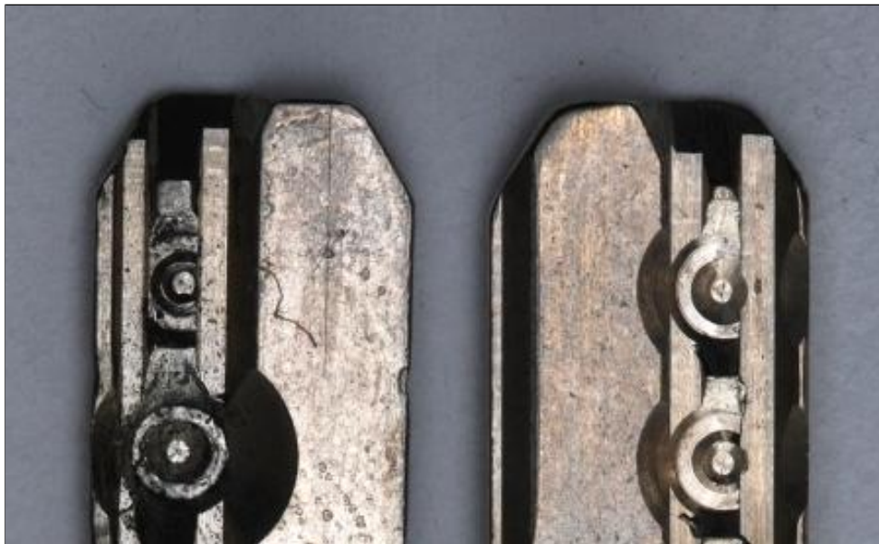
FIGURE 3.16: Left-Up/Right-Down and Right-Up/Left-Down bitting orientations.
