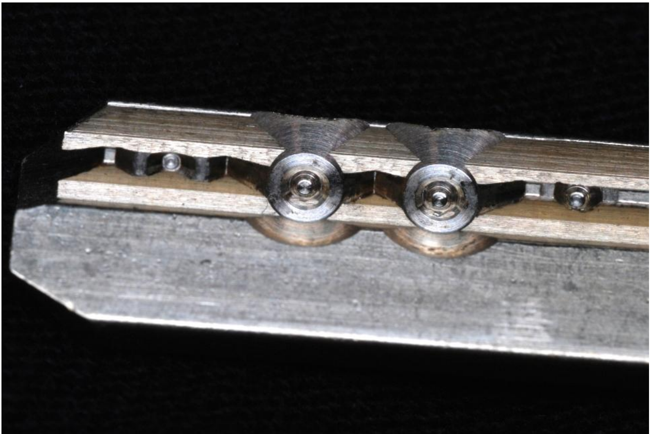
FIGURE 3.8: Bitting of a Mul-T-Lock Classic key, keyway 006C. Notice the concentric cuts used to position each telescoping pin.
