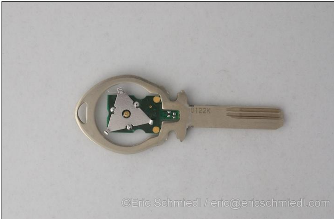
FIGURE 5.3: Control key with CLIQ electronics exposed. Note the lack of biting cuts.
