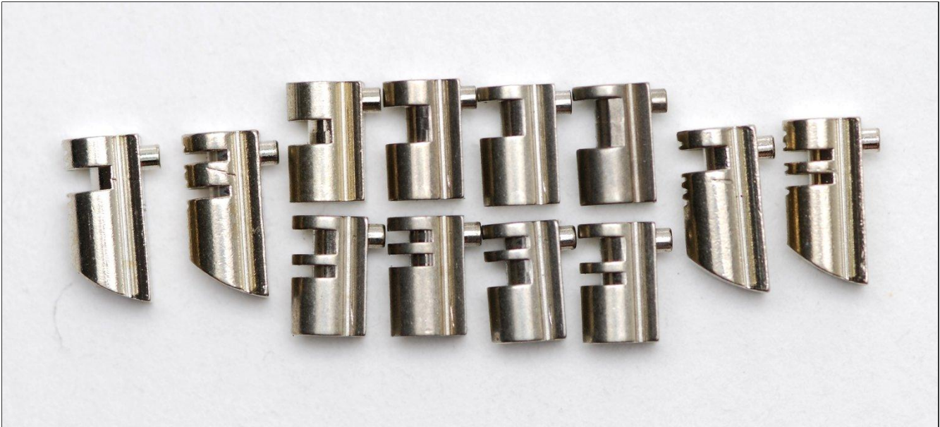
FIGURE 7.16: MT5+ slider master keying, both extended and multiple true gate varieties.
