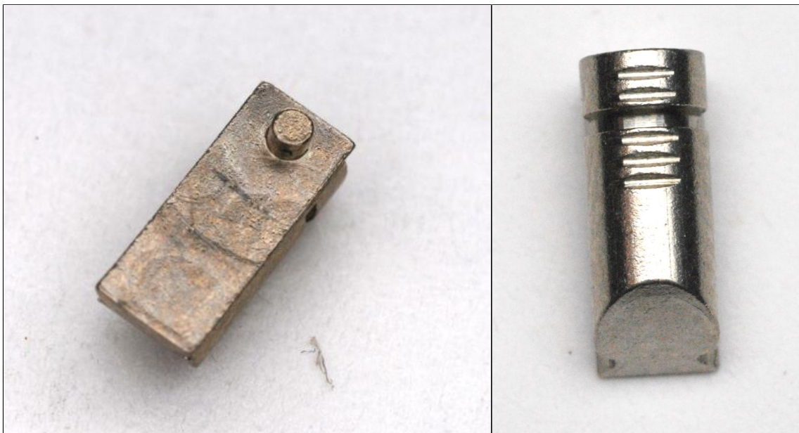
FIGURE 7.10: MT5+ slider. The top (left) interfaces with a track on the key, and the bottom (right) interfaces with the sidebar. Note the anti-picking false gates.
