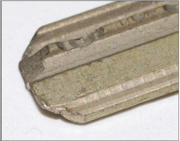
FIGURE 3.10 (Left): The 006C, by far the most common Classic key profile. FIGURE 3.11 (Right): A Classic key with light warding on the edge of the blade.
