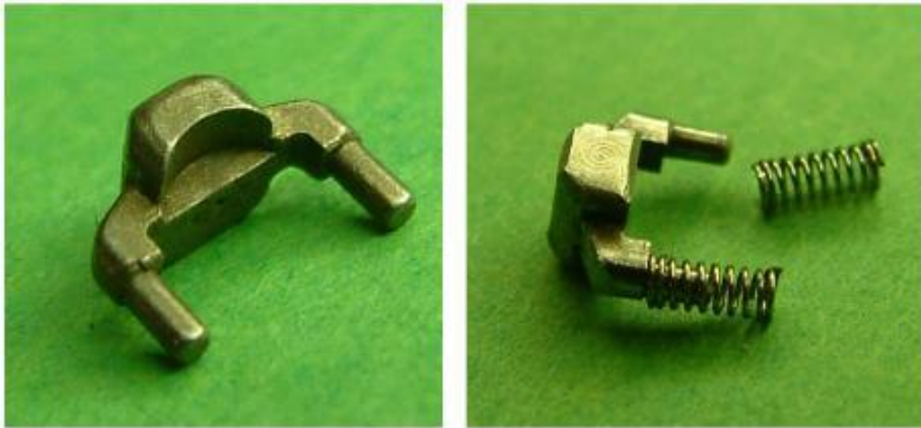
FIGURE 8.16: Design variations in the Mul-T-Lock CLIQ sidebar. (Image courtesy of Barry Wels )
