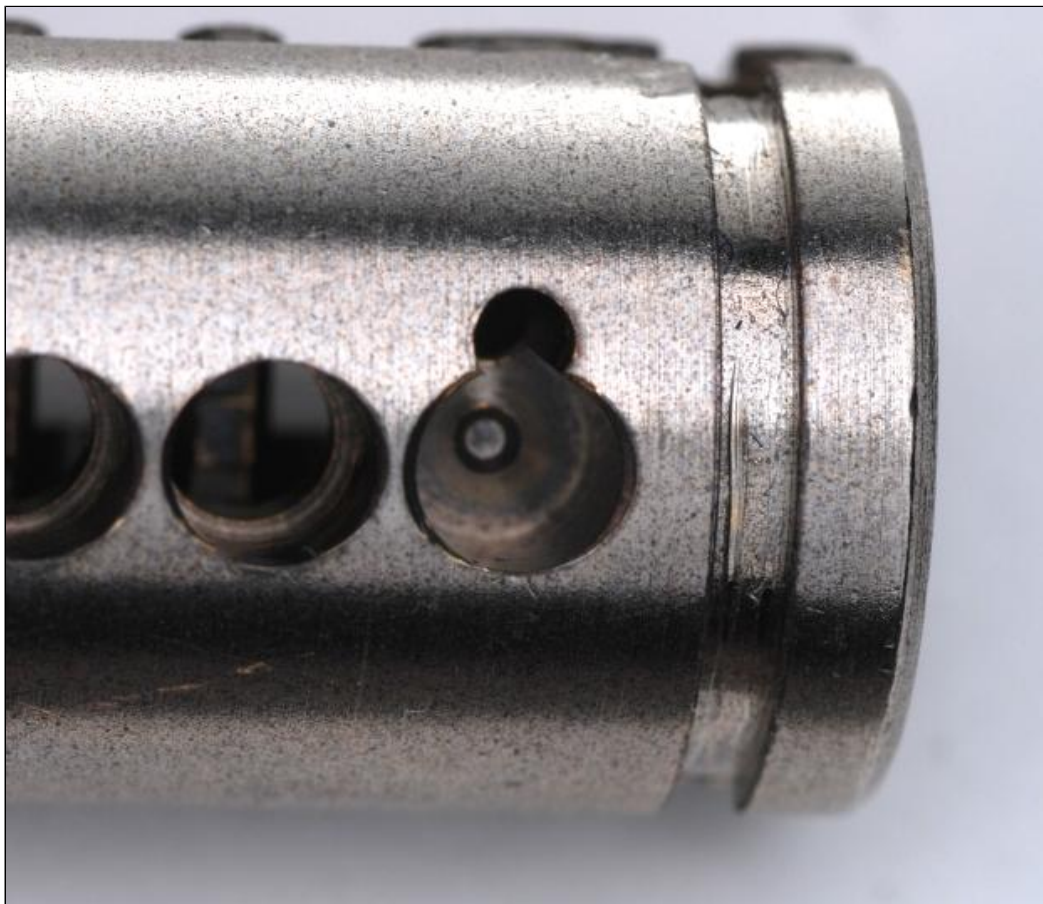
FIGURE 7.7: The Alpha chamber is not drilled like a traditional pin chamber. Instead, it only exposes the protrusion on the key pin.
