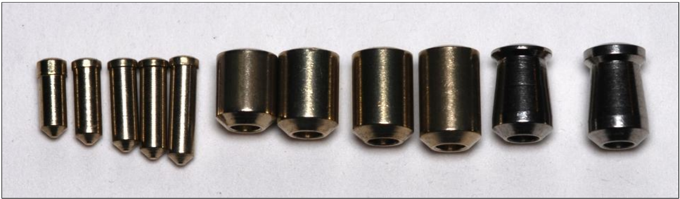
FIGURE 3.9: Classic key pins (all). Notice the difference in lips on the mushroom pins.
