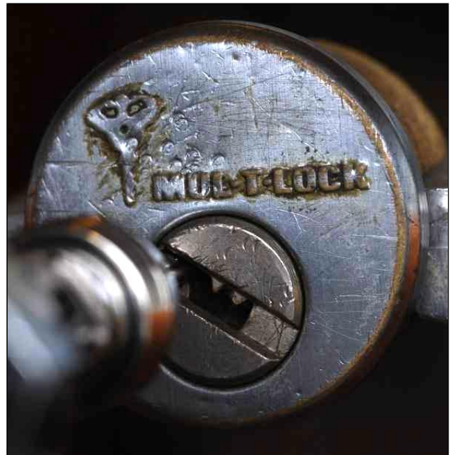
FIGURE 8.1: A Mul-T-Lock Classic fully picked.
