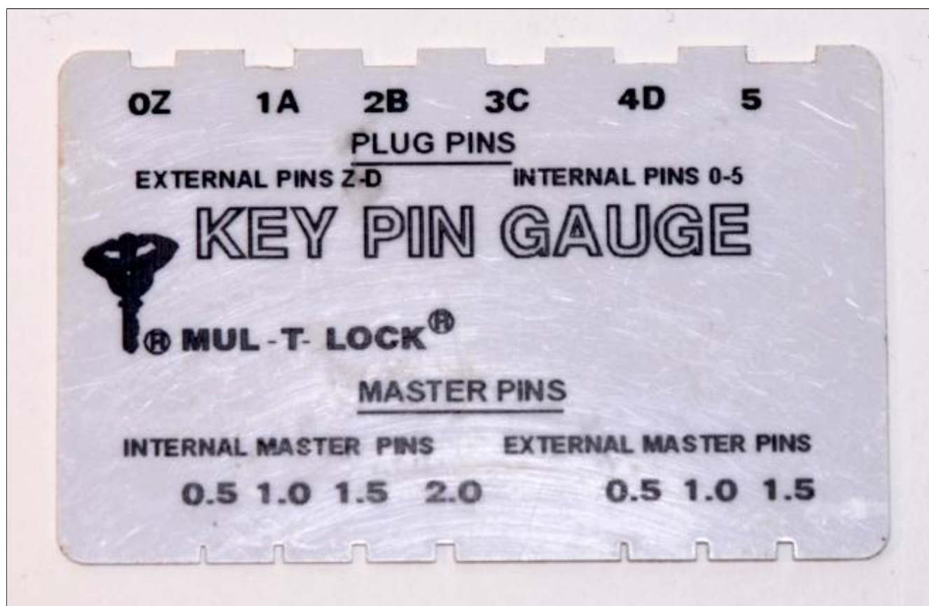
FIGURE 4.13: A Mul-T-Lock Classic/Interactive key gauge with 0/Z and master pins included.
