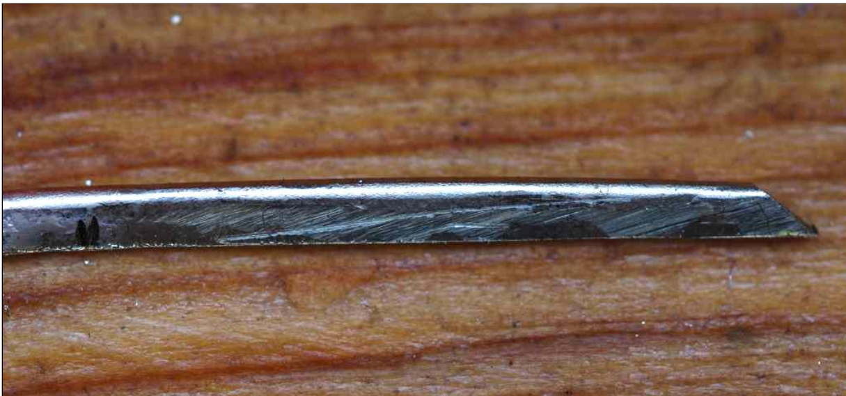
FIGURE 8.13: Mul-T-Lock impressioning tool, made out of brass.
