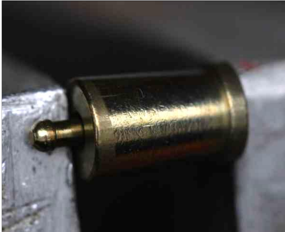
FIGURE 8.11: Modern style “nipped” driver pin, common in almost all new Mul-T-Lock cylinders.
