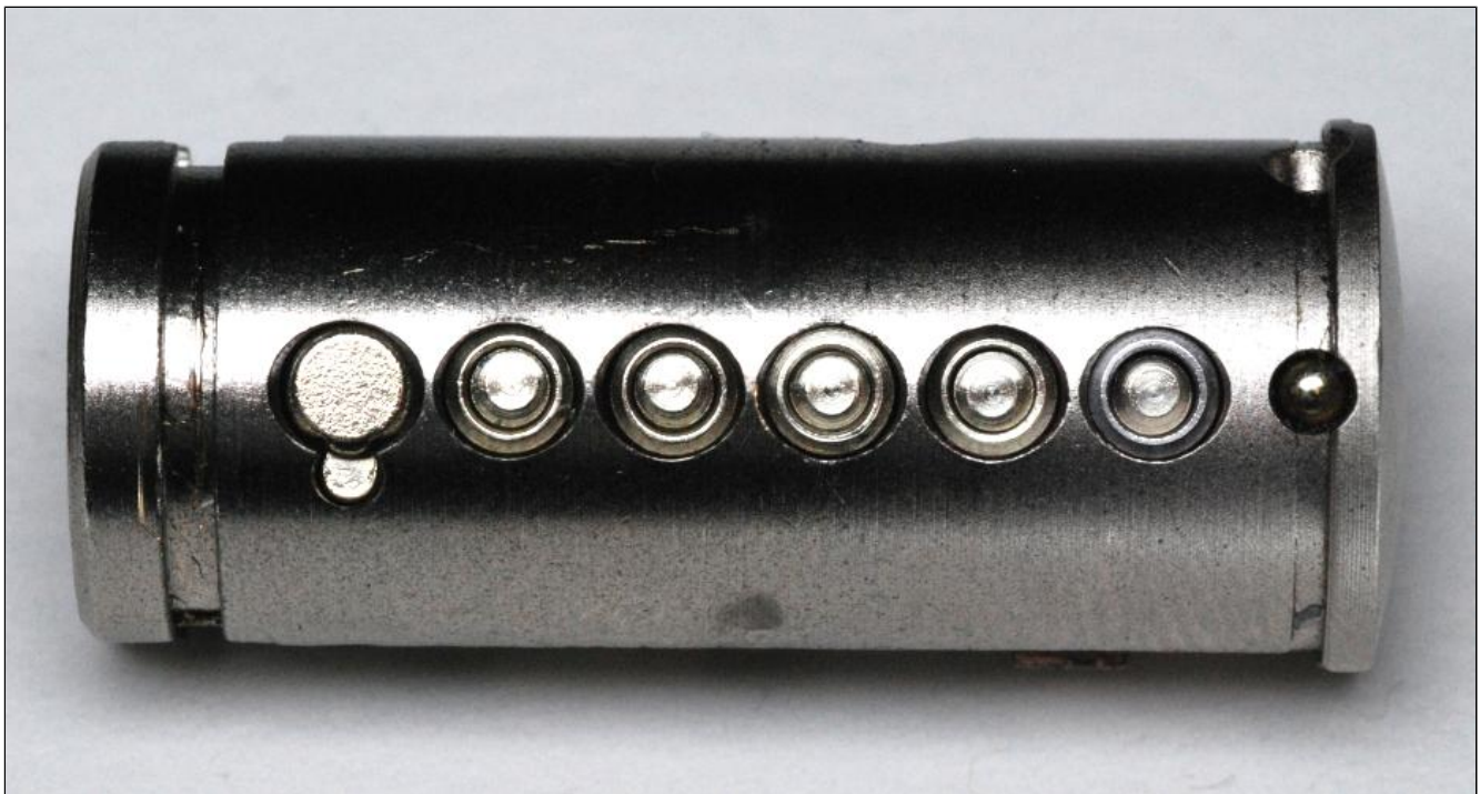
FIGURE 7.2: Top view of the MT5/MT5+ plug, showing five telescoping pin pairs, Alpha chamber (far left), and anti-forced entry ball bearing (right).
