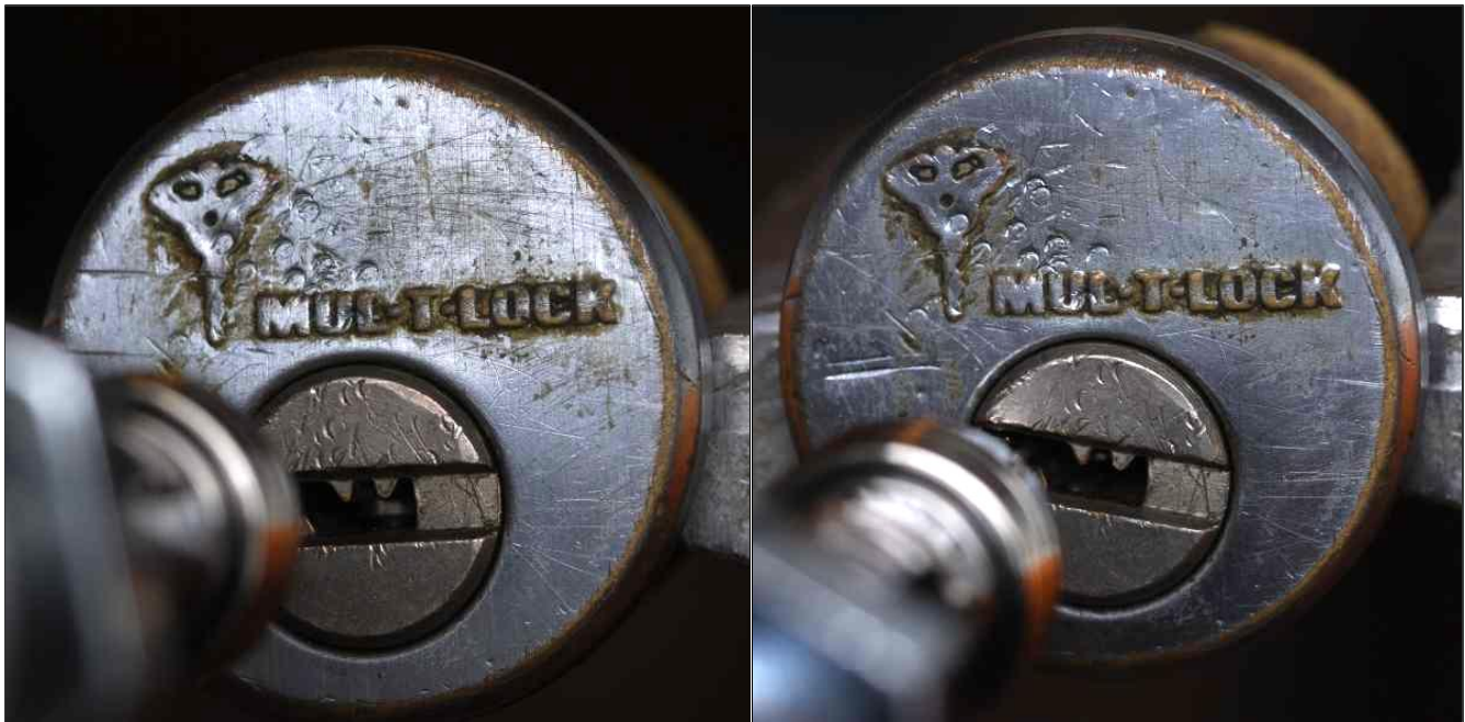
FIGURE 8.2: A Mul-T-Lock Classic in the normal (left) and partially picked (right) positions.
