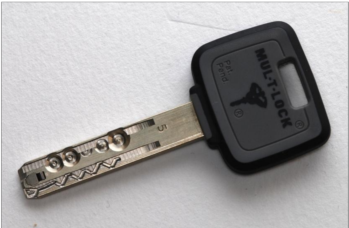
FIGURE 7.13: The MT5+ key with telescoping bitting, Alpha spring, and sidebar track.
