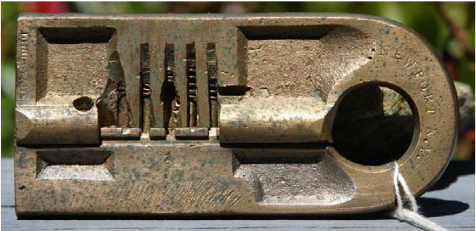
Linus Yale Sr's original Patent Model for the first pin tumbler lock. From the Patent Model Collection of Mr. & Mrs. O. Rundle Gilbert. Recently up for sale on eBay, though it received no bids.
