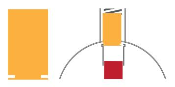
lock, the channel and the shelf will marry into one another, forming a tight connection. It will feel just as though the pin has set, and discovering it is incredibly difficult, much less correcting for it.
