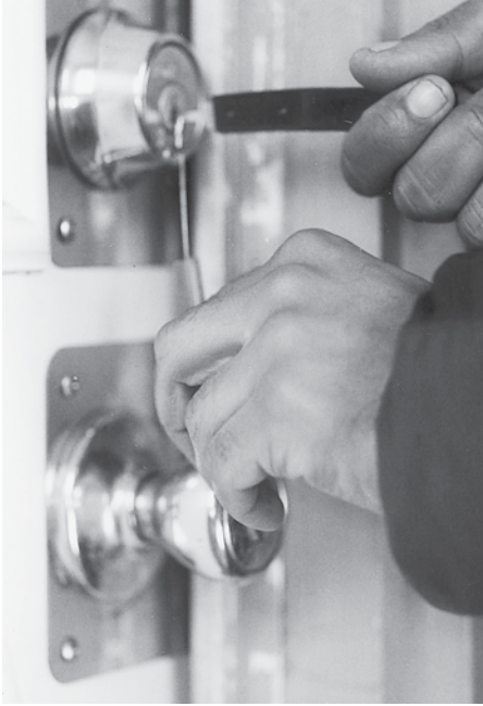
Figure 2.1 Most pin tumbler locks can be picked open with a pick and a torque wrench.
