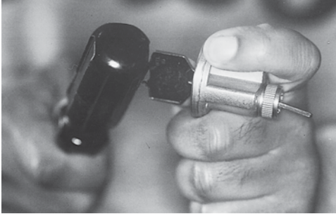
Figure 3.3 You can bump a key by using your thumb to apply turning pressure to the key's bow while tapping the bow, pushing it fully into the cylinder.
