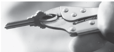
Figure 4.6 You can use pliers to hold the blank while impressioning.
