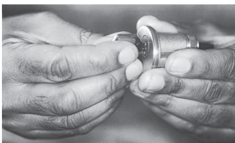
Figure 3.2 To bump a key, you first need to fully insert the bump key into a lock's plug.
