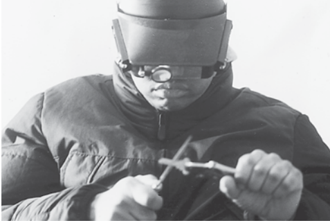
Figure 4.8 A head-wearing magnifying glass leaves your hands free while impressioning.
