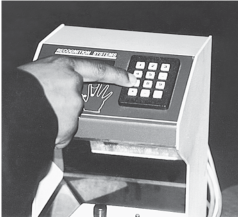
Figure 14.1 A hand reader is a popular biometric device.
