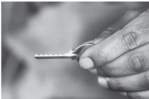
Figure 3.1 A bump key has all of its cuts at the deepest cut for the lock to be opened.
