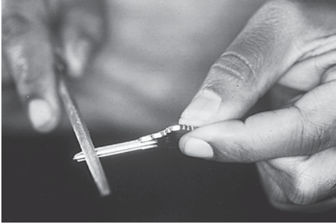
Figure 4.3 Use a file to prepare a key for impressioning.
