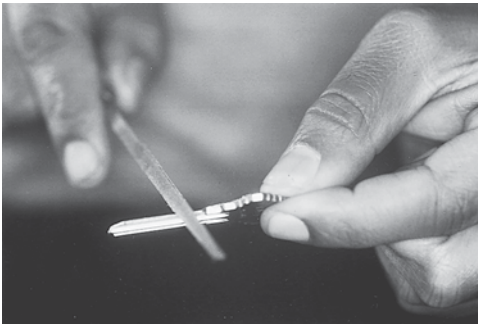
Figure 4.4 File along the length of the blade.
