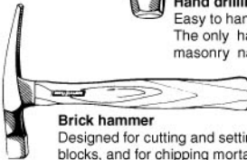
Figure 2.11 Striking tools are useful to locksmiths. (Vaughan & Bushnell Manufacturing Company)
