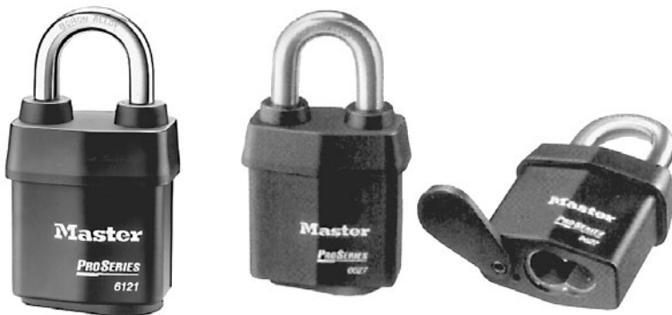
Figure 12.10 Pro Series "Weather Tough" padlocks are protected with "Xenoy" thermoplastic covers and feature boron alloy shackles and special drain channels that move water and debris through the lock body and away from the locking mechanism. ( Master Lock Company )
