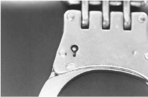
Figure 17.11 The keyway of most cuffs is for a small-barrel key.
