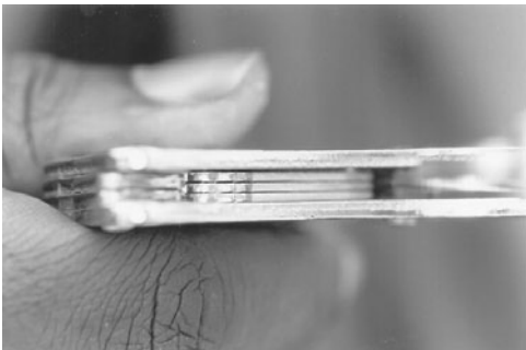
Figure 17.13 The pawl of a cuff is a spring-loaded bar with teeth angled opposite of the teeth of the ratchet, which lets the ratchet close but not back out without a key.
