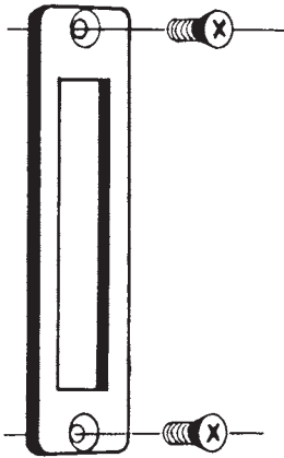
Figure 13.158 Simple trim strike plate for deadlocks in a metal stile door unit. ( Adams Rite Mfg. Co. )
