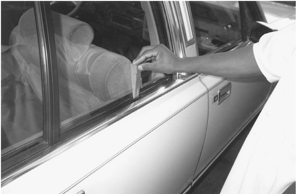
Figure 16.9 Before inserting a tool within a car door, insert a wedge to spread the door a little.
