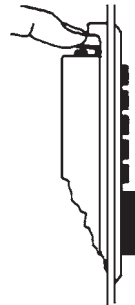
Figure 18.4 Changing Simplex combination, Step 3.
