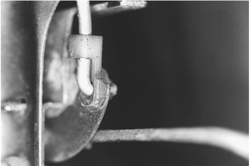
Figure 16.8 Linkage rods are attached to the bell crank. Many times, a vehicle can be unlocked by pushing or pulling on the bell crank.
