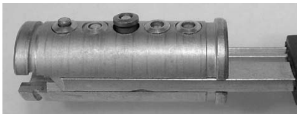
Figure 2.186: Mul-T-Lock plug with key partially inserted.
