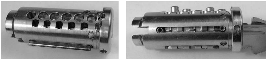
Figure 4.121: (Left) Top view of plug from Scorpion lock. (Right) Side view of plug with side-bar removed and key partially inserted.
