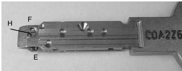
Figure 2.153: Key detail for Vachette Radial NT. Points E and F refer to ends of movable element. H is the hole.
