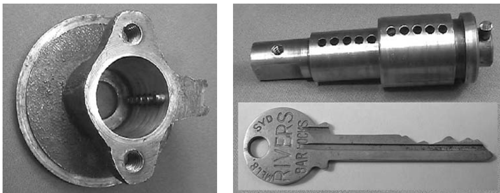
Figure 2.47: (Left) Rivers lock driver pins are captive in upper chambers. (Right) Core comprises inner and outer plugs, shown alongside key.
