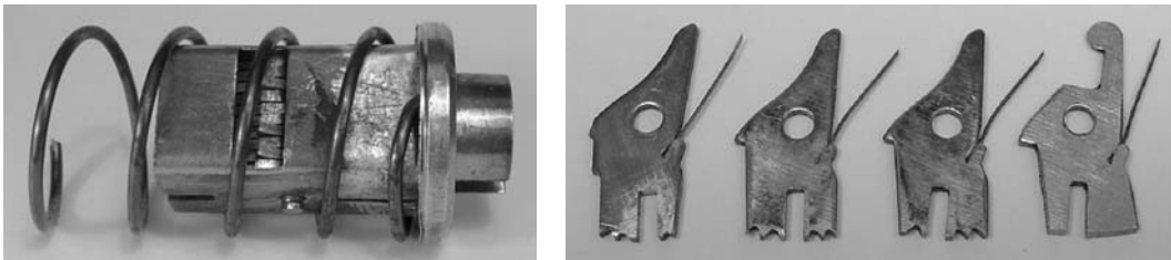
Figure 5.94: (Left) Plug and main spring from Muel cylinder. (Right) Selection of levers with scoop-type lever on right.
