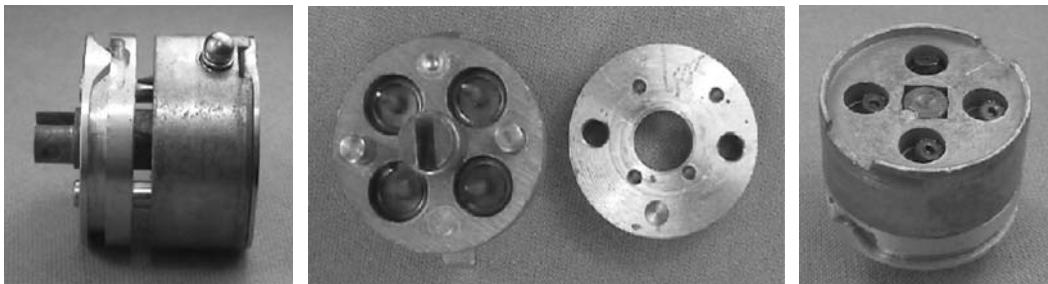
Figure 6.25: MagLok core consists of front and rear sections; front section contains four tilting magnetic tumblers.
