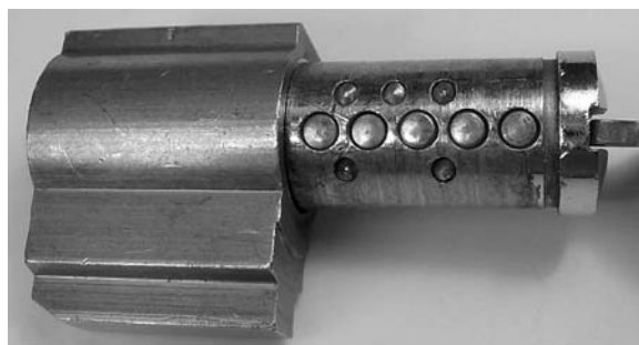
Figure 2.100: Vachette 2000 plug with key inserted to align pins.
