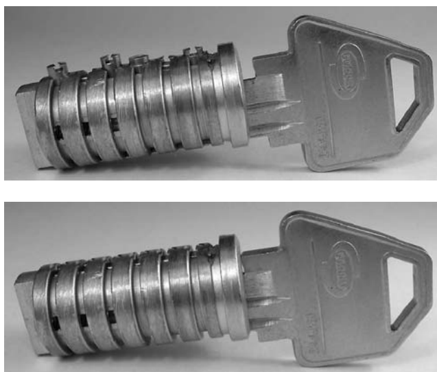
Figure 2.195: (Top) Emhart plug with key partially inserted. (Bottom) Key fully inserted to align pins with grooves in plug.
