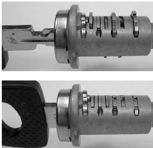
Figure 7.30: Operation of Mercedes four-track lock.
