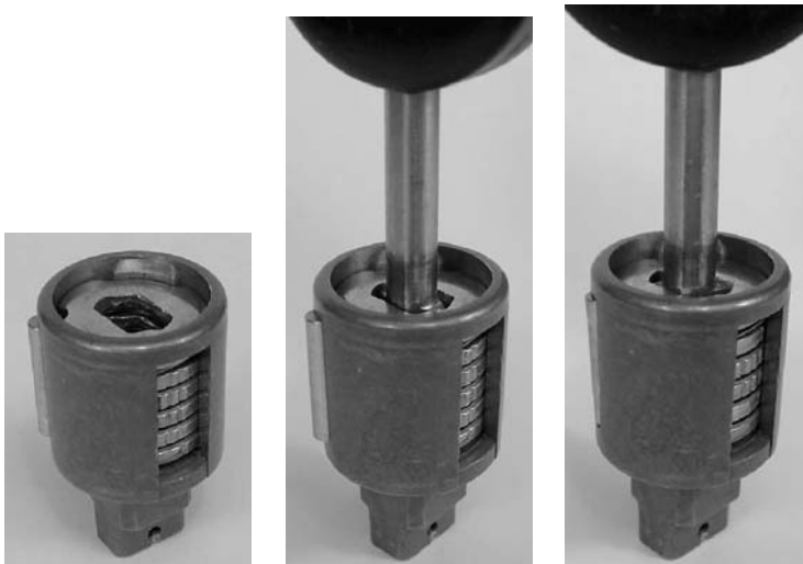
Figure 7.12: (Left) Ford Tibbe core. (Middle & right) Key aligns discs to retract side-bar.
