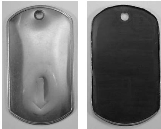
Figure 6.37: (Left) Schlage CorKey card key. (Right) Cover removed to expose flexible magnetic strip.
