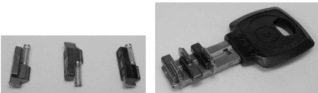
Figure 6.23: (Left) Miwa magnetic tumblers. (Right) Key with three magnetic tumblers in position.
