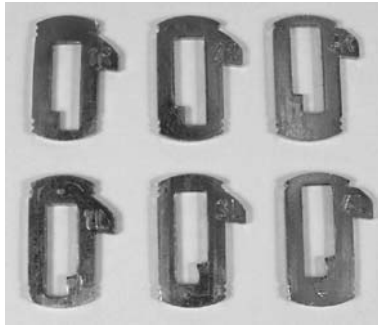
Figure 7.41: Volvo four-track wafers: right-handed on top row, left-handed on bottom row.
