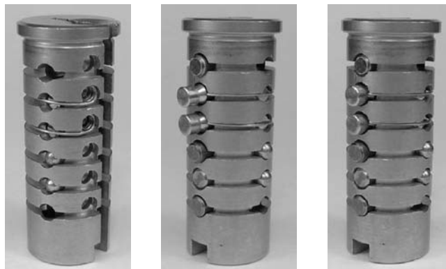
Figure 2.103: MLA Binary Plus plug: location of side-trap springs (left); antipick pins overraised and caught by side-trap springs (middle & right).
