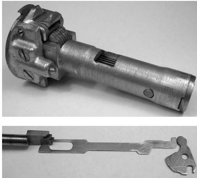
Figure 5.90: (Top) NS Fichet core and barrel assembly with crank engaging rocker gates. (Bottom) Operation of a single push-rod and rocker.
