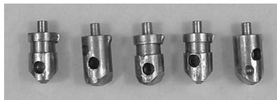
Figure 4.59: Medeco cam lock pins with either false-depth hole or antipick groove.
