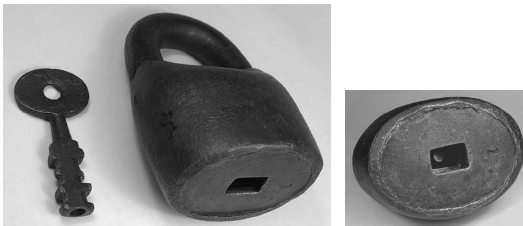
Figure 4.1: Scandinavian 3-disc padlock taking a pipe key.
