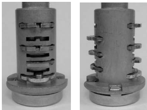
Figure 7.29: Two views of Mercedes four-track plug.
