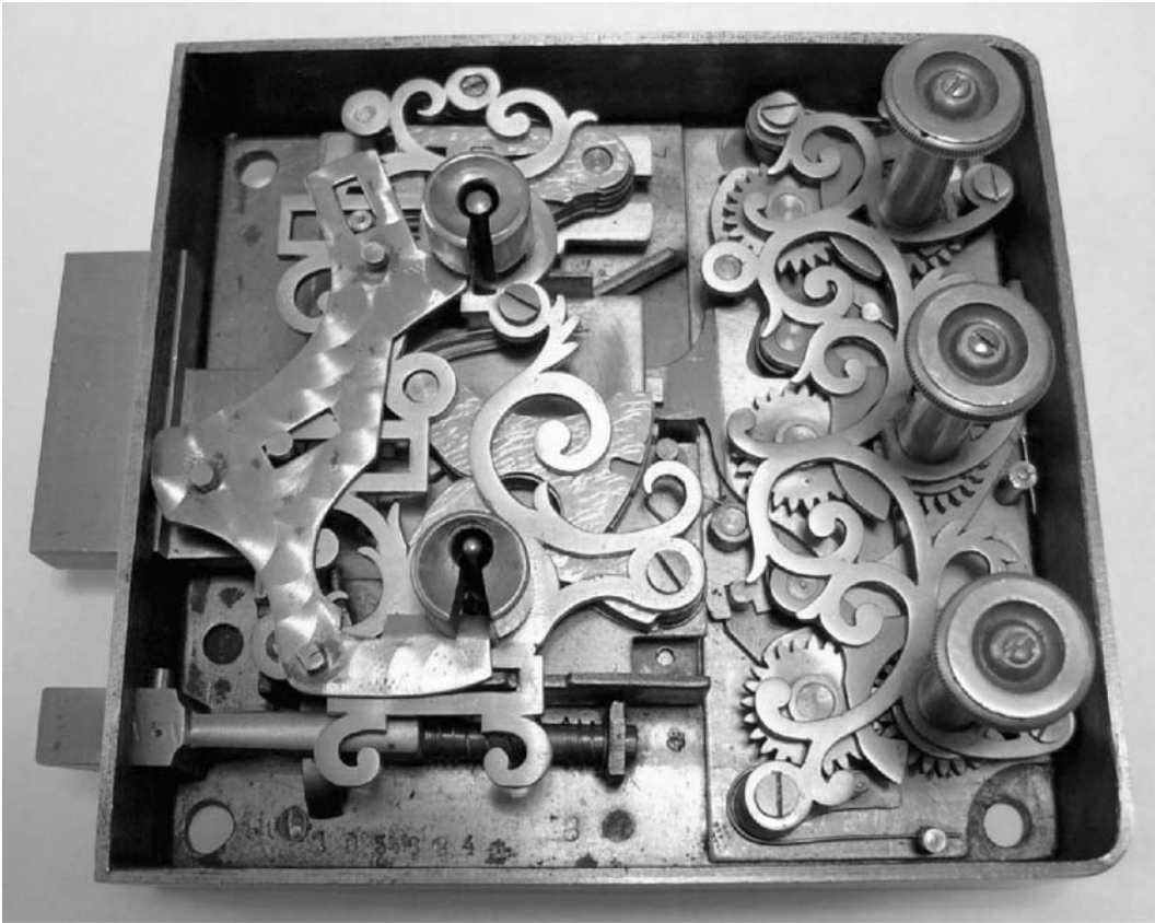
Figure 5.47: Triple-control Fichet safe deposit lock with 3-knob “click” mechanism. First, the three knobs must be set at the correct positions. The guard key is then inserted in the upper keyhole and turned to allow access for the renter’s key (top), which is inserted in the lower keyhole to operate the compound 5-lever lock. The fretting is ornamental—the original lock would have had a plain steel front plate.
