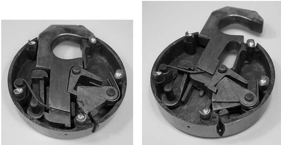
Figure 5.86: Miller padlock with cover removed in locked and unlocked positions.
