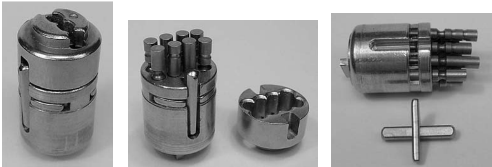
Figure 4.82: (Left) Tubar core. (Middle) Core with cap removed. (Right) Tubar core with one side-bar.
