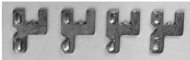
Figure 7.17: Selection of wafers from a GM side-bar lock.
