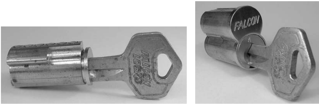
Figure 2.43: (Left) Control key aligns pins at control shear line. (Right) Retracting the locking lug for removal of core.
