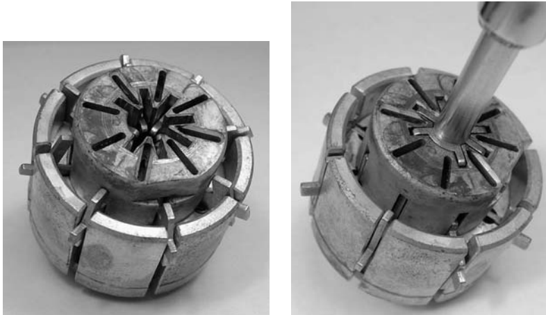
Figure 5.107: (Left) Fichet-Bauché M2B core with levers in rest positions. (Right) Core with key inserted.
