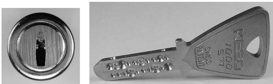
Figure 2.124: KESO 1000 S cylinder and key with both left- and right-handed bore patterns.
