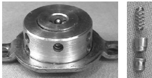
Figure 2.155: YBU lock with cover removed (left) and close-up of pin-tumbler (right).
