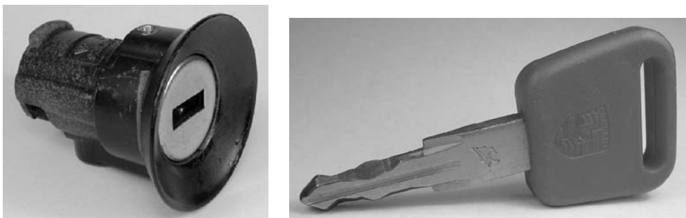
Figure 7.34: Porsche 928 four-track lock barrel and key.
