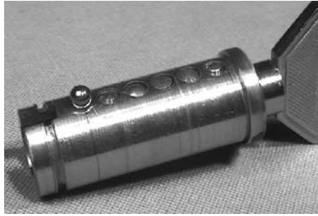
Figure 2.39: Maxis plug with pins at shear line.
