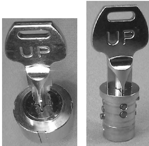
Figure 2.114: A cruciform lock with 10 pins.
