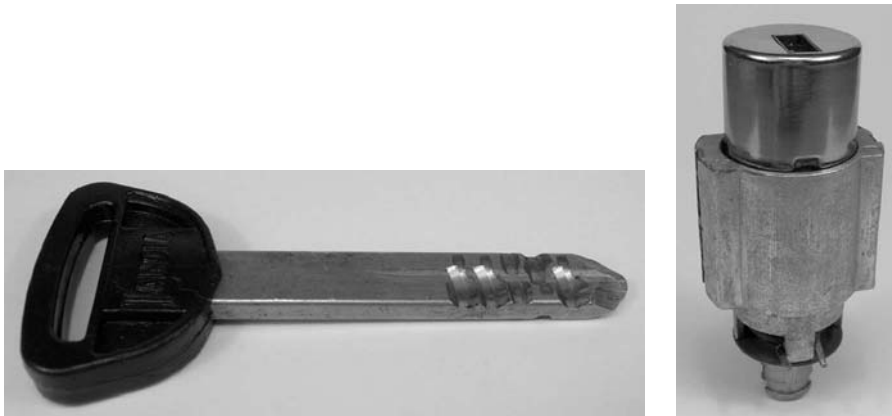
Figure 7.37: Lancia/Alpha-Romeo key and 10-pin lock barrel.
