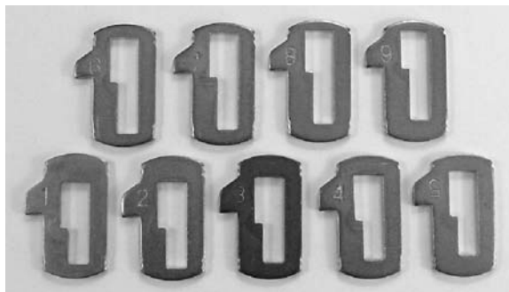
Figure 7.9: Set of wafers from Holden Commodore lock.
