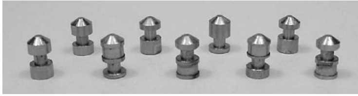
Figure 7.44: Driverless pins from Simplex lock.
