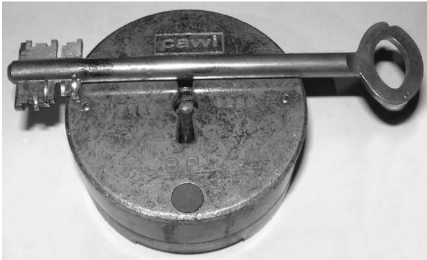
Figure 5.124: CAWI safe lock and double-bitted key. (Courtesy O. Diederichsen).
