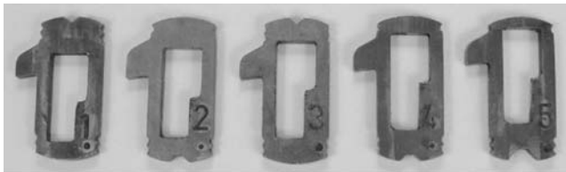
Figure 7.22: Wafers from Mercedes two-track lock.
