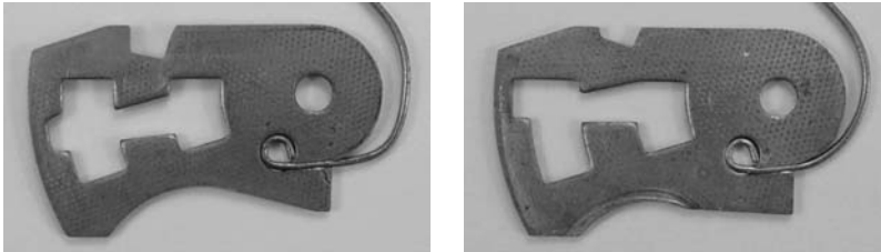
Figure 5.69: Detector lock levers have constant-width section at top of gate.
