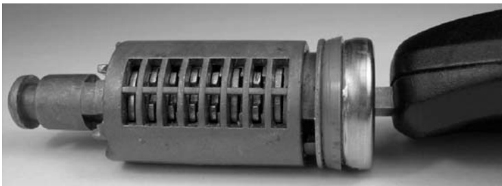
Figure 7.26: BMW plug and cage with correct key fully inserted.
