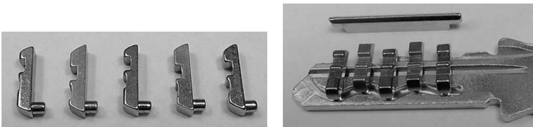
Figure 4.122: (Left) Finger pins from Scorpion lock. (Right) Finger pins on key blade, side-bar at top.
