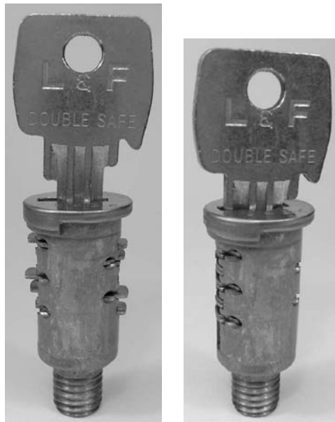
Figure 3.8: Side view of insertion of double-sided key as it brings wafers into alignment.
