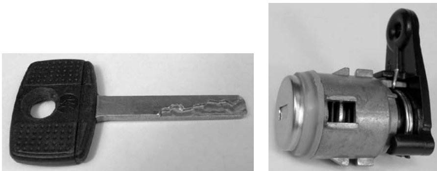
Figure 7.8: Holden Commodore 7-wafer barrel and two-track key.
