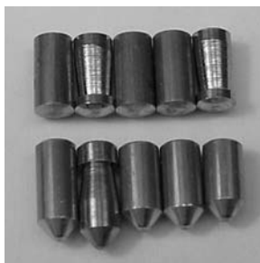
Figure 2.85: Pin pairs from the Tover 2F30, including spooled top and bottom pins.
