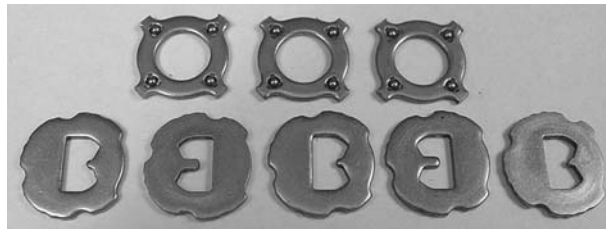
Figure 4.36: Sample of DOM Diamant left- and right-handed discs with separators.
