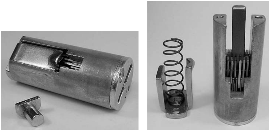
Figure 4.44: (Left) Mottura core with side-bar in foreground. (Right) Core with rear cover removed to show sliders and tail-piece.
