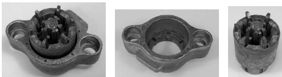
Figure 3.53: Supra 6-slider core and rear cap.
