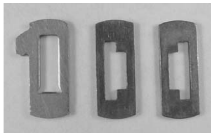
Figure 3.18: Conventional wafer-tumbler and two Bricard wafer-tumblers.
