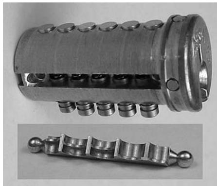
Figure 4.103: Assa Twin plug with six top pins and five side pins. Inset shows side-bar.
