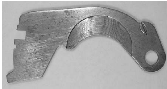
Figure 5.29: Lever from a Chubb 3G110 Butter's system lock.
