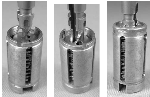
Figure 4.37: (Left and middle) DOM Diamant shell with key partially inserted. (Right) Full insertion of key aligns gates in discs.
