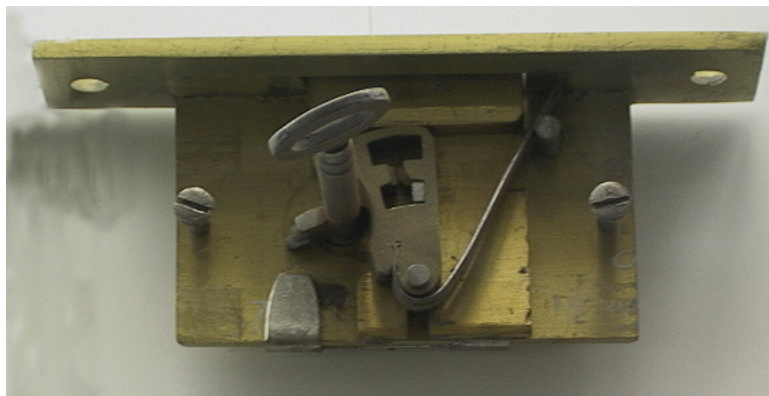
Figure LSS+116 The lever lock developed by Hobbs and Hart.
