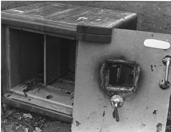
Figure LSS+3521 These photographs show attacks by torch. In the middle picture, an inept attempt to open the safe by cutting through the side. The burglar knew how to use a torch, but had no idea of where to cut. In the photograph (right), a torch attack on the lock box.
