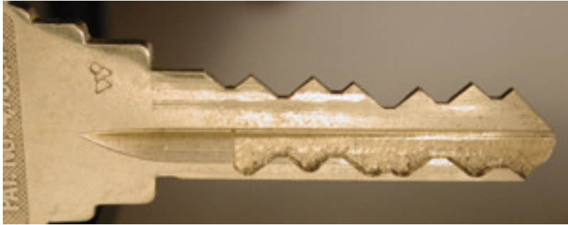
Figure LSS+1709 A schlage Primus key, showing sidebar millings with a code of 23624. There are three rotations and four actual depth increments that are available with Primus.
