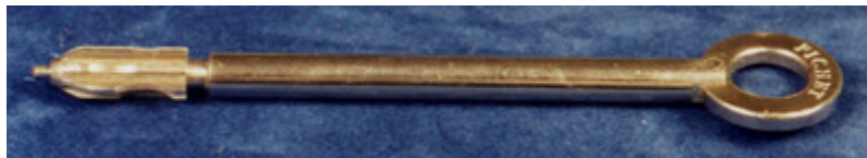
Figure LSS+3108 Note the unusual design of the key for the Fichet Monopole lock. Courtesy of John Falle.
