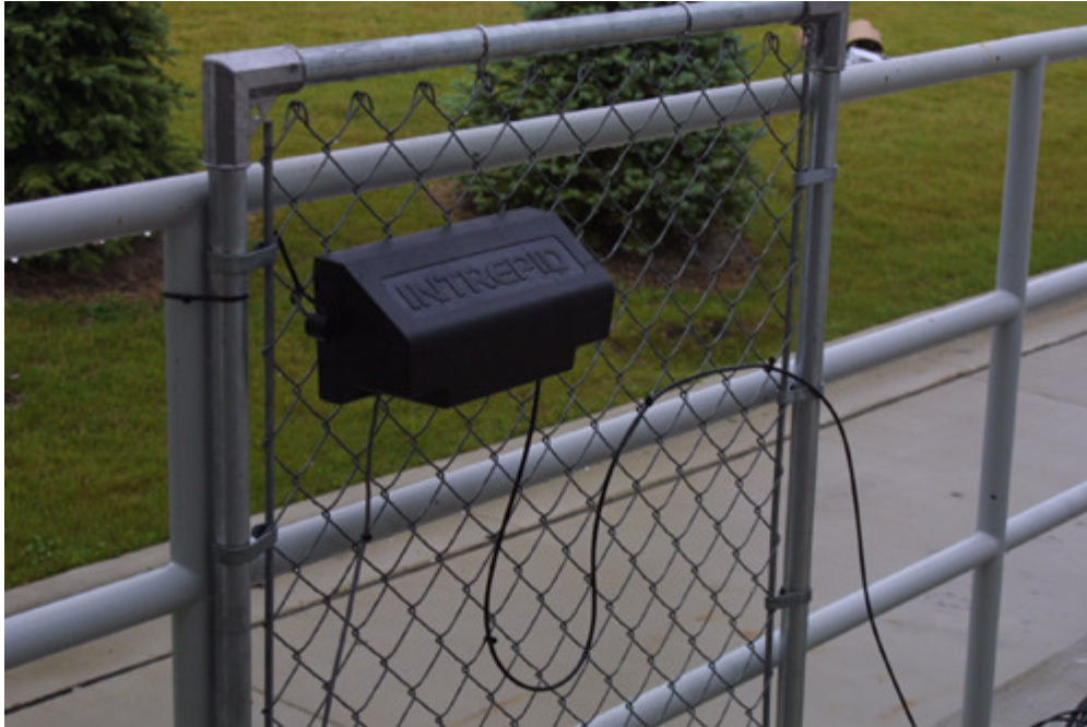
Figure LSS+4047 There are several different sensor technologies that are utilized to protect fences, including strain, vibration, and noise detection.
