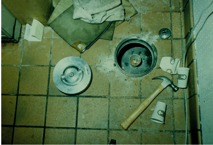
Figure LSS+3551 (ISP 8-2963 left; 10-2963 right). Example of floor safe that has been angle drilled to view wheel pack. Courtesy of Illinois State Police, Bill Sherlock.
