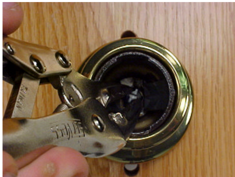
Figure LSS+3901 The Kwikset cylinder key-in-knob assembly may be removed quickly and easily with a special tool to release the two retaining clips. A vicegrips or pliers may then be inserted to manipulate the bolt. Courtesy of Medeco.
