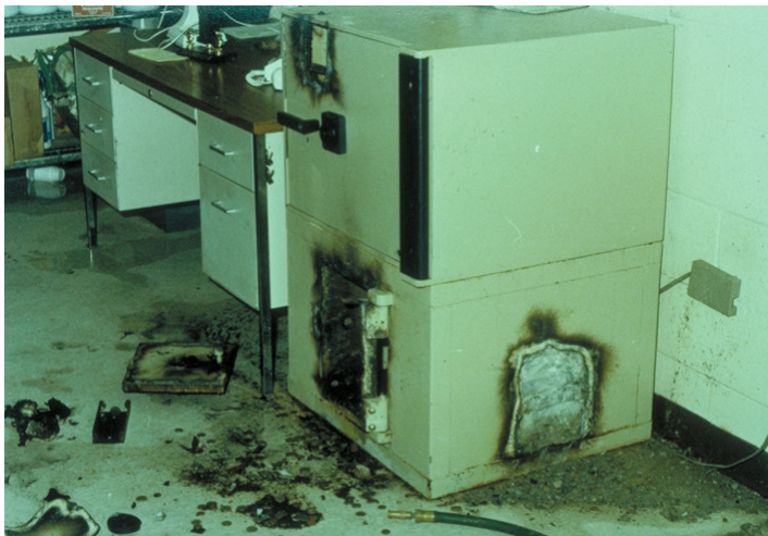
Figure LSS+3527, (left) a torch attack where burglars cut a portion from the door for access, and (right) where part of the skin was removed to access the bolt mechanism.
