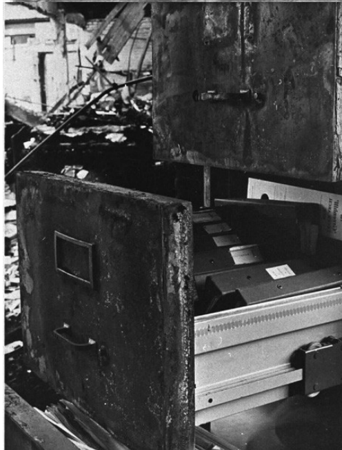
Figure LSS+3308 Examples of fire protected file cabinets.
