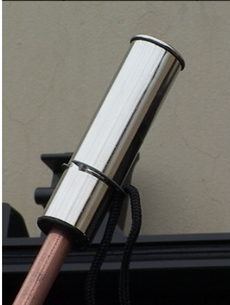
Figure LSS+3229 A close-up of the control valve with a rod inserted. The rod is inserted into a self-contained ignition system which requires no battery. It is pushed into the special capsule and will ignite.
