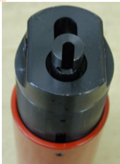
Figure LSS+3225 The MSC Lock Force tool can be used to remove profile cylinders from their housing.
