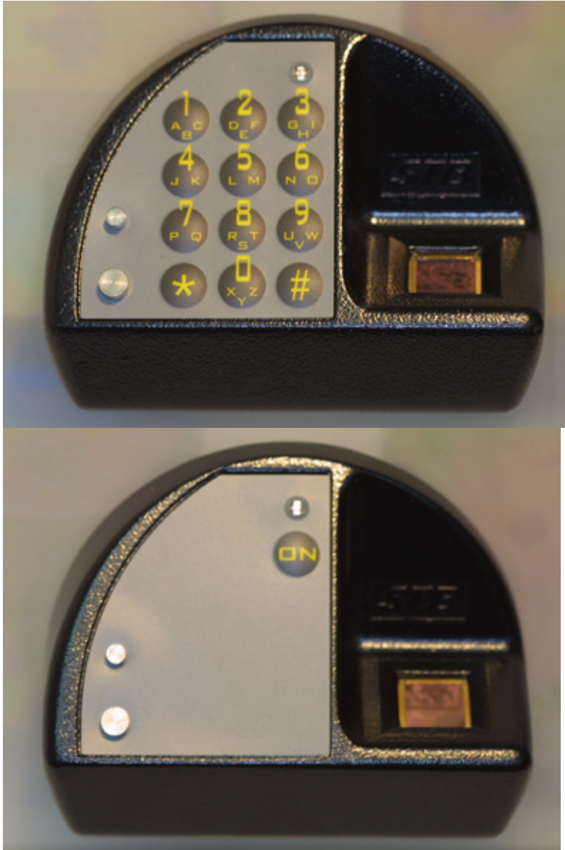
Figure LSS+3902 Fingerprint recognition is utilized in the STB electronic combination lock for safes.
