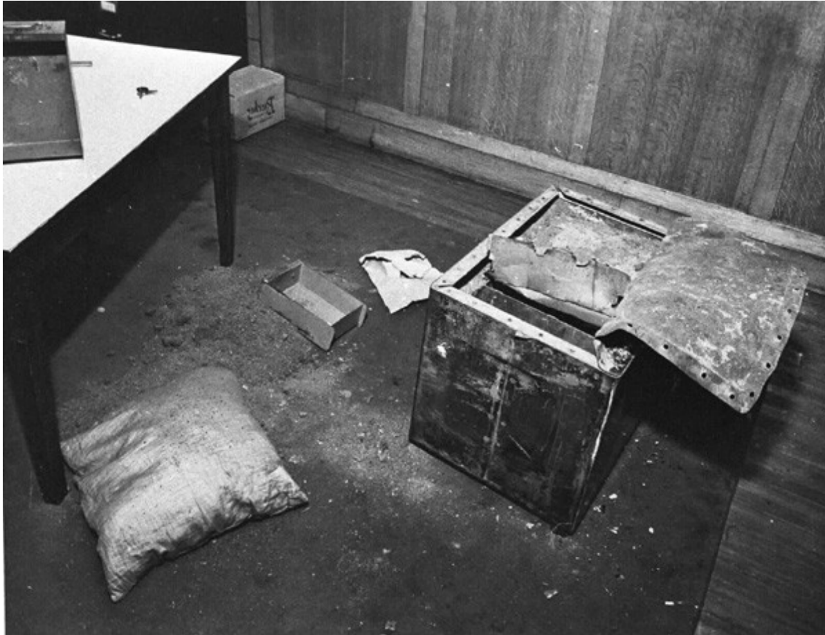
Figure LSS+3512, examples of peeling of the outer skin on the top of the container (left), and the rivets popped through peeling (right).
