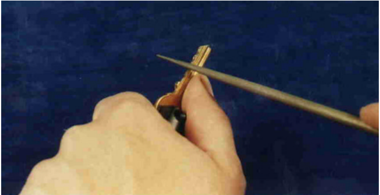
Figure LSS+3002 Use of a pippin file for impressioning.
