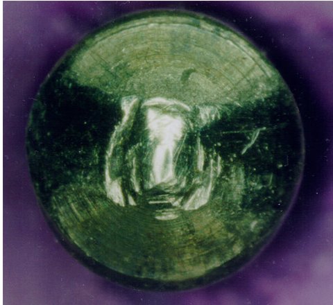
Figure LSS+2614 Marks produced from pick gun.
