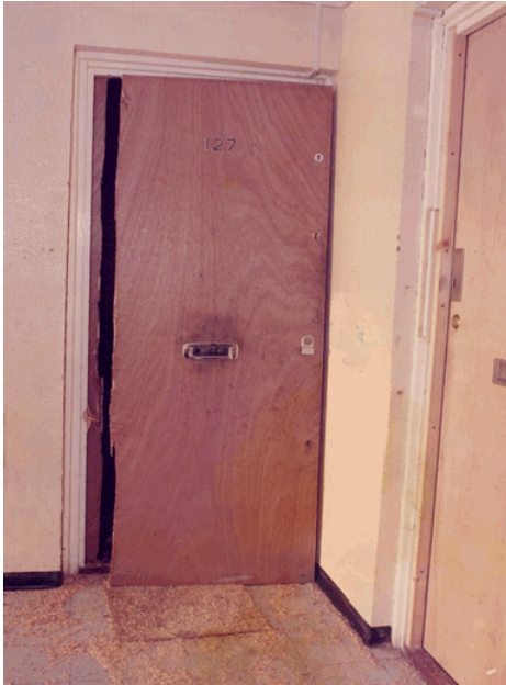
Figure LSS+3215 Right hand inward opening solid timber door with four individual locks. Attack made with chain saw on hinge side.
