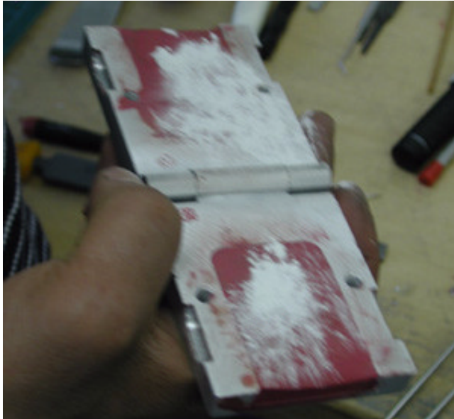
LSS+806 Talc or other lubricant is applied to the clay to facilitate removal of the source key after an impression is taken.
