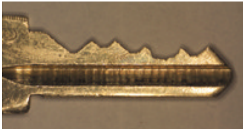
Figure LSS+601, a back cut key. Note the angle of cut of the fourth tumbler position from the shoulder
