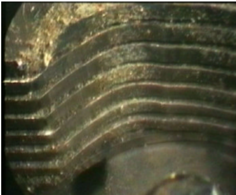
Figure LSS+2939 Markings on levers can be utilized as an aid to picking.
