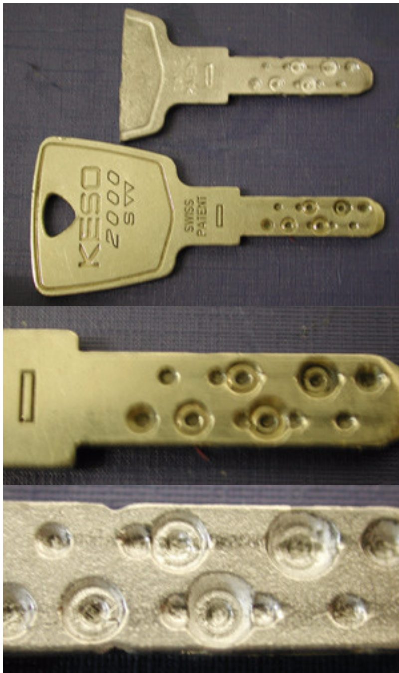
LSS+820 The source and target key in two different castings are shown. Exact detail is replicated.
