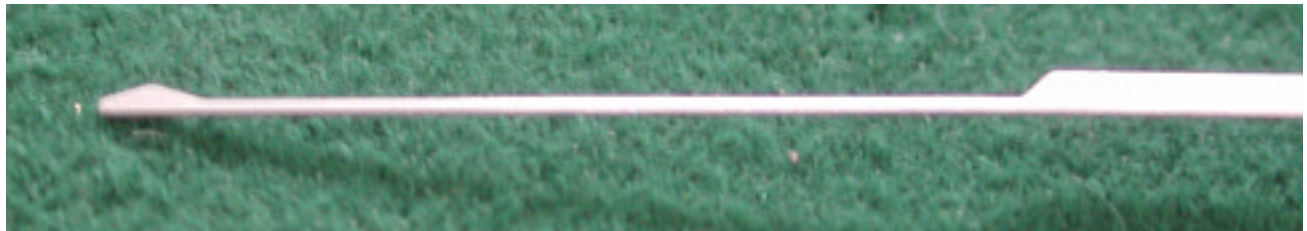
Figure LSS+3138 The calibrated pick-probe holder forms part of the decoding tool.
