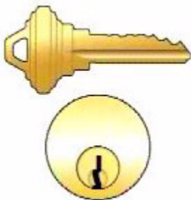
Figure LSS+1104 The change key is the lowest level of keying. One key fits one lock. Courtesy of HPC Interactive Learning Series.
