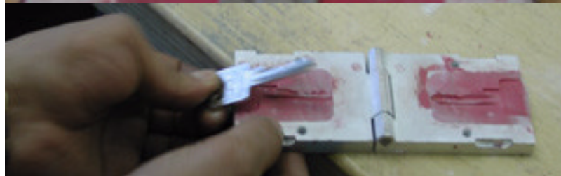
LSS+812 The key is carefully removed from the mold, taking care not to distort the impression.
