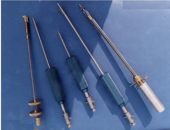
Figure LSS+2924 A variety of tools are produced by John Falle for opening high-security lever locks. Courtesy of John Falle.
