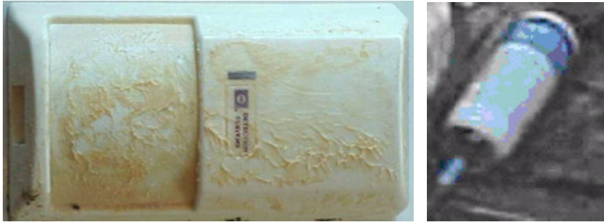
Dual-technology sensor, covered with silicone
