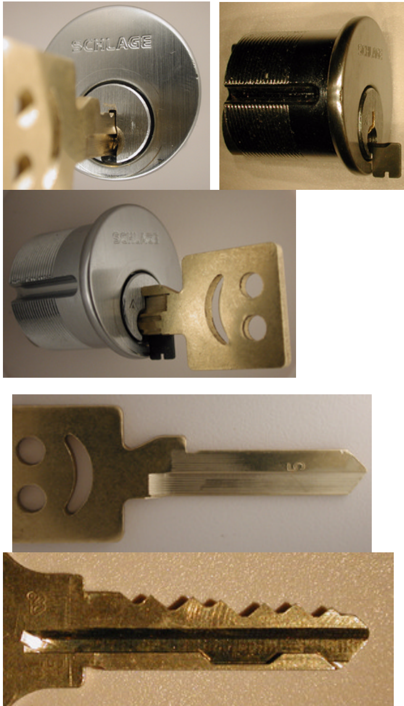
Figure LSS+3148 The Schlage Everest cylinder utilizes a patented check-pin system and undercut keyway. A blank has been produced with the Easy entrie profile milling machine that effectively eliminates the requirement that a corresponding channel on the key must pass the undercut in the keyway. Compare
