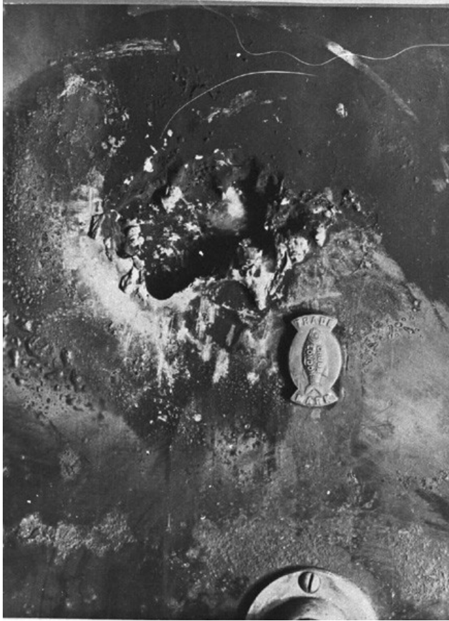
Figure LSS+3524 (left) photograph showing lines scored by an oxyacetylene torch in the outer shell of a Chubb safe. The burglars tried to cut the lock out of the middle of the door. In the photograph (right), a close-up of an oxyacetylene attack of Chubb safe which was not successful.
