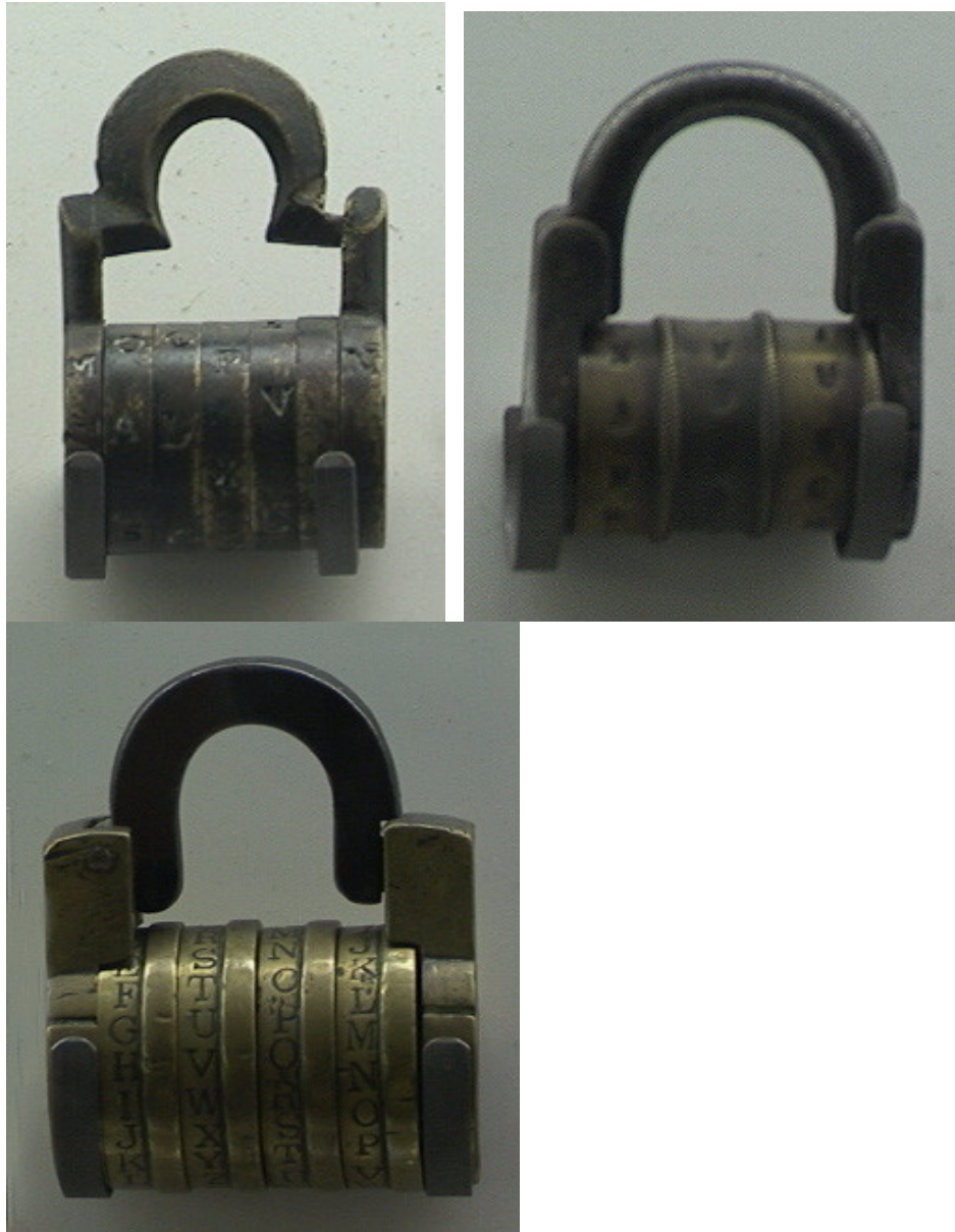
Figure LSS+3409 Examples of early combination padlocks. Shown is an Italian nineteenth century puzzle lock (left), another example of a permutation lock, origin unknown (middle), and an eighteenth century four wheel lock.
