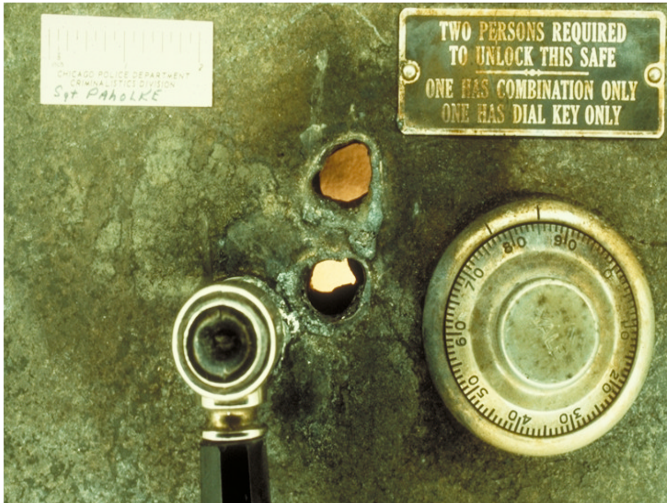
Figure LSS+3530 (ISP-76-3563) An example of a safe attacked with a thermic lance.
