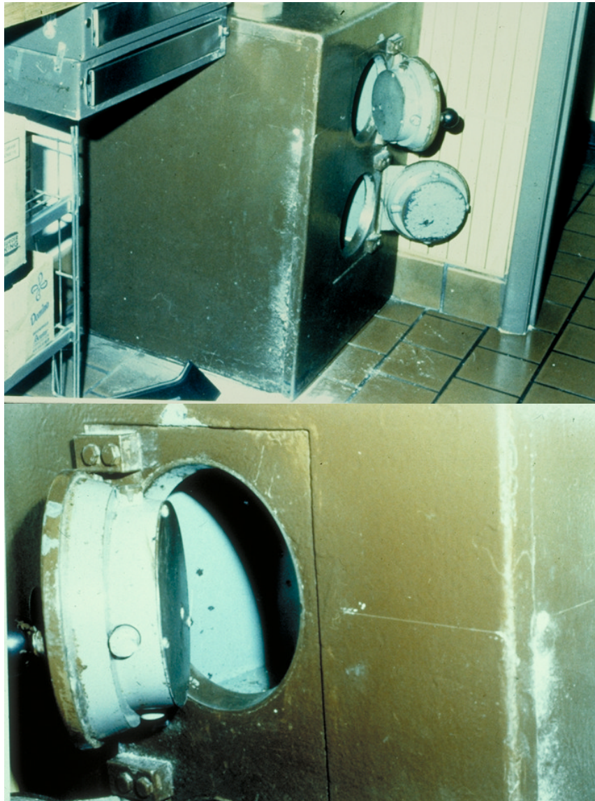
Figure LSS+3540 (top left, ISP 2-2963; right 3-2963; bottom left 5-2963; right 6-2963) In 2,3 above, burglars drilled into the side of the safe to punch and drive the bolt out of the way. The same procedure was utilized in 5,6. Courtesy of Illinois State Police, Bill Sherlock.
