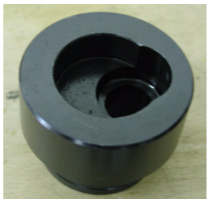
Figure LSS+3225 The MSC Lock Force tool can be used to remove profile cylinders from their housing.
