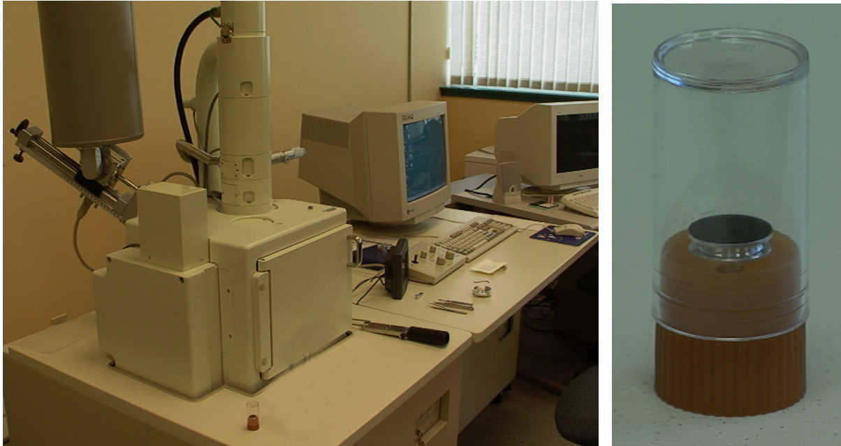
Figure LSS+2616 A Jeol 5900 SEM system and a specimen container for placing a small amount of material in the chamber to be analyzed. This system is in operation at the University of Rhode Island Forensic Laboratory.
