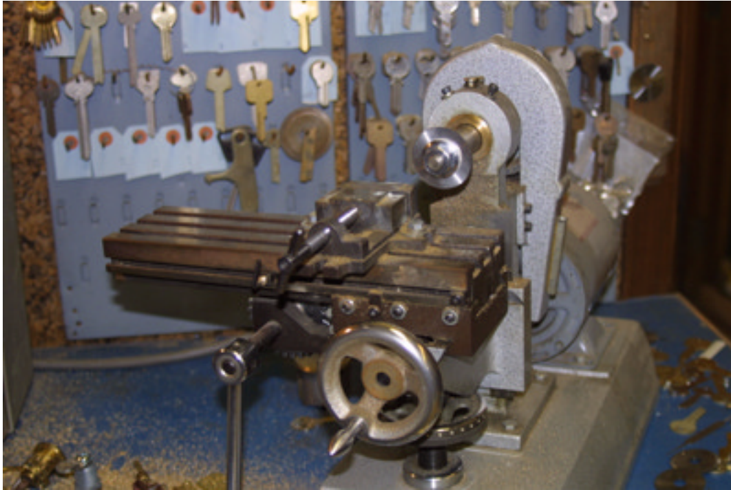
Figure LSS+836 The Keyway King is a milling machine that operates in three planes.
