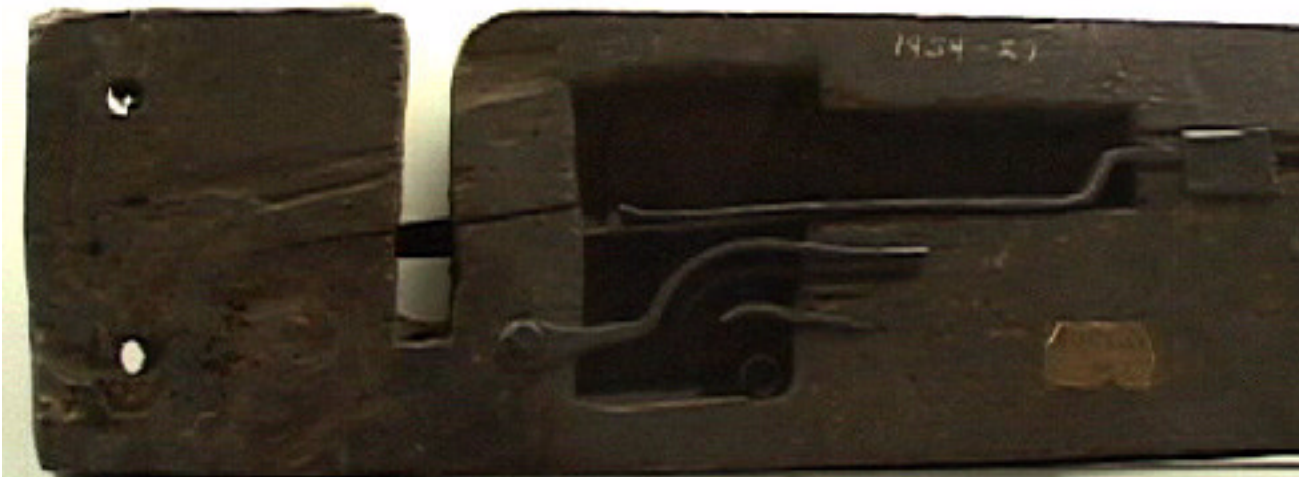
Figure LSS+107. An early warded lock, showing the obstructions to rotation of the key.
