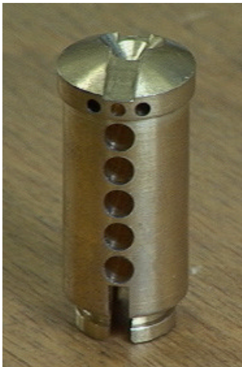
Figure LSS+1608 A plug is formed; drill resistant pins are inserted, then the individual chamber holes are drilled.
