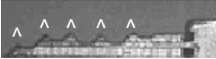
Figure LSS+603, bitting of key showing steeples.
