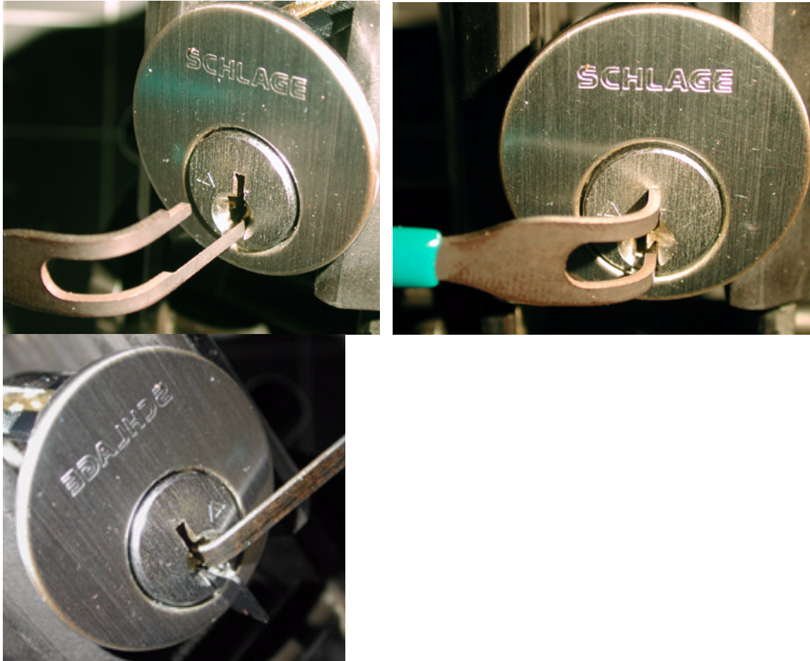
Figure LSS+2941 The Peterson pick tools for the Schlage Everest cylinder. The ET-2 is a combination tension wrench and second prong to raise the check-pin, while allowing ample room to insert a pick into the keyway. The ET-1 is an individual insert that enters within the undercut portion of the keyway to raise the pin. A separate tension wrench is inserted to apply torque.
