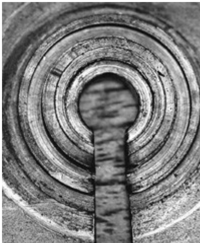
Figure LSS+307 A case ward is integral to the lock body.
