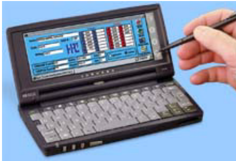
Figure LSS+823 HPC makes their codes available on handheld, laptop, or desktop computers. Shown is the HP720 handheld. Hewlett Packard produces one of the most sophisticated devices for this purpose. The HP720 is a 206 MHz. processor and allows the storage of more than 1 Gigabyte of data on removable PCMCIA cards.
