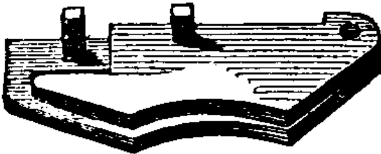
Figure 110. Pair of Barron's Tumblers. A, The Front Tumbler. B, The back Tumbler.
