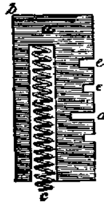
Figure 118. Bramah's with spiral spring, and False notches, as introduced in the year 1817. b, the point on which the key presses. c, The spiral spring. d, The principal notch or Main gating. eee, The False notches.
