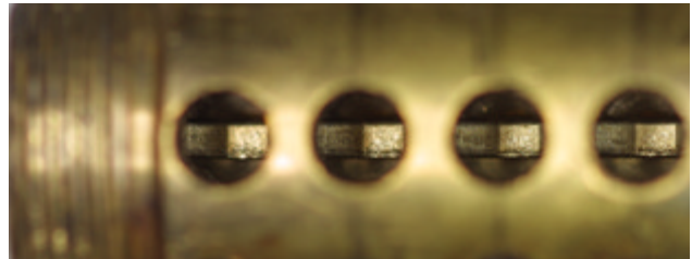
LSS+702b. In this photograph, proper alignment between each cut and corresponding chamber is shown. Note that the root is positioned at the center of each chamber, thereby allowing the tumblers to seat properly in each root.
