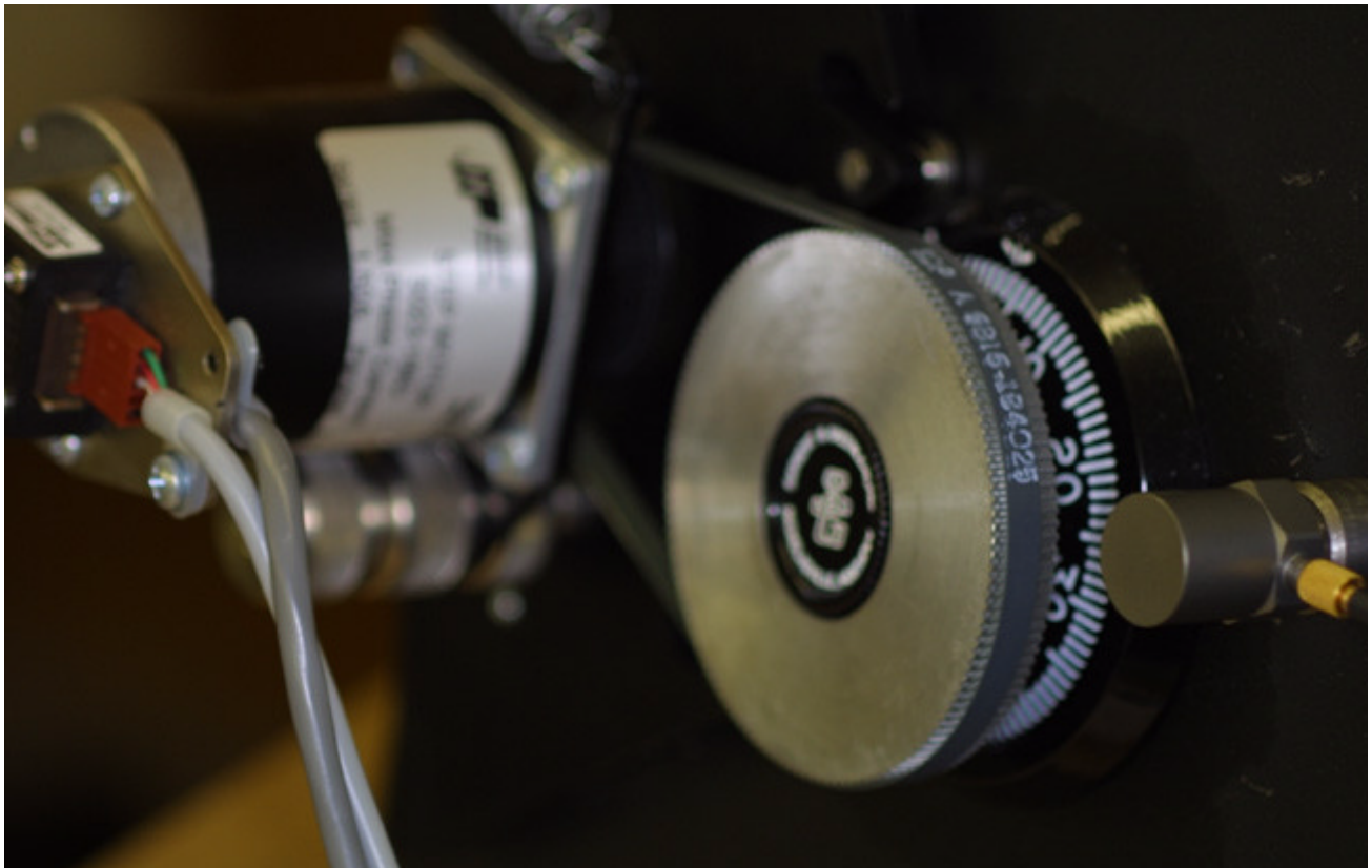
Figure LSS+3601 The Mas-Hamilton Soft Drill system is self-contained and integrated a laptop computer with sophisticated sensors that are attached to the front of the safe. Courtesy of Mark Bates.
