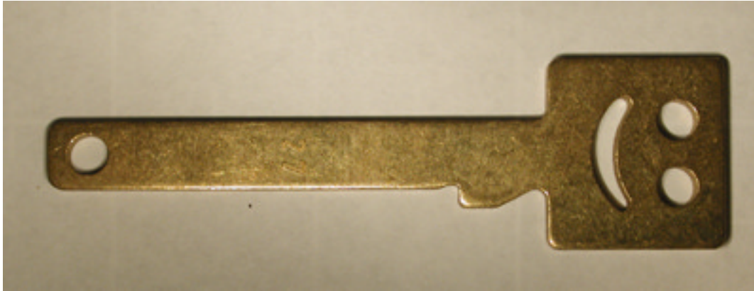
Figure LSS+831 The source key is measured mechanically with a thin probe. The correct Easy entrie blank key is then inserted into the cutting area and milled. There are at least five different blank thicknesses that are available.
