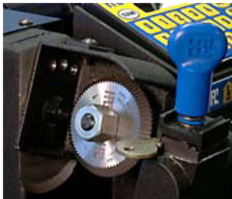
Figure LSS+826 The Codemax was one of the original HPC computerized code cutters.
