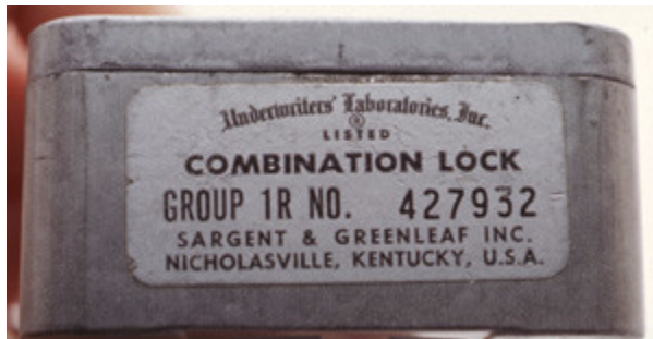
Figure LSS+3701 An example of a UL label for a safe lock. Courtesy of Mark Bates, The National Locksmith Guide to Modern Safe Locks.
