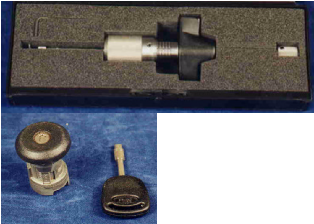
Figure LSS+3133 Ford Tibbe decoder and lock. This tool is produced by John Falle.
