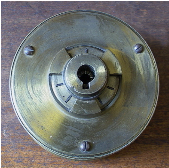
Figure LSS+118 The Bramah lock that was successfully opened by Alfred Hobbs.
