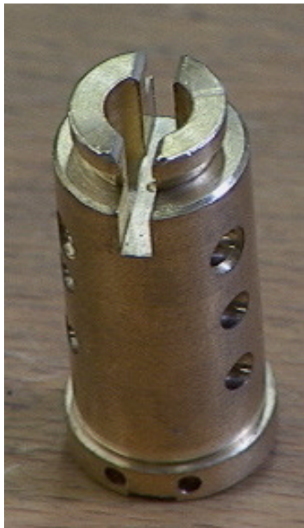
Figure LSS+1608 A plug is formed; drill resistant pins are inserted, then the individual chamber holes are drilled.
