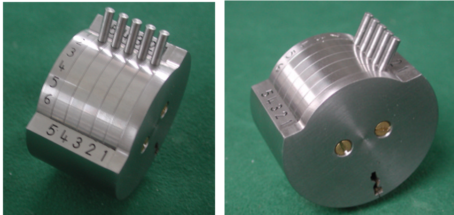
Figure LSS+3139 The tip of the tool is inserted into the Var-Key to select the proper depth segment. All possible differ pieces are contained within this self-contained unit.
