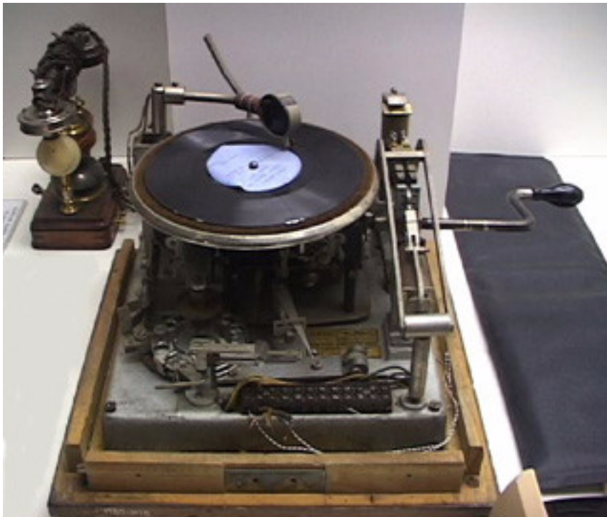
Figure LSS+4037. One of the original dial-up alarm reporting devices, used in
