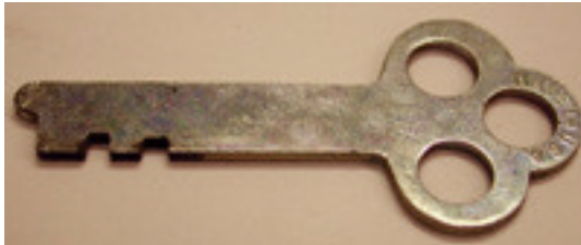
Figure LSS+316 A flat steel key, usually made of brass or steel. This key fits a safe-deposit lock.
