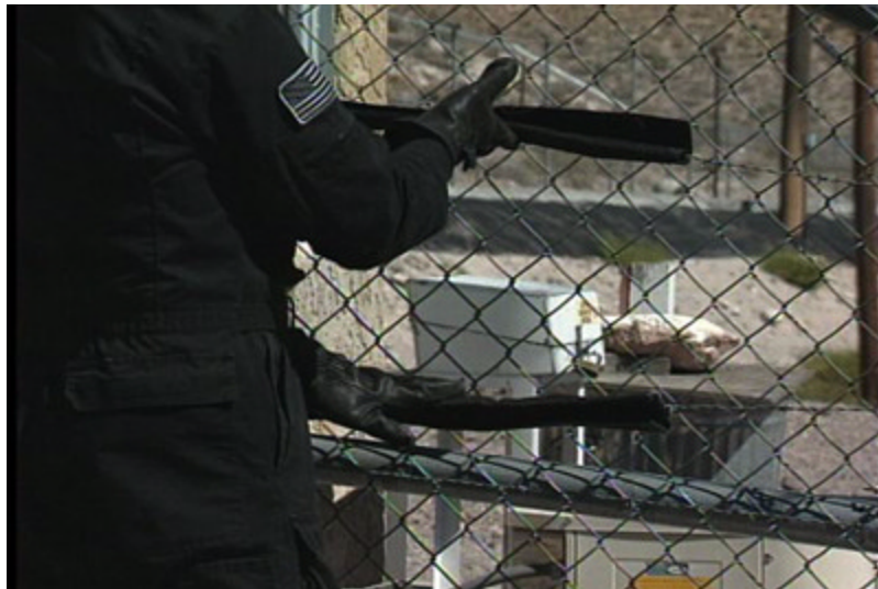
Figure LSS+4061 Taut wire systems can be defeated by spreading the wires, as shown, to create a gap for an intruder of up to fourteen inches.
