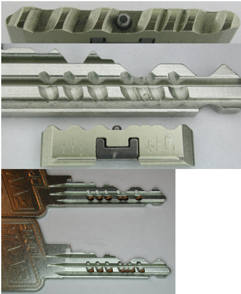
Figure LSS+1128 Evva DPI series dual sidebar lock, showing two different
