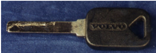
Figure LSS+3120 The Falle vehicle decoder system will open many laser track locks. Courtesy of John Falle.
