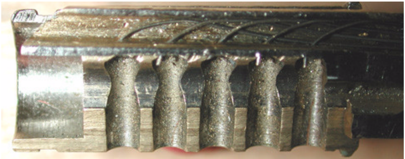
Figure LSS+2916 A blank key with the correct keyway profile must be produced by MSC for a specific lock. A hole is drilled to correspond with each pin chamber.
