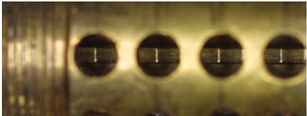
LSS+702a. A key must be properly positioned so that each cut is precisely centered under its corresponding tumbler. In this photograph, there is mis-alignment between chamber and the location of each depth cut.
