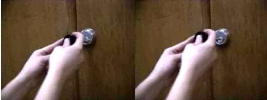
Figure LSS+2902 The use of the HPC Flip-it tool. The plug-spinner is a spring-loaded device that can spin the plug in the opposite direction without allowing driver pins to drop into lower chambers. This is especially useful if the plug is picked in the wrong position. To operate, the spinner main spring is wound; the tang is inserted into the keyway, and the spring is released. Photographs courtesy of HPC Interactive Learning Series.
