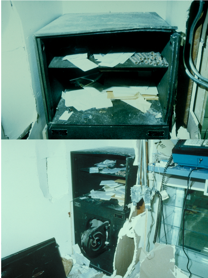
Figure LSS+3519, These photographs show an attack by the use of a wedge to pry apart and separate portions of the container. (top left ISP 51-3563, center 52, right 55, lower left, 54, right 53). Courtesy of Illinois State Police, Bill Sherlock.
