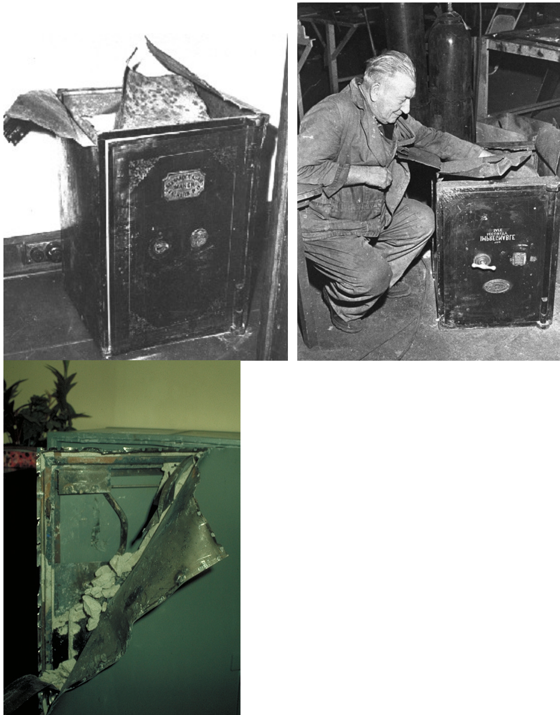
Figure LSS+3510. In this figure, peeling was accomplished from the corner using a cold chisel.
