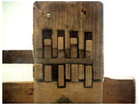
Figure LSS+102. Examples of different approaches to the original Egyptian pin tumbler design. These locks have been gathered from different countries, and demonstrate that the idea of using pins or pegs to secure a moving bolt or locking piece was not unique to any one society, although the Egyptians are credited with the initial concept. These exhibits are on display at the Science Museum in London.
