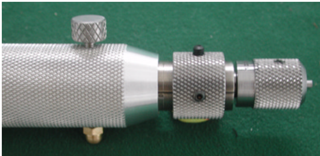
Figure LSS+3118 The Dom Diamond decoder system by John Falle. The lock in some respects resembles an Abloy because of the use of wafers.
