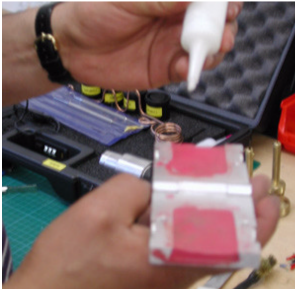
LSS+805 The aluminum mold is prepared by filling with clay, then smoothing the surface to insure uniformity in the impression.
