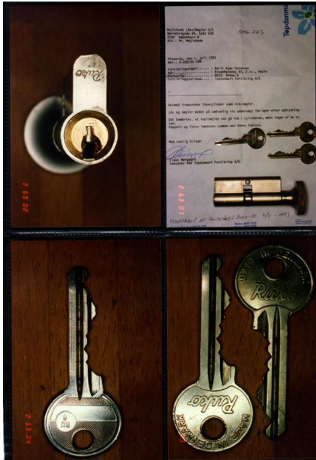
Figure LSS+2503 Sample forensic analysis report from Hans Mejlshede documenting receipt of evidence, photographs of pins within the lock, and the keyway.
