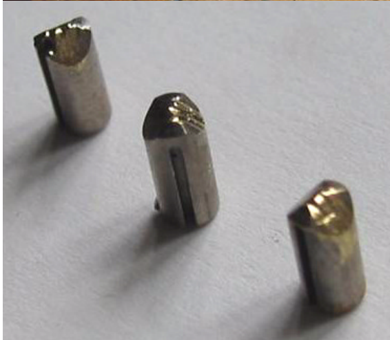
Figure LSS+2610 Examples of marks produced by different types of manual picks (above). In the photographs below, a Medeco Biaxial five pin cylinder has been picked using a probe to apply pressure against the edge of the pin. Although not a completely reliable means of opening, the technician reports that he could open this lock in between thirty seconds to one hour.
