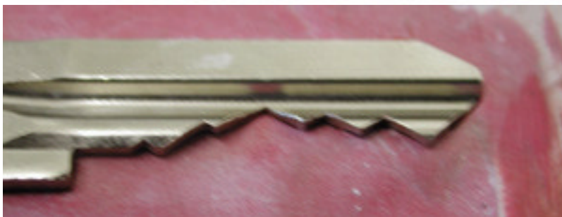
LSS+808 The source key is gently placed in position within the mold.
