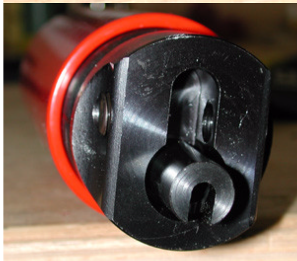
Figure LSS+3225 The MSC Lock Force tool can be used to remove profile cylinders from their housing.
