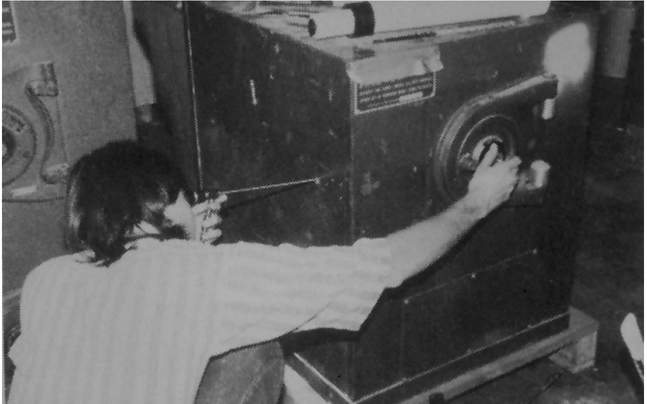
Figure LSS+3550 (ISP 18-2963) Side drilling and scoping the lock case.
