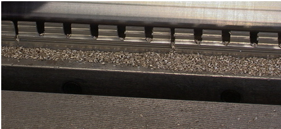
Figure LSS+1609 A broach is made of tool steel.
