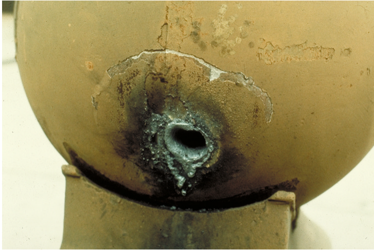
Figure LSS+3529. The thermic lance develops high temperature and can be utilized virtually anywhere. In the above photographs, the destructive power of this technology is shown. Photo ID: top left ISP 72-3563, right 73, bottom left 74, bottom right 75. In photograph 72, an older version of the lance is shown. Today, Broco produces this product in a small configuration that can be carried in a briefcase. Courtesy of Illinois State Police, Bill Sherlock.
