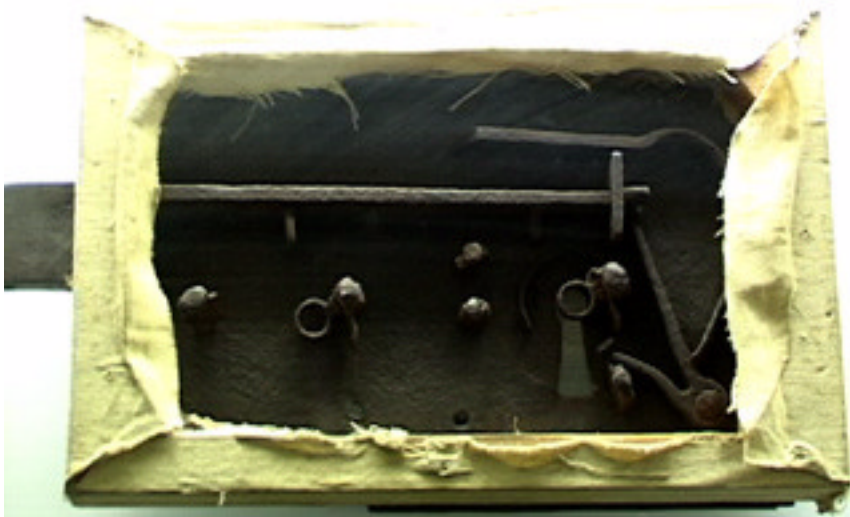
Figure LSS+109. This is a warded lock that was produced between the fifteenth and eighteenth century. Note that multiple keys were required.
