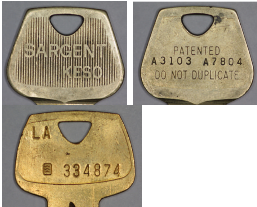
Figure LSS+607, examples of markings on a Sargent KESO key, and a Sargent LA sectional keyway series. Noted on the KESO there is an indirect code number and master key system number. On the Sargent LA keyway, the direct code 334874 appears. The key can be duplicated from this number.
