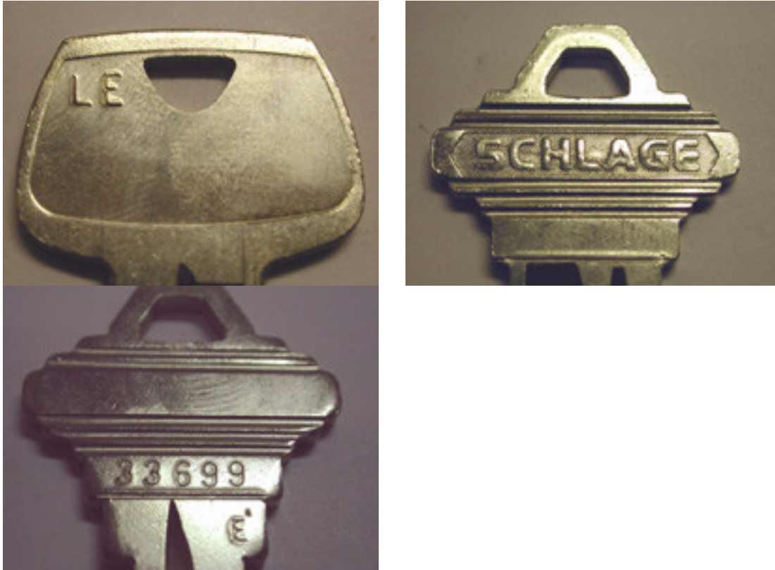
Figure LSS+318 Key heads provide identification of the manufacturer and specific blank.
