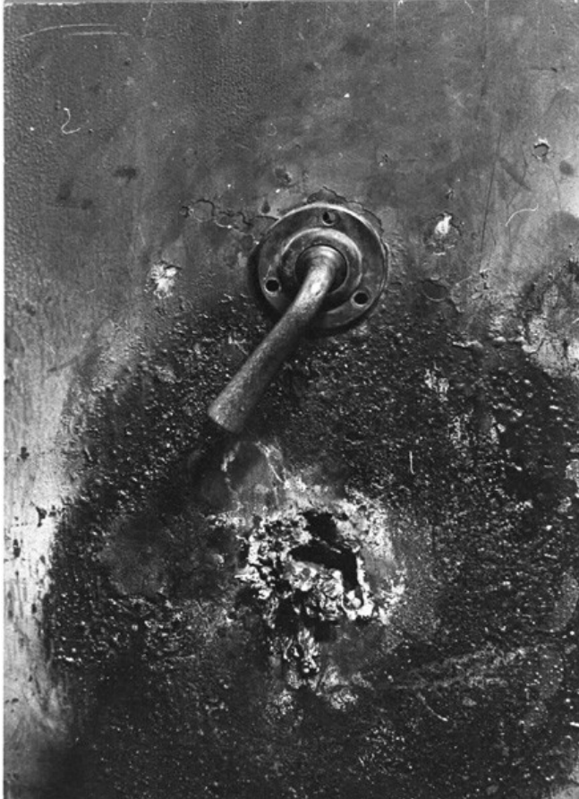
Figure LSS+3525, examples of torch attack. (left) incorrect tools were utilized on the side of the safe. This accomplished nothing. (right) a suspicious burn on the spindle, indicating perhaps an inside job.
