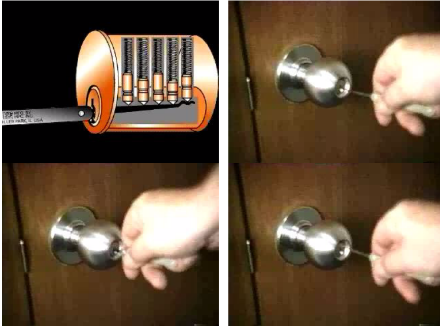
Figure LSS+2903 The pick must be free to access each pin individually without disturbing the position of adjacent pins. In the diagram, a rake pick has been inserted so as to reach the last tumbler. The photographs demonstrate how the pick is moved in and out of the lock. Courtesy of HPC Interactive Learning Series.
