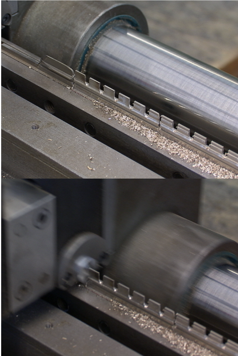
Figure LSS+1610 The broach is forced into the plug to form a keyway. The photograph on the right shows the plug being driven across the broach.
