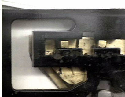
In this photograph, the levers have been raised to clear the gate, and the bolt has been
