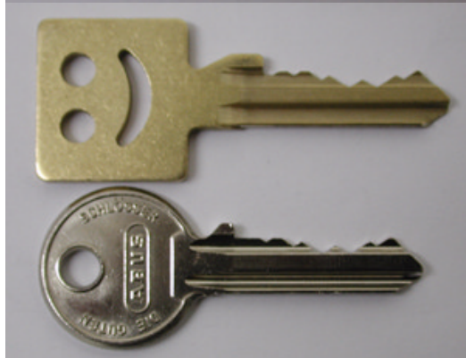
Figure LSS+833 The milled blank is not an exact replica of the source key, but will pass the wards within the keyway.
