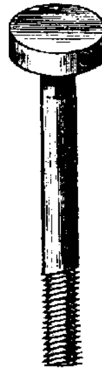
Figure 25. Cheese-headed screw. This was an early form of security fastening device
