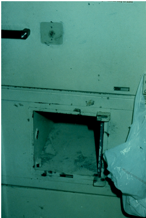
Figure LSS+3516, (top, ISP 40-3563, left, ISP 41-3563, middle, ISP 42-3563, and right, 43-3563). In this attack, the bolts were sheared by causing severe shock waves through the use of the welded bar to the front of the door. This attack changed the design of the round door from hardened to soft bolts . Courtesy of Illinois State Police, Bill Sherlock.
