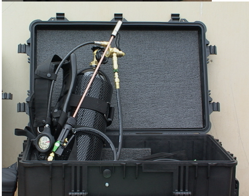
Figure LSS+3228 A smaller and newer version of the Broco thermic lance. This system utilizes a special oxygen bottle the newly designed trigger valve. The control valve can be utilized as shown, or connected via an extension hose to a separate oxygen source.
