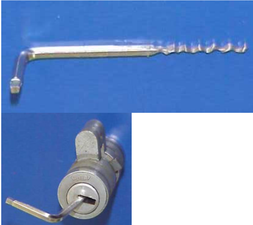
Rake picking tool for Lips lock, fashioned from an Allen wrench
