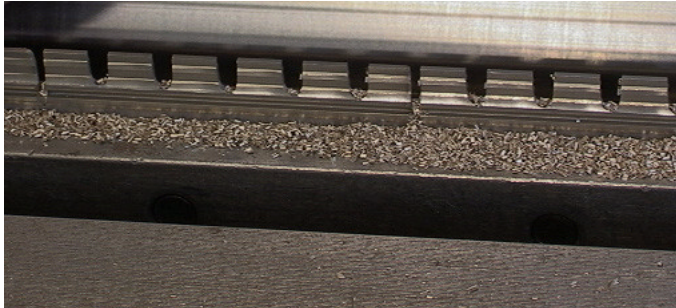
Figure LSS+1602 A broach for creating a keyway profile.
