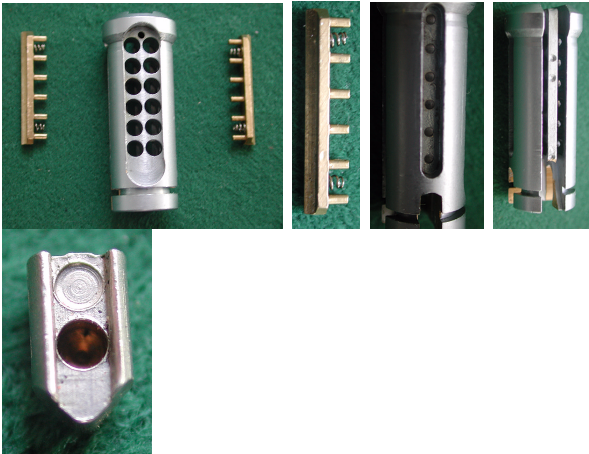
Figure LSS+3126 The BiLock plug contains two sidebars that must retract in order for the plug
