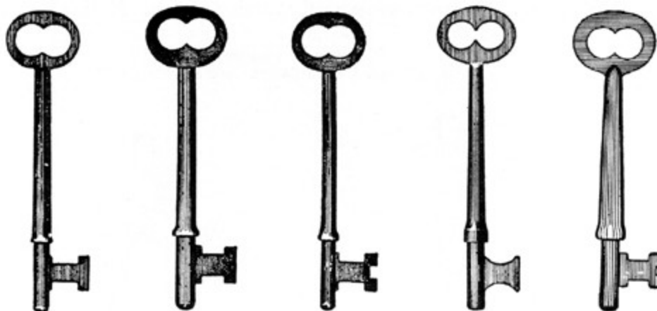
Figure LSS+903 Examples of three warded flat keys. From left, locker key, luggage, and padlock.
