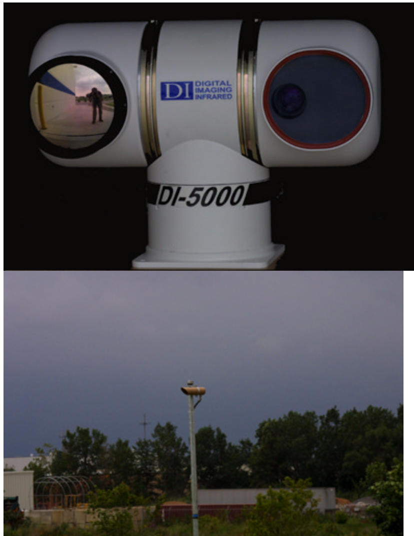
Figure LSS+4051 A thermal imaging sensor will detect body heat of an intruder.
