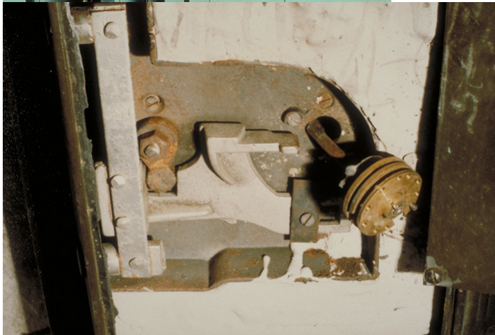
Figure LSS+3508. Punching involves the wheel pack being forced inward (left, ISP 35-3563), as shown in the photograph (ISP 34-3563). Courtesy of Illinois State Police, Bill Sherlock.
