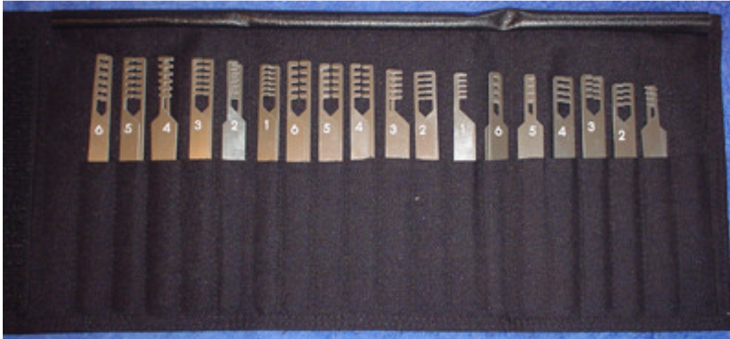
Figure LSS+2927 The John Falle comb pick set. These picks have been designed for different cylinder chamber sizes and spacing.
