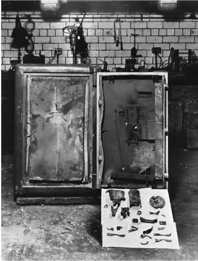
Figure LSS+3522. (Left), an attack using a torch where there was obviously no knowledge of where to cut. In the photo (right) the burglars burn and cut the bolt works. The parts are displayed.
