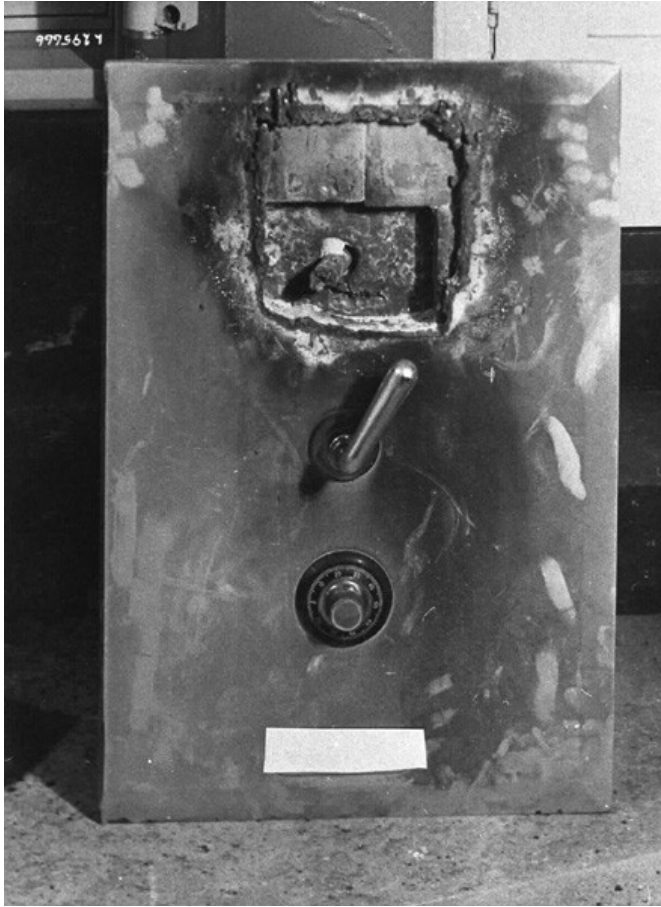
Figure LSS+3527, (left) a torch attack where burglars cut a portion from the door for access, and (right) where part of the skin was removed to access the bolt mechanism.
