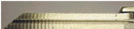
Figure LSS+304 The bitting surface of a blank key is known as the blade.
