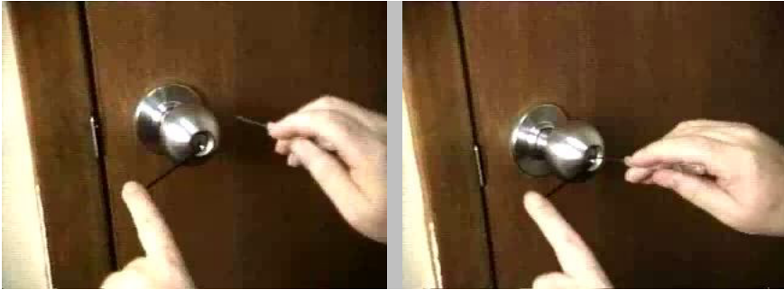
Figure LSS+2901 Methods of application of torque with the tension wrench. Courtesy of HPC Interactive Learning Series.
