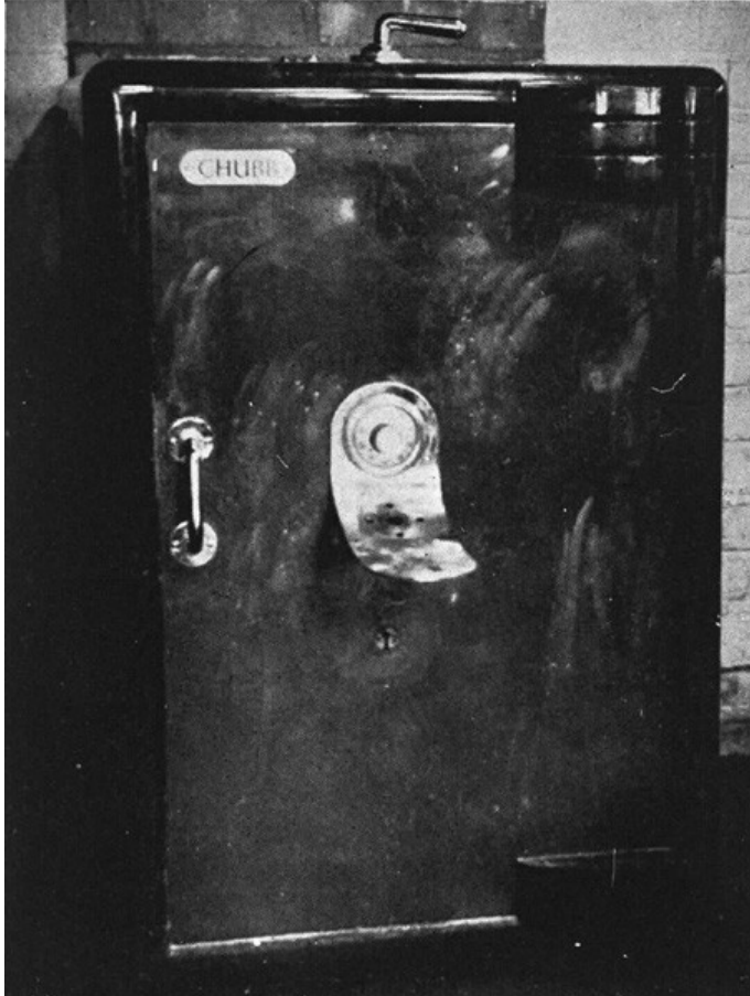
Figure LSS+3532, a free-standing Chubb safe was attacked with explosives. The violence of the blast blew the mounting plate away from the lock.
