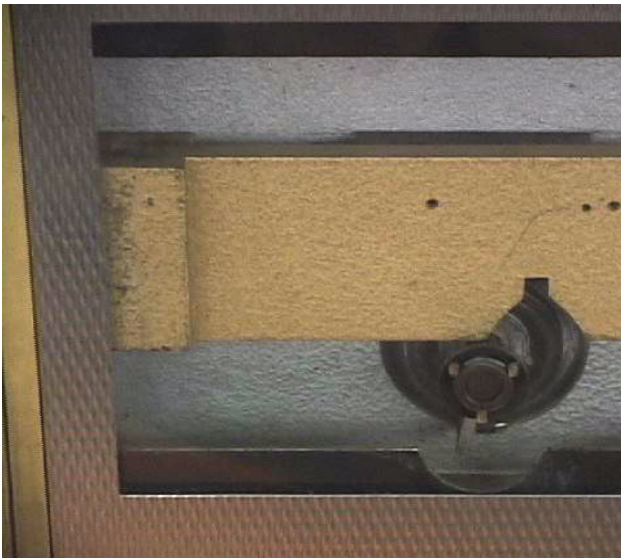
Figure LSS+108. This mock-up of a warded lock demonstrates its principle of operation. The key is allowed to rotate the bolt only when the obstructions are cleared. This and the following illustration were produced by the Science Museum, London.
