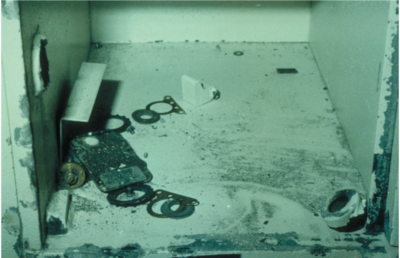
Figure LSS+3518 (top left, ISP 44-3563, top right ISP 45-3563, and bottom ISP 46-3563). This was a pound attack in a pattern burglary in four locations having the same layout. The door was pounded (45) with many hits. The parts shown inside (46), including the door stop after the tack weld was broken.
