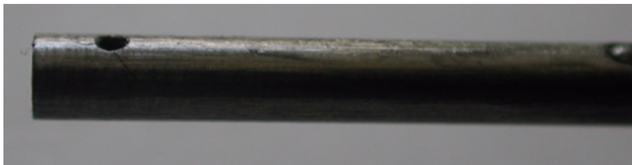
Figure LSS+3101 The John Falle Pin and Cam system relies upon the movement of a bearing under each moving pin that is inserted into the die corresponding to
