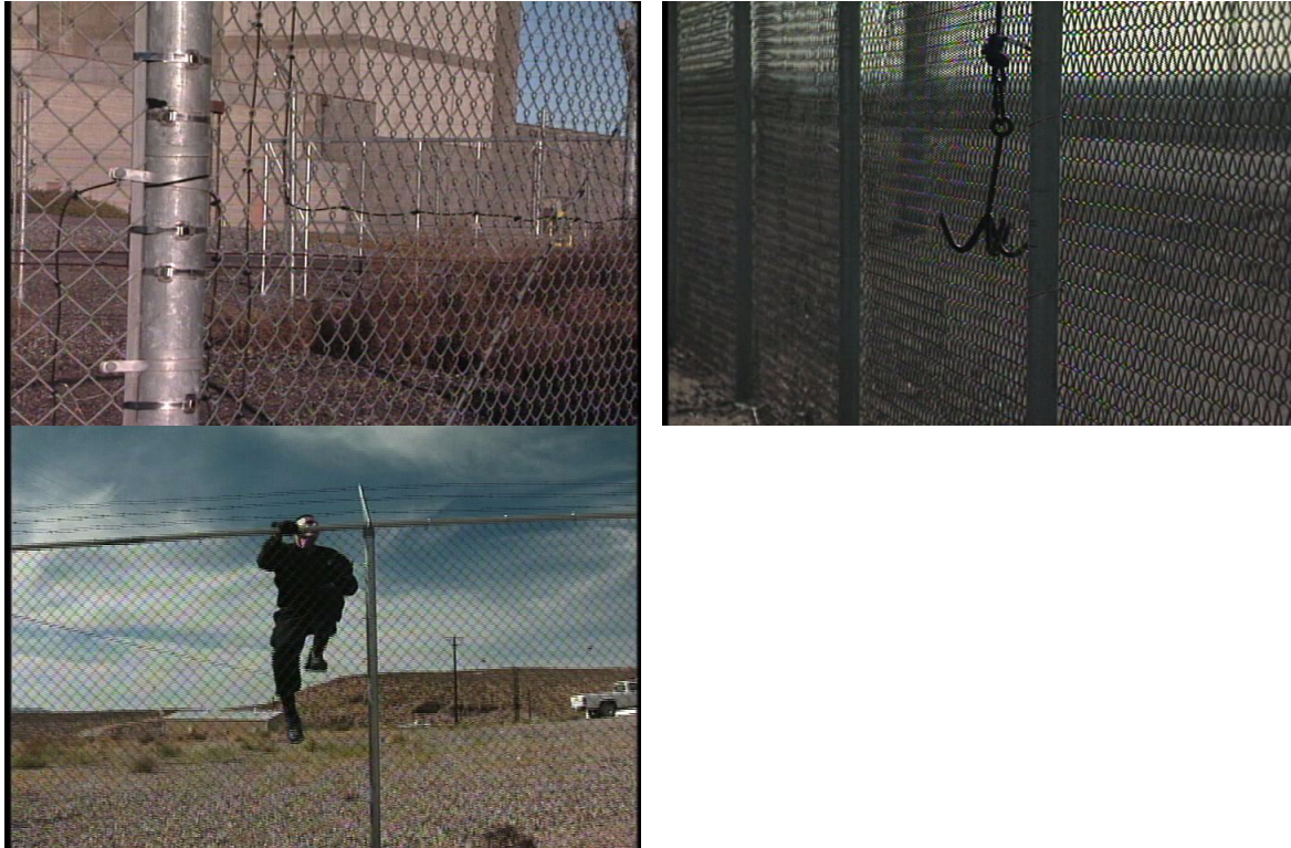
Figure LSS+4056 A fence vibration sensor will trip from the use of hooks or a climber. Courtesy of DOE Office of Security and Safety Performance Assurance
