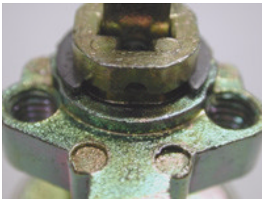
Figure LSS+302 An arc ring retains the core.
