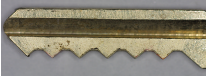
LSS+701c. This code-cut key shows the symmetry of each cut.
