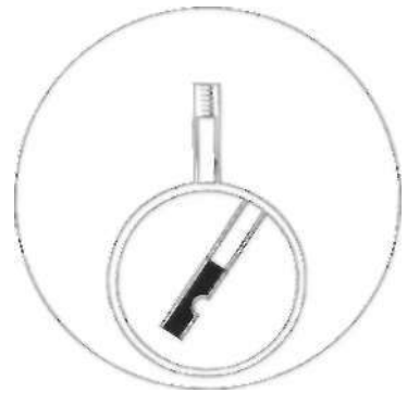
Front view—key inserted & plug rotated
