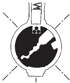
As change key rotates, construction balls fall into hole in the side of plug
