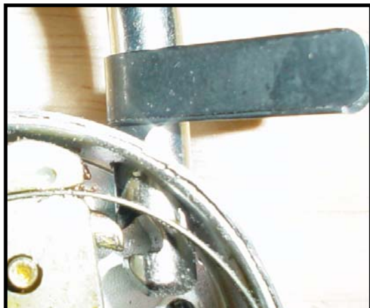
Unlocked – Bolt Retracted/Shim Turned.
