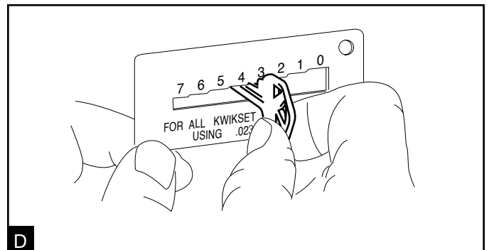
Key measurement Measure cuts of key or keys as illustrated, and write down key cut combinations.
