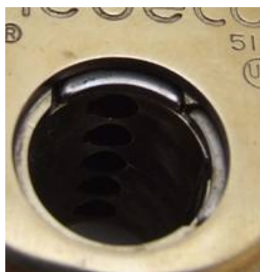
Fig. 10- Crescent's position in cylinder
