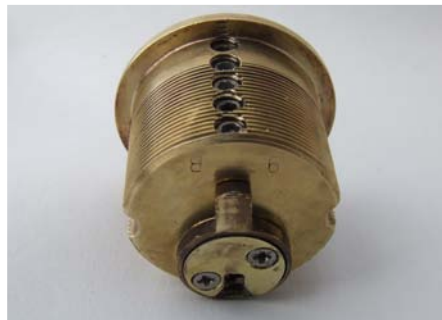
Fig. 2- Rear of Medeco Biaxial lock showing the cam and cover
