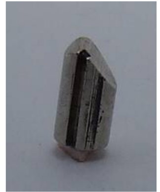
Fig. 16- Side view of a pin. The true sidebar slot is on the left, the false one is on the right.
