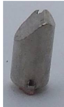
Fig. 13- Side view of pin showing long and short chisel face
