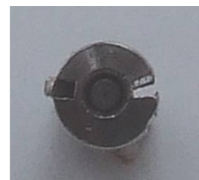
Fig. 15- Top view of a pin. The tang is the protrusion on the left hand side. The indent roughly opposite it is the sidebar slot. The center circle is a steel pin.
