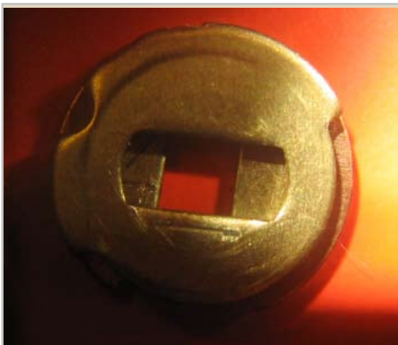
NOT COVERED: TURNED 90°, THE SPACER & SECOND CODE DISC PROVIDES VERY LITTLE COVER.
