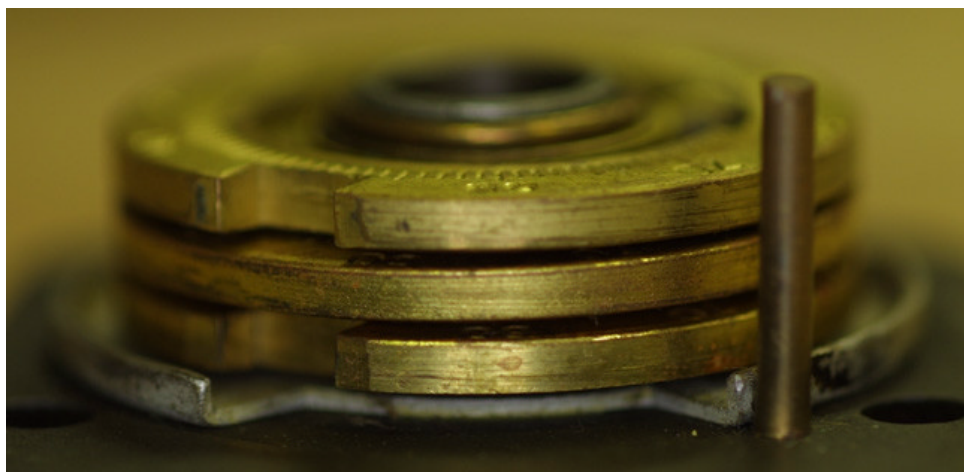
Figure M13. Yale OC5 geared roller fence. Only the left contact is read.
