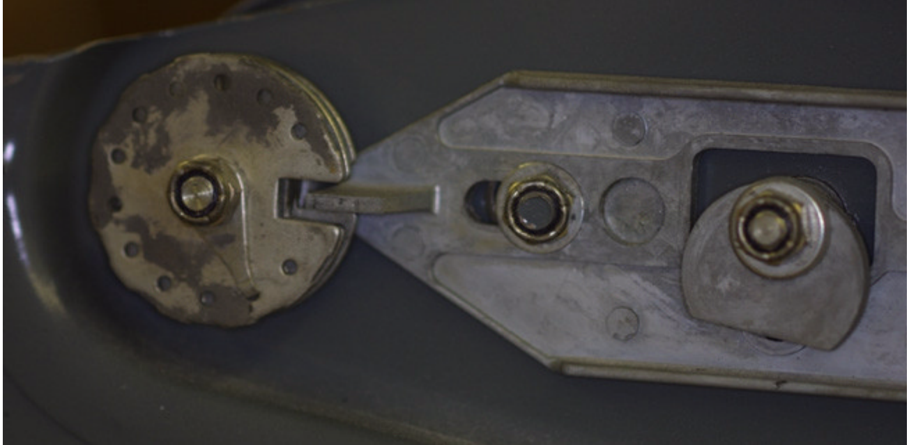
Figure M10. Straight tail piece. Pressure can be applied directly against the wheel pack to determine gate position.
