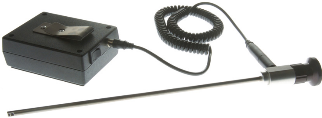
Figure 10: A 10 inch by .200 inch 90° fiber optic borescope with portable 30 Watt halogen light source. An angled borescope provides a good view of the gates and/or the fence through a small opening.
