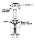
The assembly is now checked with the correct key for the lock. When the key is turned 90°, either clockwise or counterclockwise, the locking bar gates in the combination discs should be aligned. The drum is now oiled through the opening in the drum for the locking bar.
