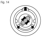
The starting position of the cylinder has been reached. The cylinder drum and housing are once more engaged. The combination is scrambled and the key may now be removed without resistance.
