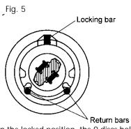
In the locked position, the 0-discs hold the locking bar and the returns bars in place.
