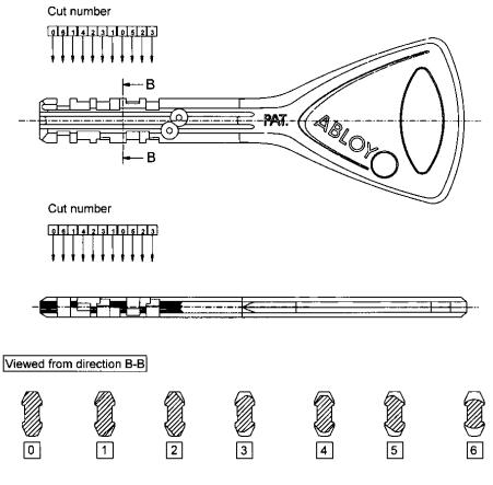
An o-cut is an uncut portion on the key, whilst a 6 is cut all the way around. All other cuts are formed using precise angles and depths.
