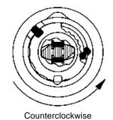
As the key turns, the 0-discs lift the locking bar, and move the return bars to the locked position. As the return bars
