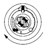
Position of the number 2 disc after a clockwise operation
