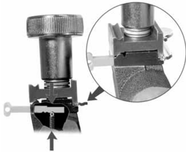
Fig. 3B. Properly seated key in jaw C.
