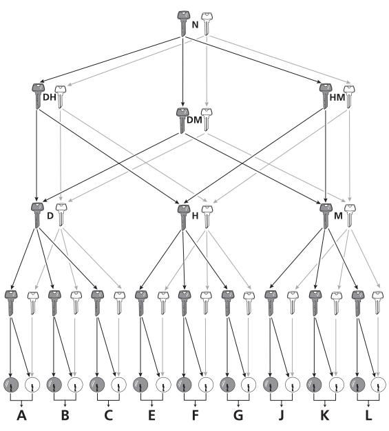
SARGENT Signature keys are produced with a special feature that allows them to operate Signature cylinders as well non-Signature cylinders within the same keyway family. The standard key does not contain the special feature which allows it to operate a Signature cylinder but will continue to operate non-Signature cylinders.
