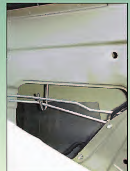
7. Inside the door, the tip of the tool is hooked onto the lower of the two horizontal linkage rods.
