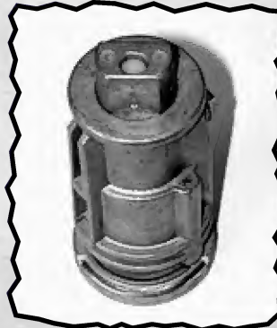
15 If the plug actuator is not in the plug when you re-assemble it, the anti-theft device located in the rear of the plug will not properly engage the security components in the steering column. The car will not start if there is no contact.
