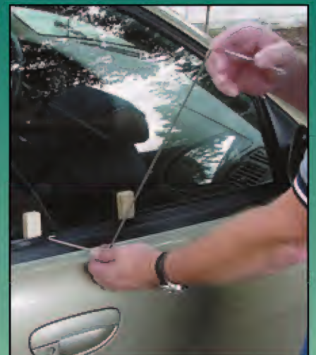
2. The front door can be unlocked with the TT-1017 tool.
