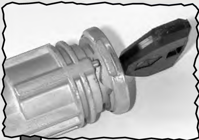
12 To disassemble the lock, rotate the lock counter-clockwise and depress the stop pin.
