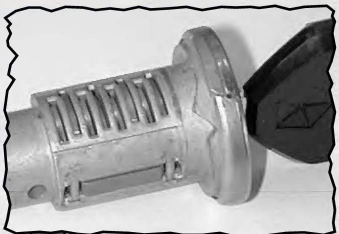
13 The cylinder plug removed. The lock plug uses eight tumblers and has a sidebar.
