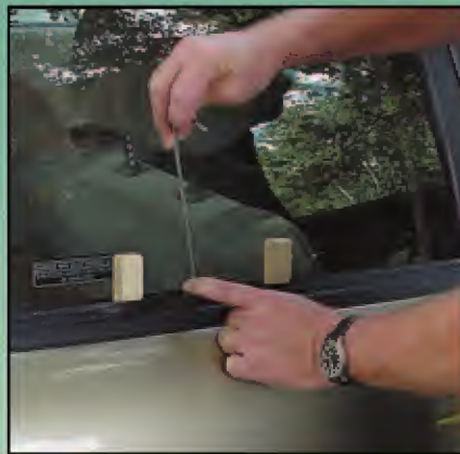
6. Twist the top of the tool in order to bind the linkage and then lever the linkage forward.
