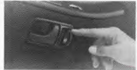
2. Back side of the inside handles is now inaccessible.
