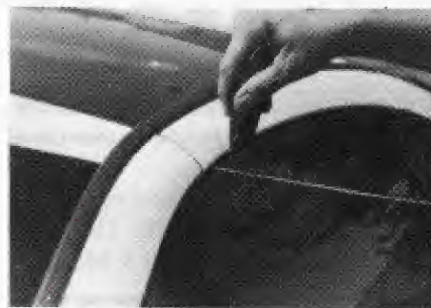
4. Fishing a key ring on a string through the window.
