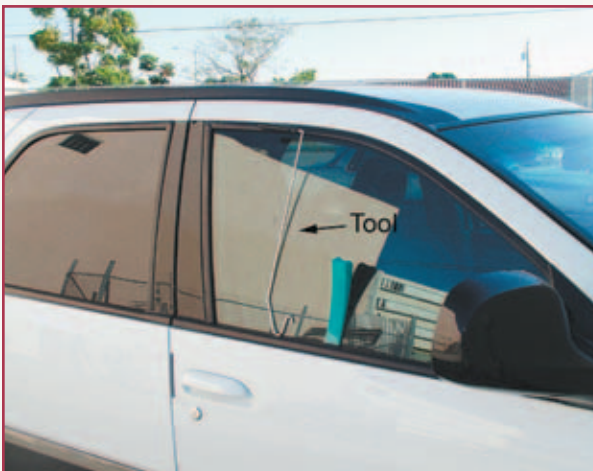
2. Point tip of tool forward.
