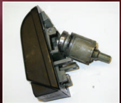
17. You can now remove the cylinder from the rear.
