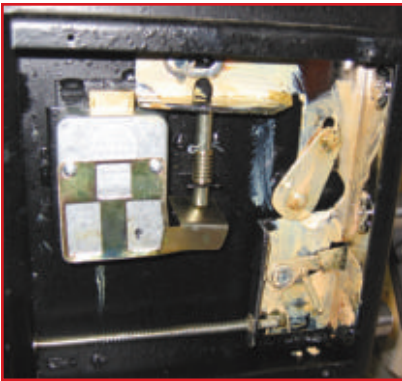
4. Internal configuration of this Amsec Door. Lock is VU.
