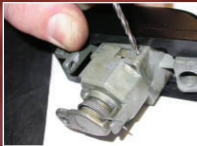
14. To disassemble the lock you will need to remove the roll-pin that holds the lock body together. Drill a hole behind the pin as shown.
