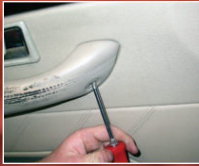
6. Begin by removing the Phillips screw under the handle rest.
