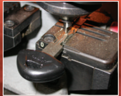
23. I used a Matrix machine to cut the center groove.
