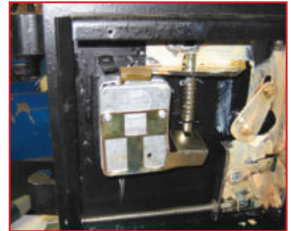
6. Lock bolt punched and relocker set off.
