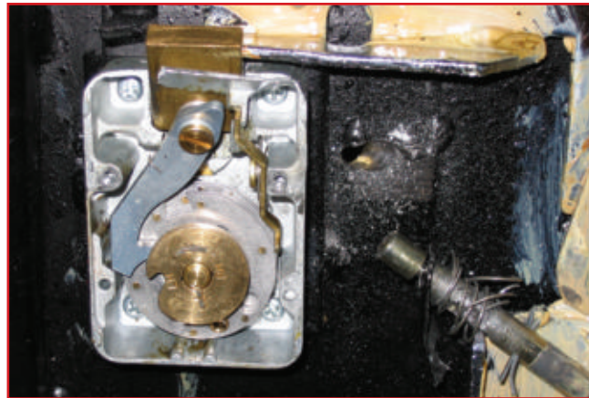
9. External relock falls off (finally) and safe door opens!
