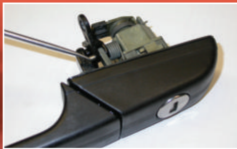
12. The door lock contains all cuts to make a complete key. Disassembly is not difficult. Begin by removing the pin that secures the handle linkage connector.
