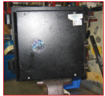
3. Back of the Amsec door with chrome label over change key hole.
