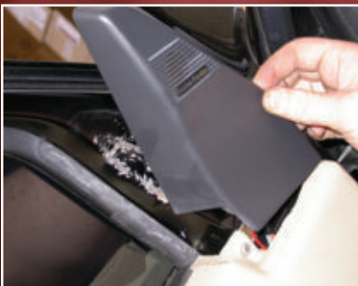
8. Remove the triangular plastic trim piece on the top of the door panel.
