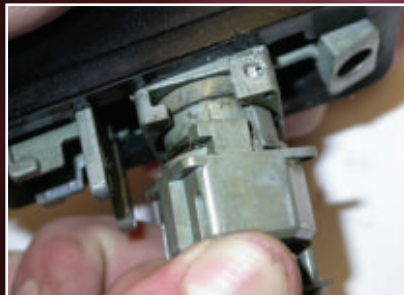
16. Rotate the rear part of the lock body and it will disengage from the front. There is a large spring between the two parts.
