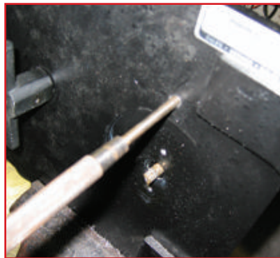
5. Punching dial and combination lock spindle.
