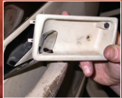
7. Remove the plastic trim piece behind the inside handle.
