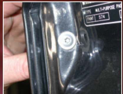
10. You can now remove the panel. Remove the Torx-27 on the door edge and the lock can be removed.
