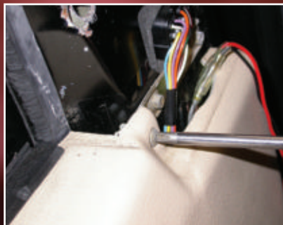
9. After removing the trim piece, this will give access to another Phillips screw.
