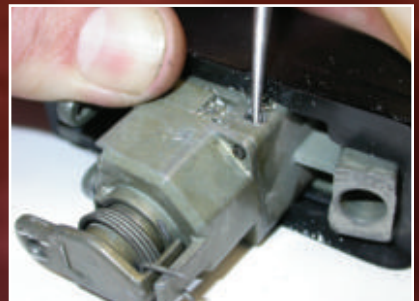
15. Use a sharp pick to push the roll-pin out.
