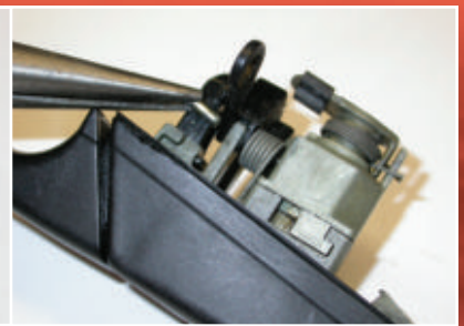
12. The door lock contains all cuts to make a complete key. Disassembly is not difficult. Begin by removing the pin that secures the handle linkage connector.
