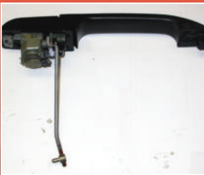
11. The lock removed.
