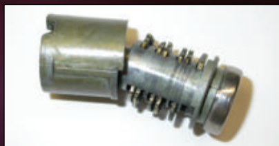
18. The plug easily slides out of the housing.
