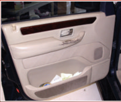
5. It is easiest to remove the panel and then remove the lock.
