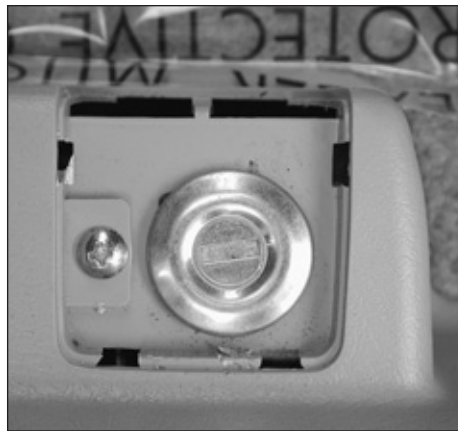
8. There is a small cover on top of the lock. The cover can be removed to expose a screw that does not need to be removed.
