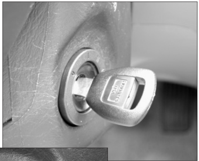
17. The key you want to start the car cannot be programmed from your back pocket. You must put the key in the ignition lock cylinder and turn to position "II".
