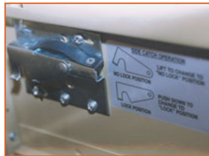
7. View of the side catch that locks drawer. Lots of adjustment here.
