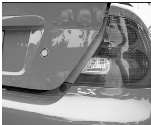
1. The trunk lock cylinder is located on the right side of the trunk lid.
