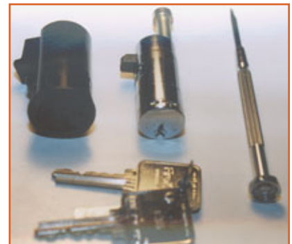
3. Cylinder, case, and Medeco keys. Screwdriver is to remove cylinder from case. Pop out locking slide is at 9:00 o'clock.
