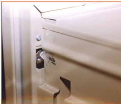
5. Rear of cylinder with locking bar stud removed prior to raising front of door.
