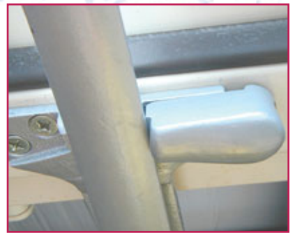
16 When the arm contacts the cushion dead stop, it acts like a shock absorber.
