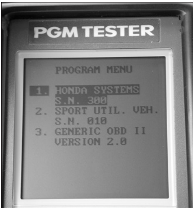
18. Select Honda Systems from the start up screen on the PGM tester.
