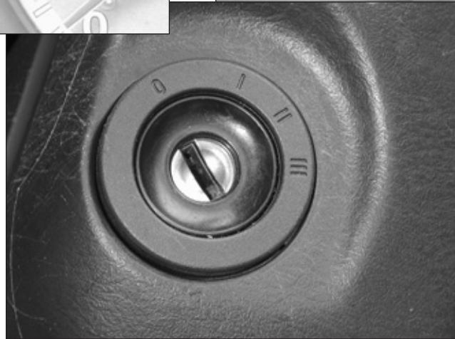
17. The key you want to start the car cannot be programmed from your back pocket. You must put the key in the ignition lock cylinder and turn to position "II".
