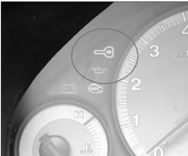
16. There is a green "key" indicator light in the instrument cluster for the transponder system.
