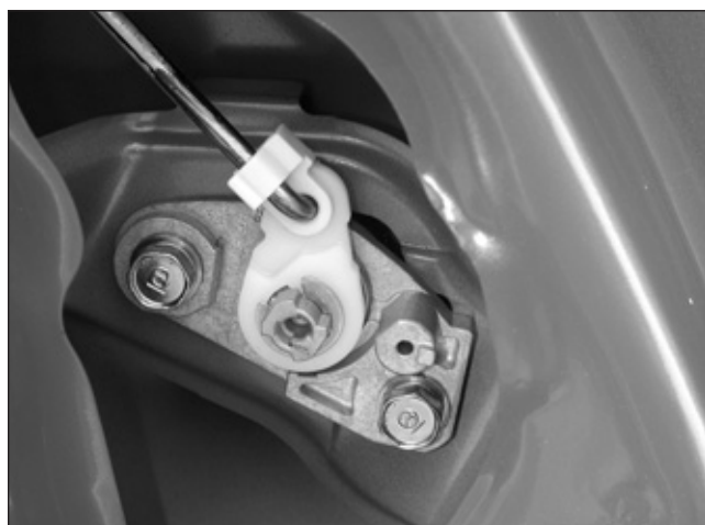
2. The lock cylinder is secured with two 10mm bolts. Remove the bolts and disconnect the linkage rod.
