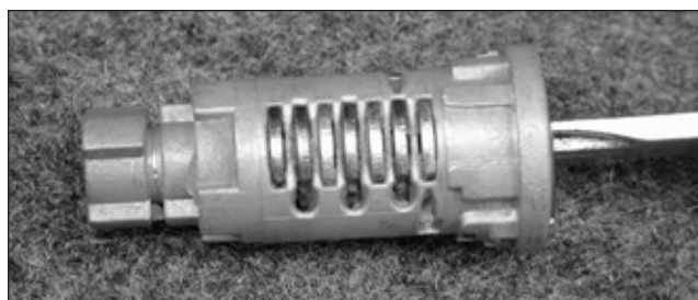
5. The trunk lock cylinder plug contains 7 tumblers in positions 2 thru 8; the first tumbler is not used in this lock.
