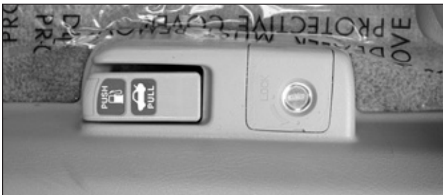
7. There is a lock cylinder for the release of the trunk lid. It is located on the floor to the left of the driver's seat.
