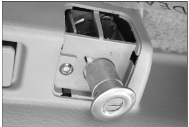
9. The cylinder will then slide right out the top.
