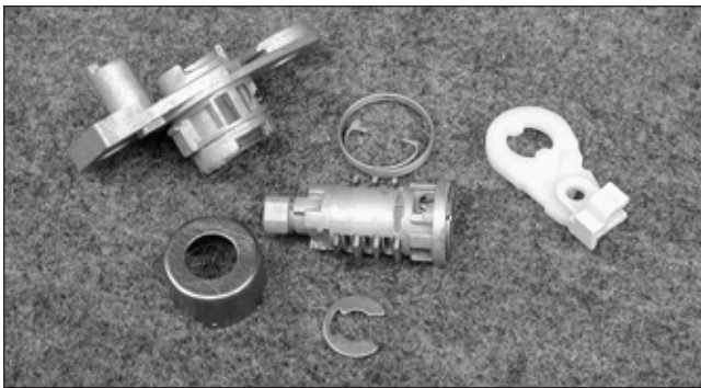
6. The trunk lock components.
