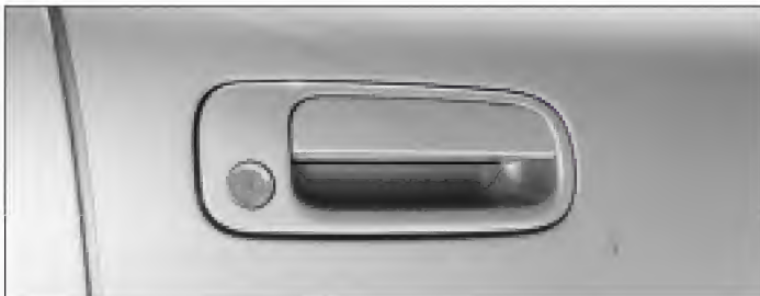
Photograph 1. The door lock cylinder is part of the door handle assembly.
