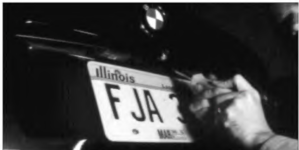
2. Remove the screws that secure the trunk lock cowl.
