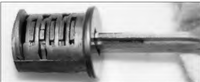
Photograph 33. The cylinder plug contains tumblers in positions five through eight with a spit tumbler in position eight. The valet tumbler is in position nine.
