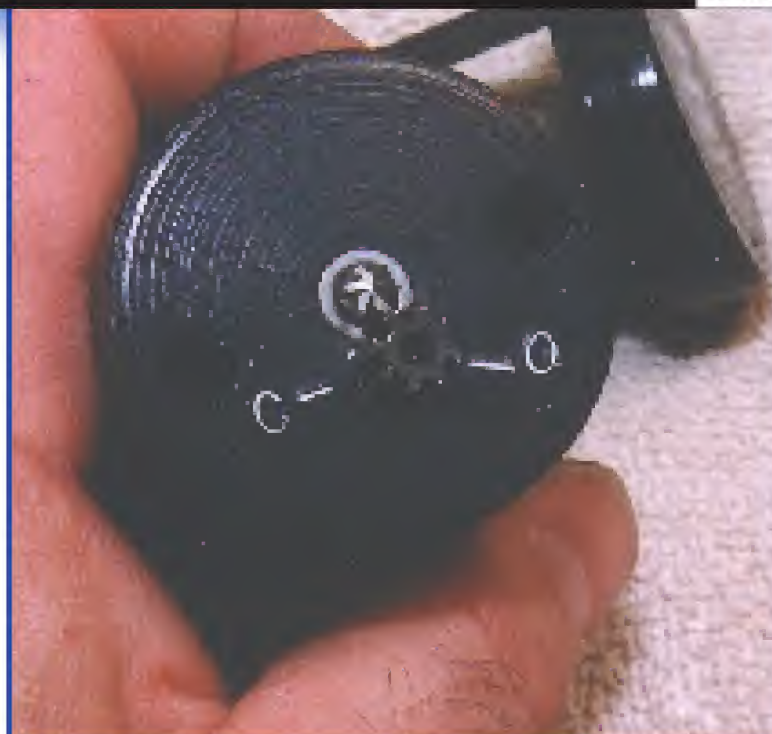
5. The "C" and "O" indicator is for the center, offset left and right cuts.
