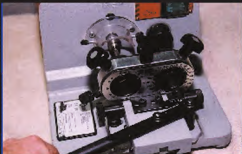
14. The left side of the Synchronized Self Centering Device T10 is line indexed with the most popular spacing positions. The right side provides a numbered scale in degrees.
