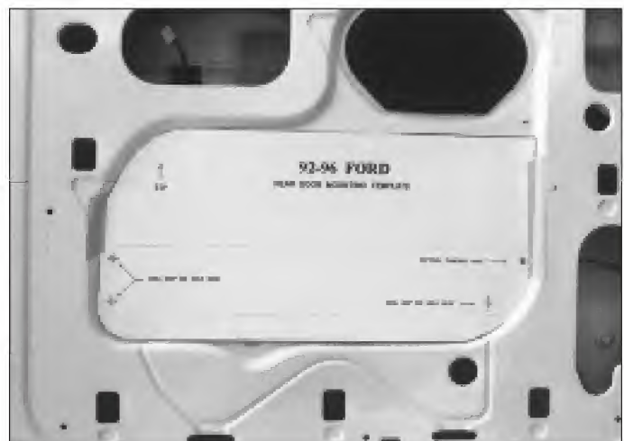
Photograph 1. Mounting template for rear door.
