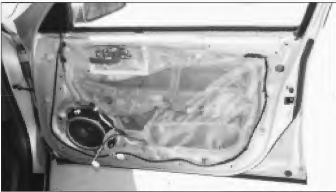
Photograph 8. A view of the door with the panel removed.
