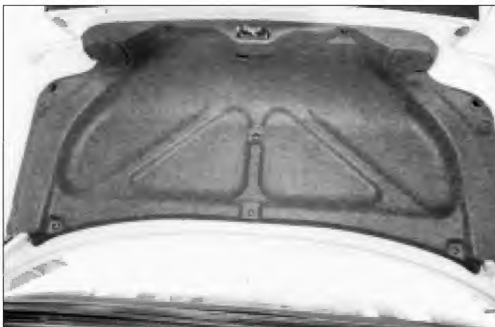
Photograph 18. The cloth-like material liner must be pulled back or removed to access the trunk lock cylinder.
