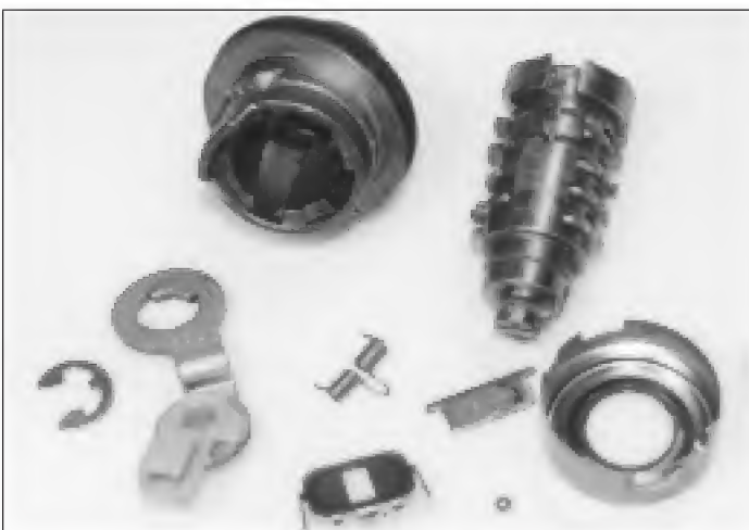
Photograph 27. The trunk lock disassembled, is shown.
