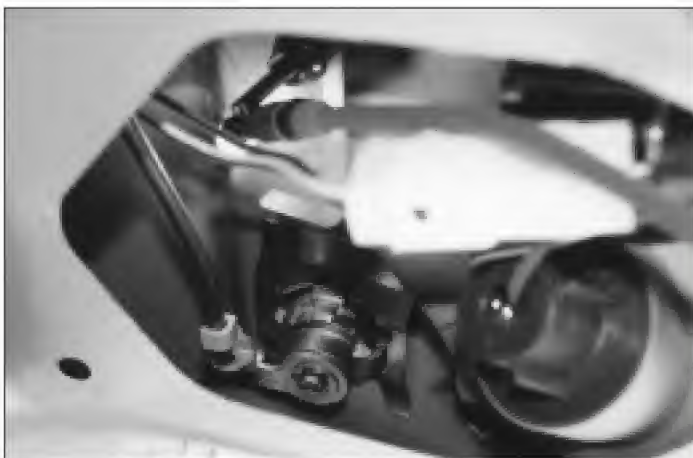
Photograph 20. The trunk lock cylinder is held in place by the standard style horse-shoe clip.
