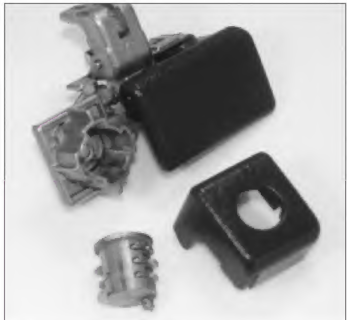
Photograph 34. The glove box lock disassembled.
