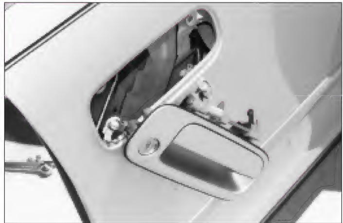
Photograph 11. To make life easier for you, disconnect the linkage rod to the handle pull and slide the handle assembly out of the door to remove the 10mm bolt holding the lock cylinder into the handle.
