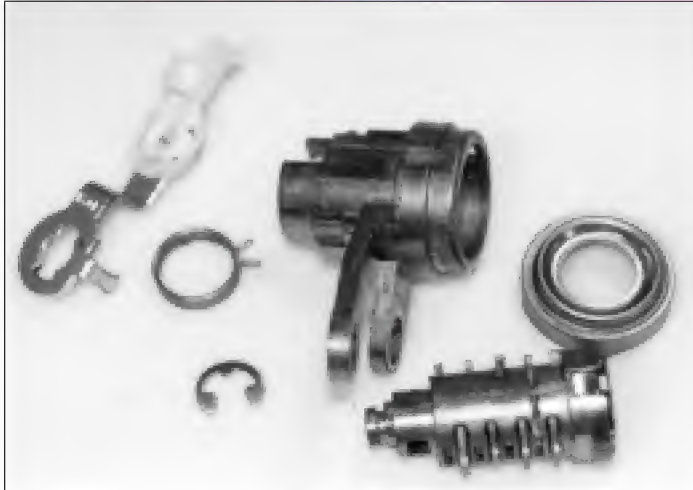
Photograph 16. The door lock cylinder disassembled.
