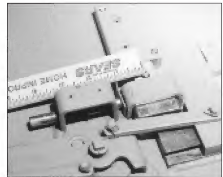
3. Relock plunger is blocked by case cover over lock.
