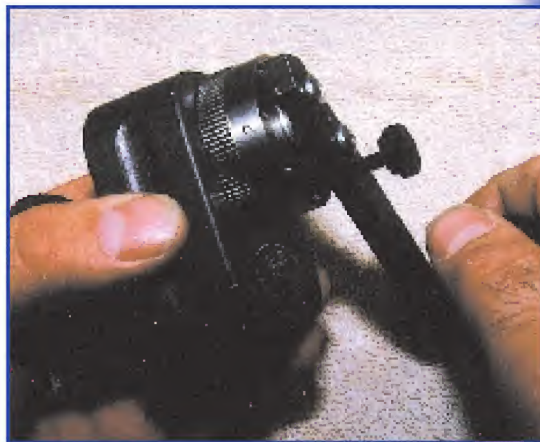
3. Rotate the crank with your right hand in a clockwise direction until the crank bottoms out against the base.
