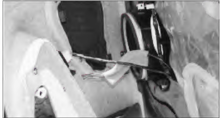
Photograph 7. Now you can remove the door panel. It uses the standard plastic push-in clips. Once the panel is removed you will need to disconnect the associated door panel wiring.
