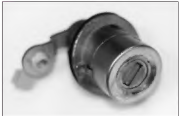
Photograph 21. The trunk lock cylinder removed.
