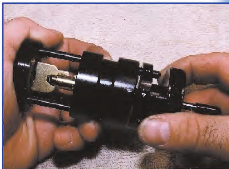
6. Compressing the key onto the positioning post with the key retainer face plate with your left hand, turn the cutter handle wheel with your right hand.
