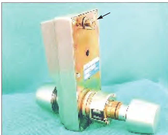
12. Changing the combination on the 1000 is done by turning the cam on the back of the lock to the LEFT.
