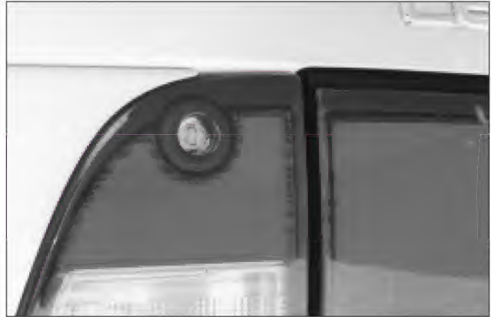
Photograph 17. The trunk lock cylinder is located under the rear taillight and trunk lid centerpiece.
