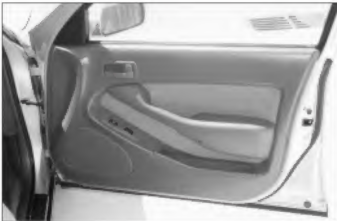
Photograph 2. The door panel must be removed to service the door lock cylinder.
