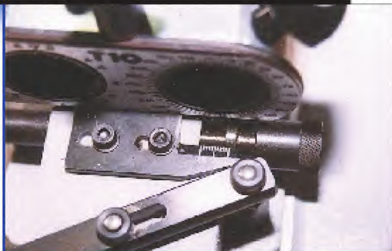
15. At the bottom right of Synchronized Self Centering Device T10, there is a height adjustment which will change the thickness of the cut at the webbing.
