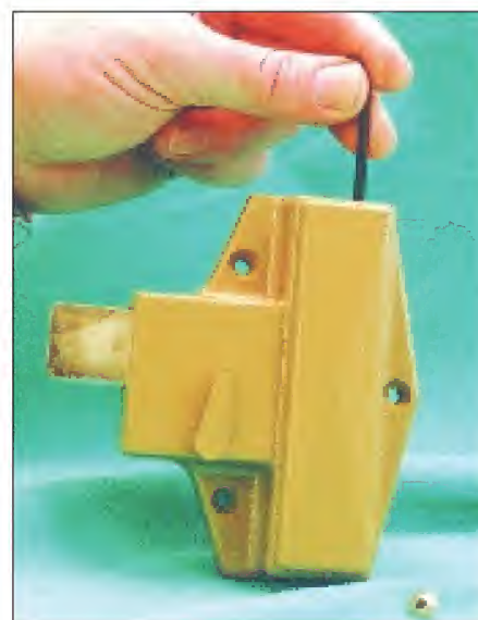
3. Remove the screw on the top or bottom of the lock housing and insert the wrench into the hole and depress the lockout slide.
