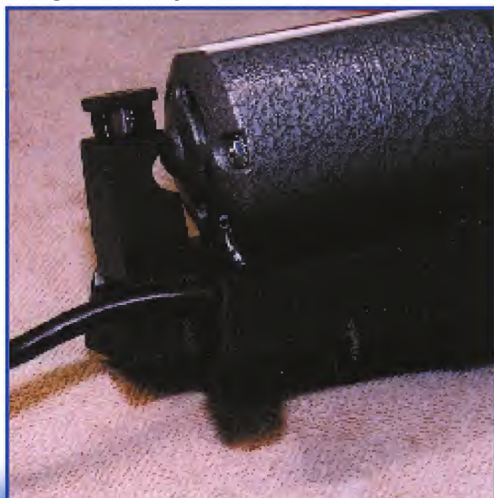
9. (Below) The stop pin can be adjusted for duplication or origination of keys with cuts within cuts.
