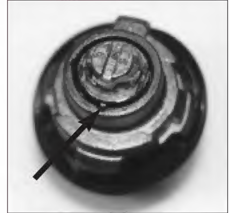
Photograph 24. Be aware of the ball bearing in the back of the lock as you disassemble it.
