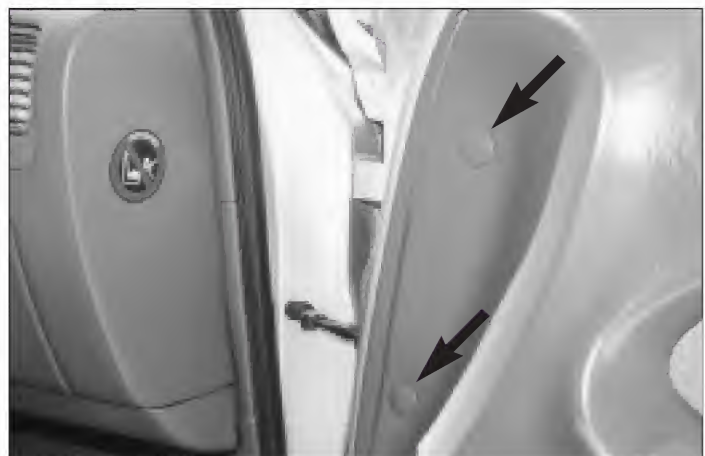
Photograph 5. There are two Phillips-head screws located at the forward section of the door panel and hidden under trim covers. Remove the screws.
