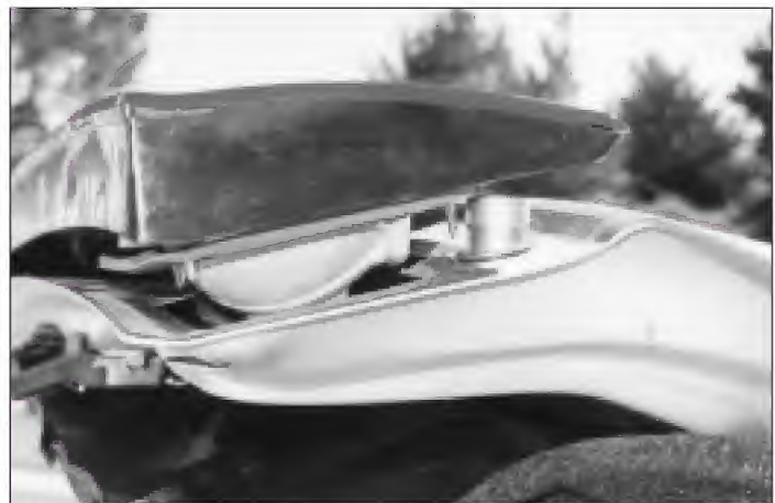
Photograph 19. Remove the 8mm nuts that hold on the taillight assembly to lift it up far enough to remove the lock cylinder.
