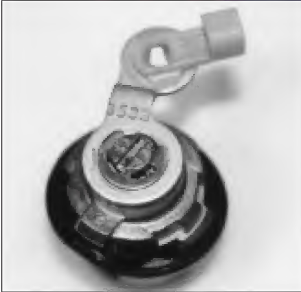
Photograph 22. To disassemble the trunk lock cylinder, remove the tailpiece and the face cap.
