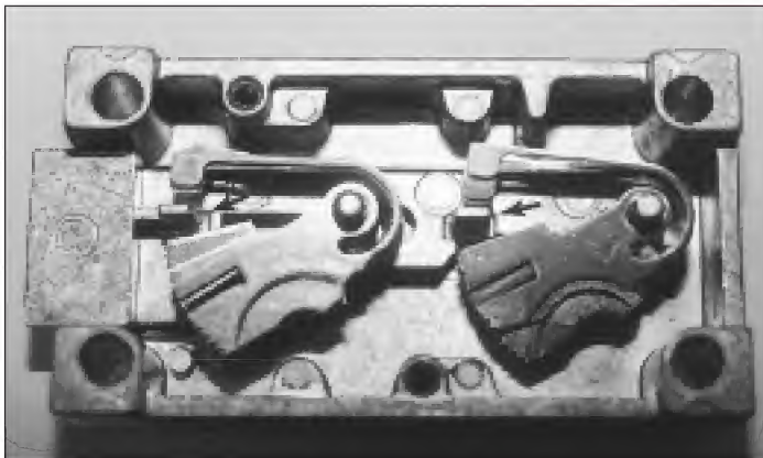
4. When the lock noses are pulled, tumblers drop below fence and lock can easily be opened.
