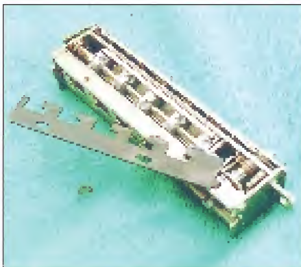
10. Lift the end of the unlocking slide at the end where the E ring clip was.
