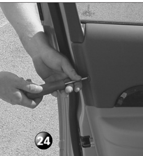
24 Remove the rest of the screws that can be found around the perimeter of the panel.
