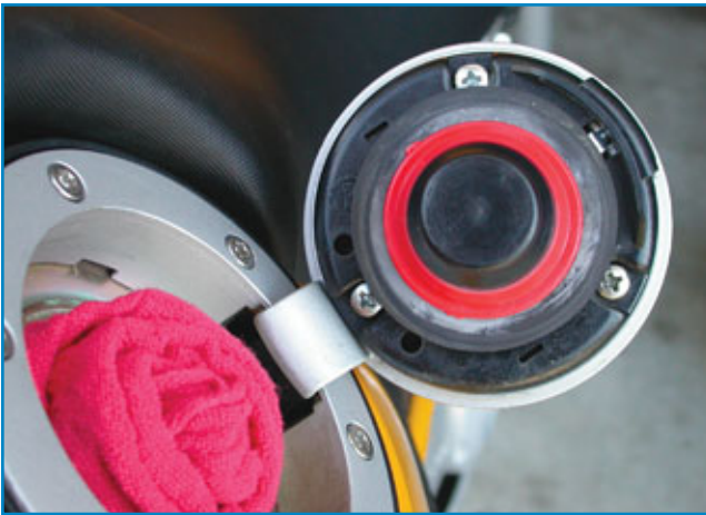
4. Stuff a clean rag into the filler neck so nothing falls into the gas tank. Then remove the three Phillips screws and remove the lock plate.
