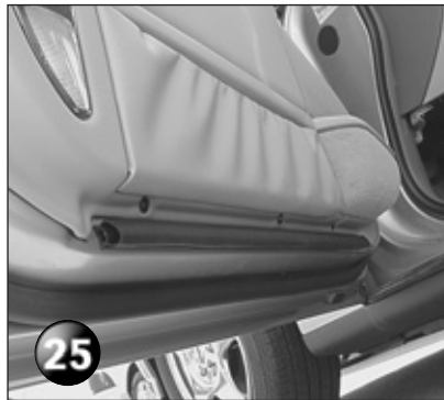
25 Three of these screws can be found along the bottom of the panel.
