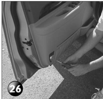
26 Once complete, pry the door panel off of the door.
