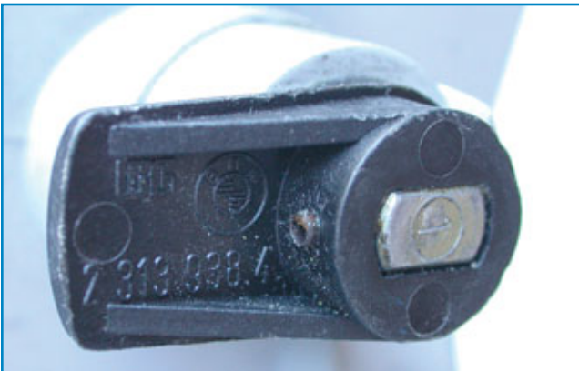
15. The tailpiece is held on by a roll pin.
