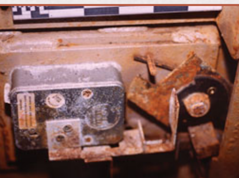
5. Door opened showing combination lock cover with attached complex relock activation bar.
