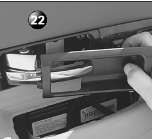
22 Carefully pry the trim from the front edge and slide it away from the handle.
