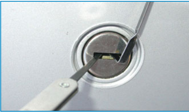
13. The rear compartment lock has just been picked 90 degrees clockwise. This lock was easy to pick by bouncing a rake between the wafers on top and bottom of the keyway.
