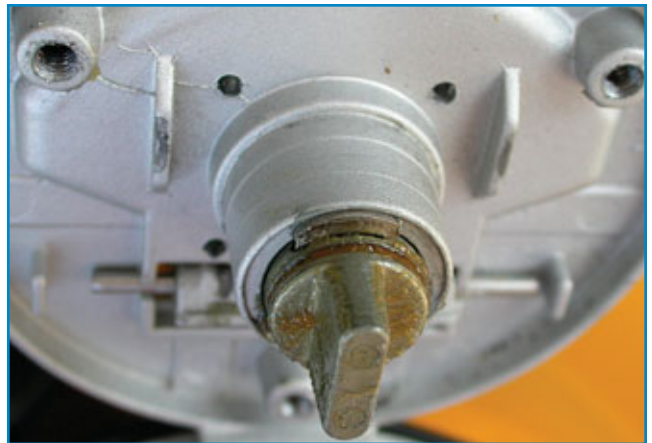
6. The wafer retainer is on the upper side of the plug. Depress it and push the plug out the front. Be careful and do not allow any of the wafers to fall or spring out.
