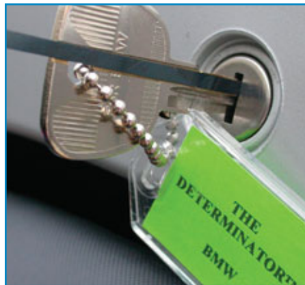
18. The Determinator™ for BMW automobiles works well on the rear compartment lock. The spacing and depths are the same as the automobiles except BMW motorcycles do not use the fourth depth.
