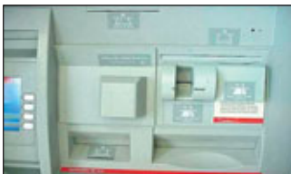
2. The equipment as it appears installed over the normal ATM bank slot.
