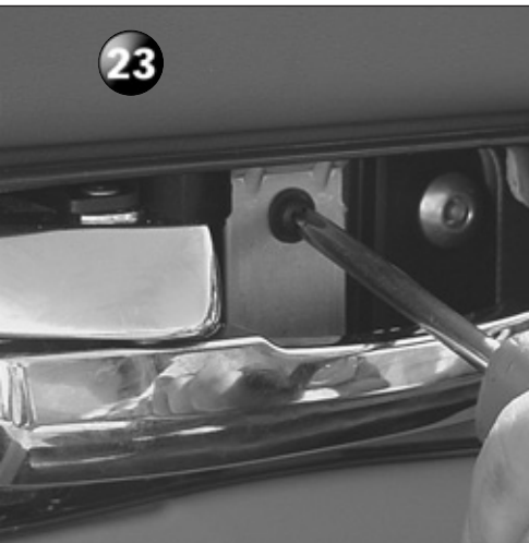
23 With the trim piece removed, a small screw is visible. Remove the screw.
