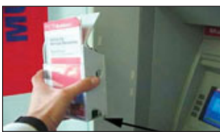
3. The PIN reading camera being installed on the ATM is housed in an innocent looking leaflet enclosure.
