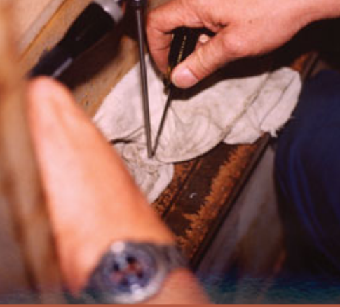
4. Borescope and shop rag inserted in the 1/2" drilled hole to view the change keyhole in the lower combination lock.
