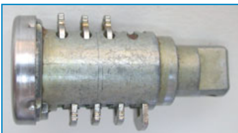
17. The rear compartment plug contains six wafer tumblers and a wafer retainer. The retainer serves no function that
