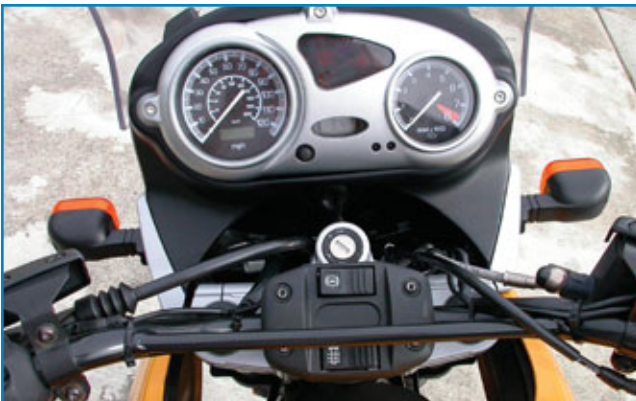
19. This view from the drivers' seat shows the ignition/steering lock located in front of the handlebars.
