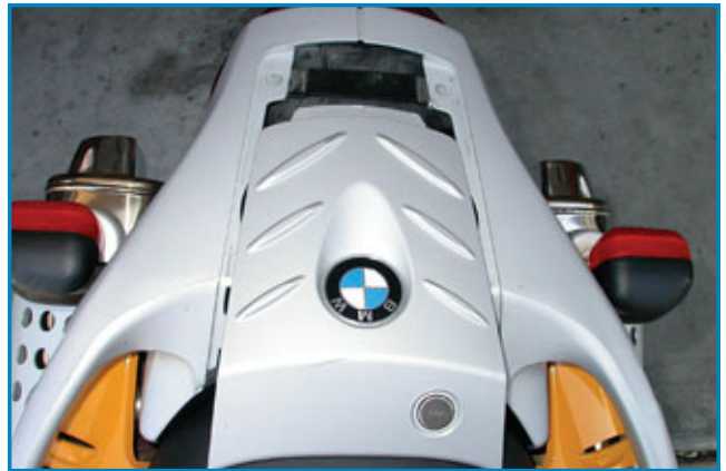
14. After you unlock the rear compartment, slide the cover forward and you can lift it off.
