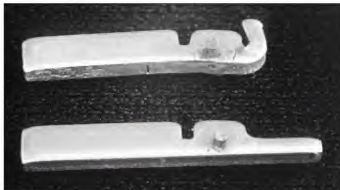
11. The bolt actuator tail has rolled over, which allowed the bolt to be pushed back into the bolt casing.
