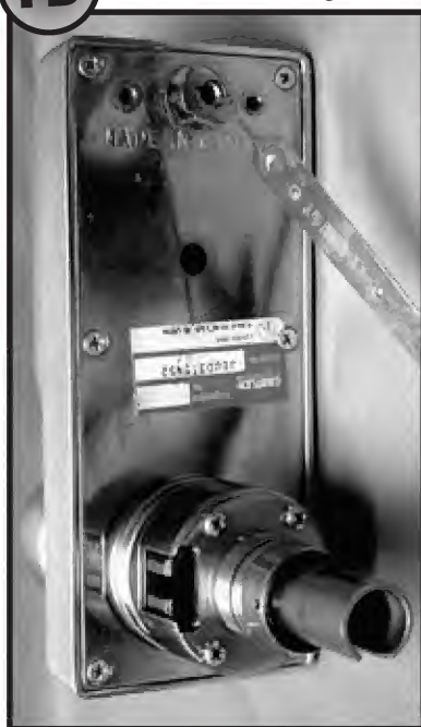
13 The spanner wrench is pointing toward the combination change sleeve.
