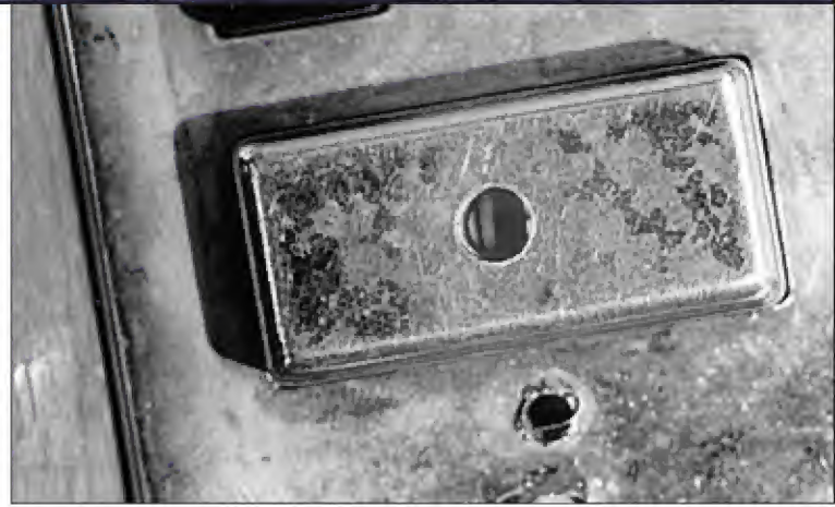
13. Drill a hole directly in the center of the large exterior button until you break through the material.
