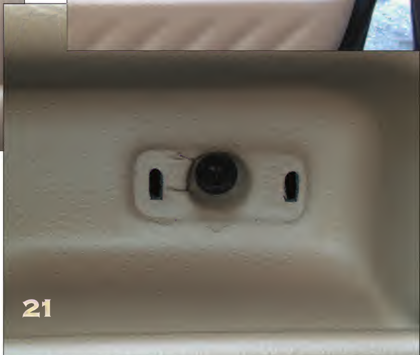
Near the rear of the panel is trim cover that hides a panel screw that must be removed.
