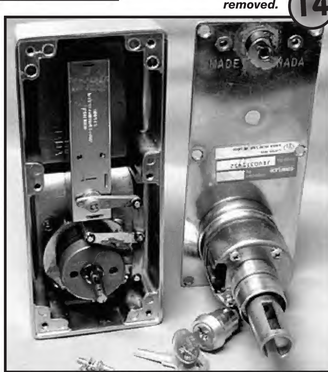
After removing the six small screws, the back plate assembly can be removed.
