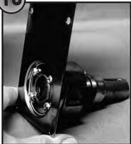
The end of the spanner wrench fits into a slot on the outside end of the sleeve.
