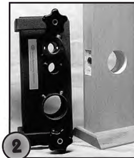
2 A lock mount prepped for a standard cylindrical lock.
