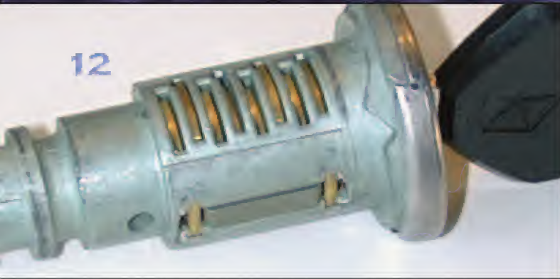
A look at the plug with all 8 tumblers and a side bar.
