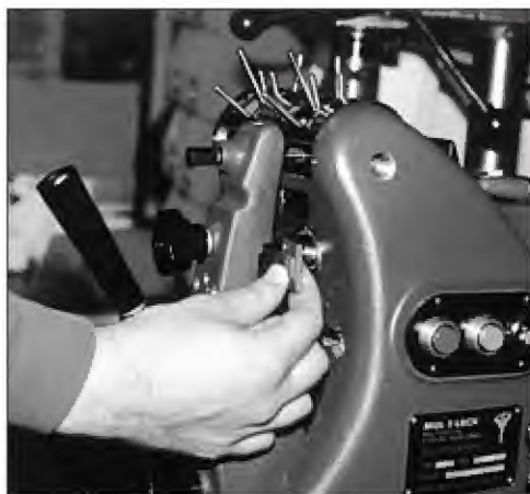
15. To cut a key, insert a key blank into the holder on the operating arm and tighten into place
