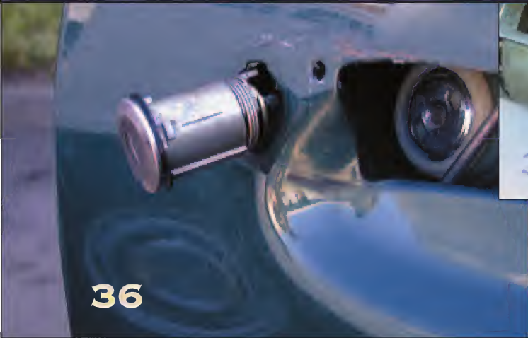
Remove the horseshoe clip and slide the lock out.
