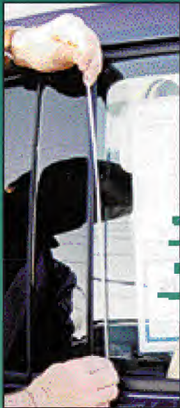
4. Once you have located the linkage, pull up with the tool to unlock the car.
