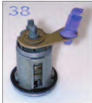
To remove the plug, remove the "C" clip on the rear of the lock.
