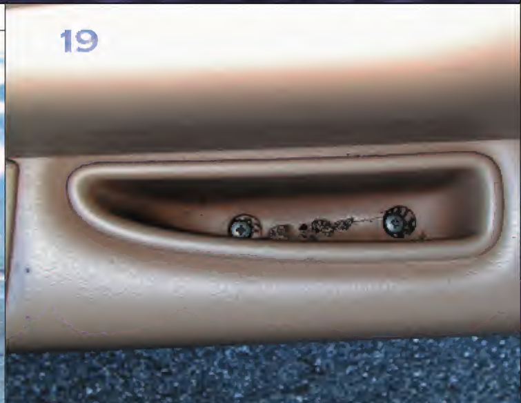
Inside the door pull cavity is 2 screws that must be removed.
