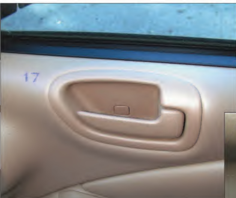
First remove the small trim cover that conceals the screw for the inside door release handle.
