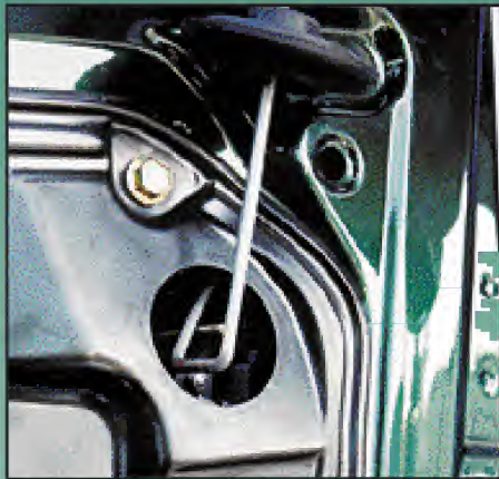
5. The tip of the tool in place to lift the linkage.
