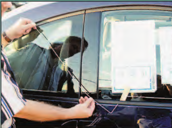
3. Insert the long end of the tool just to the rear of the inside lock button.
