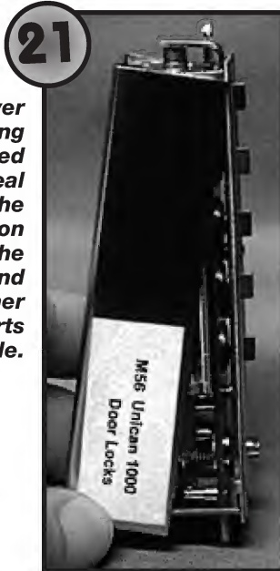
With the cover removed, the side view reveals five gears and the five toes of the unlocking slide.
