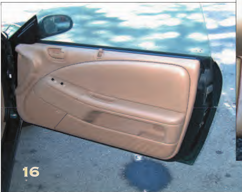
A view of the inside door panel that must be removed to access the door lock cylinder.
