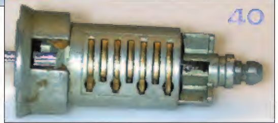
The door cylinder plug contains 7 tumblers in positions 2 through 8.
