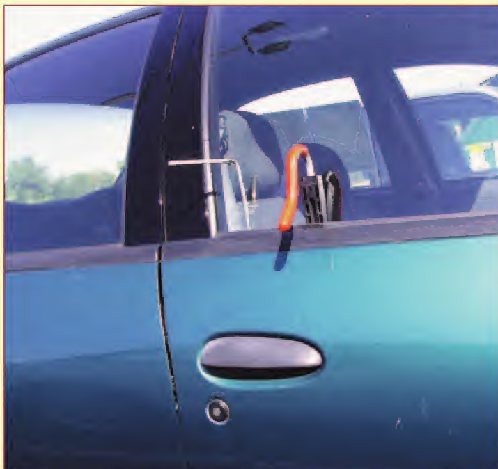
1. The door wedged and the correct working position of the down hook opening tool.
