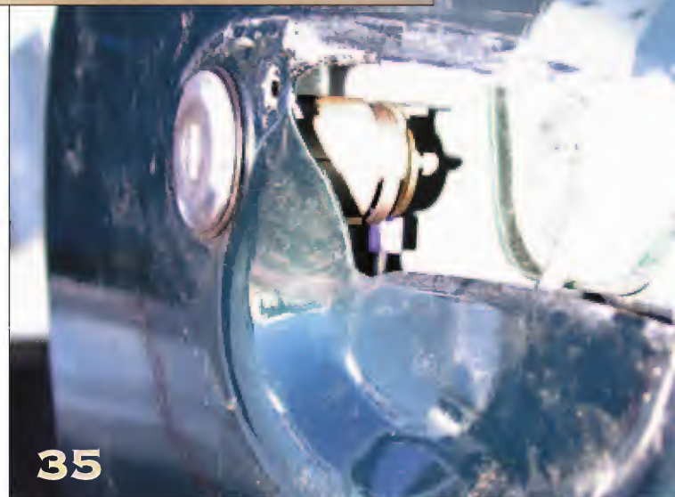
The lock cylinder linkage rod can now be disconnected.
