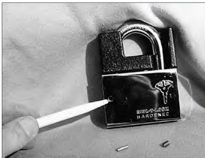
7. To rekey these locks, first remove the Allen screw and steel pin from the face of the lock.
