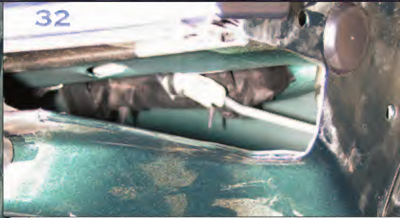
Disconnect the outside handle linkage rod. This view is from the top of the door looking down.
