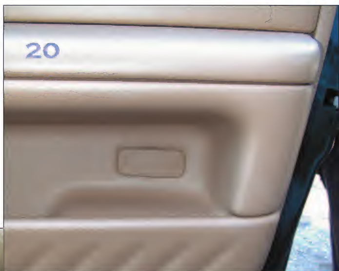
Inside the door pull cavity is 2 screws that must be removed.
