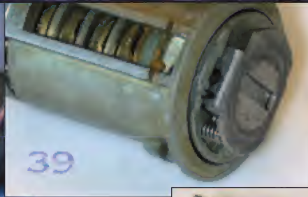
The door cylinder plug contains 7 tumblers in positions 2 through 8.
