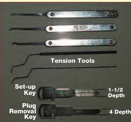
7. The assortment of tools, which I have found most effective for picking this lock.
