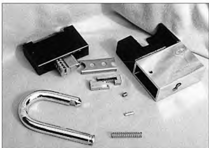
9. You can change the cam on the back of the plug to either a key retaining or a non key retaining function.
