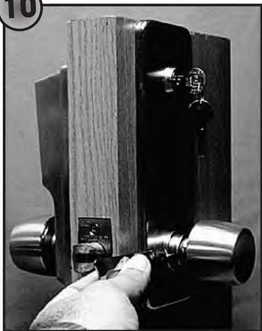
13 The spanner wrench is pointing toward the combination change sleeve.
