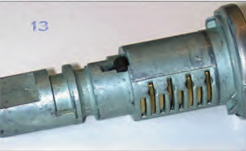
There is a very small buzzer actuator mounted in the plug. If this actuator is not there the car will not start.
