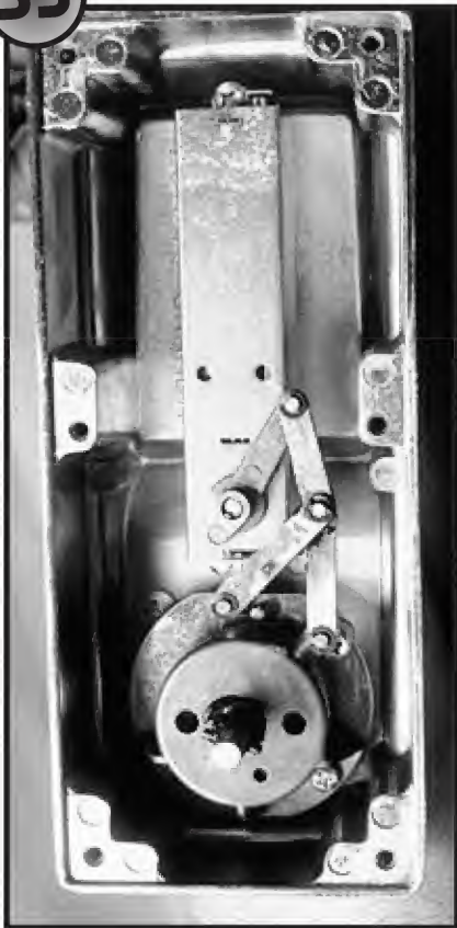
35 The knob rotation both opens the lock and sets the combination at the same time.
