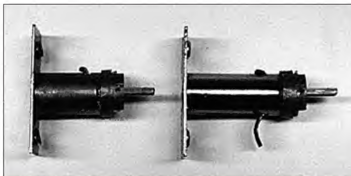
6. A recess must be made to accommodate a "multiplying lever" which allows the bolt to achieve a full 1" throw.
