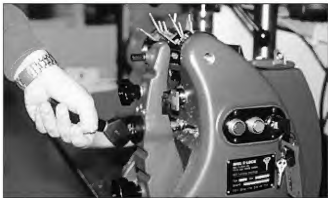
14. Milling exterior dimples on the key blank is achieved by means of an eccentric lever and round knob.
