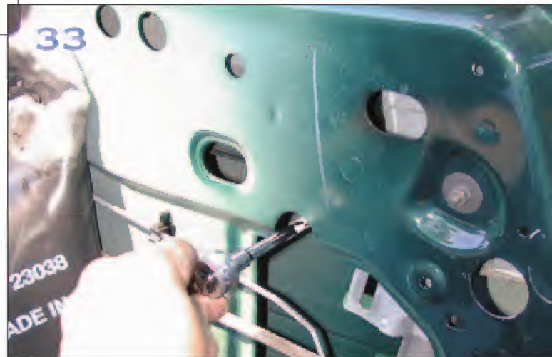
Raise the window back up to get to the forward handle 10mm nut.
