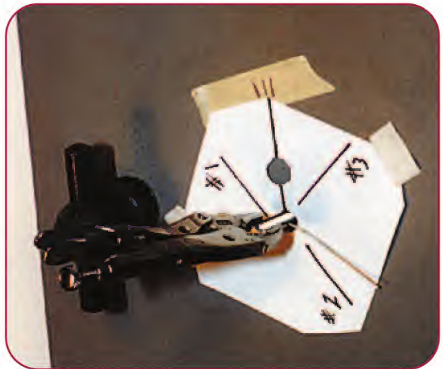
2. Just as you did with a transferring ring, move the hole reference line to the drop-in location of the lock.
