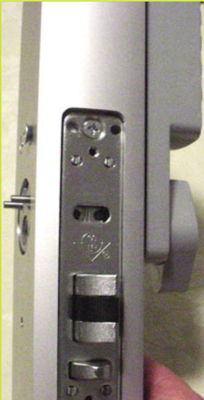
7. Two mounting screws have been inserted.
