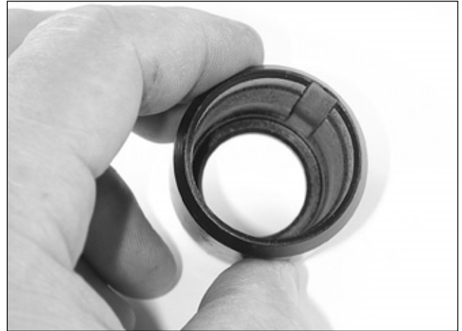
8. Looking on the inside of the security cup you see the cutout for the cylinders active retainer.
