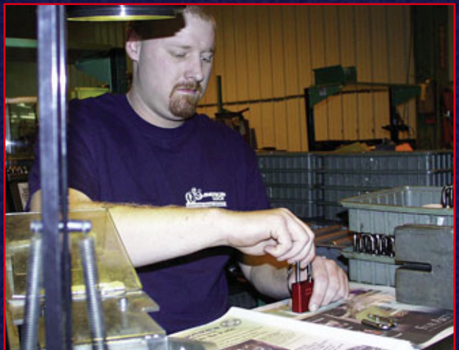
6. William Gillette demonstrates how each hardened shackle is individually fit to the machined lock body.
