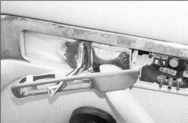
36. The next trim plate to remove is for the inside handle release. It won't remove entirely until the last armrest bolt is unscrewed.
