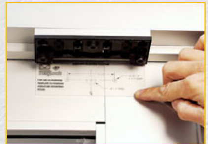
8. Holding the marking template mark the required three holes.
