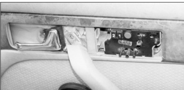
38. Now that the trim plate has been removed you can see the actual seat control module.
