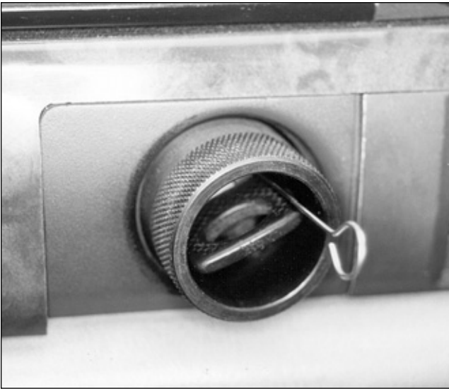
4. The black security cup can be difficult to unscrew because it doesn't get much use. I am using a gripping tool made to aid in the unscrewing of this security cup. The dash trim also gets in your way.
