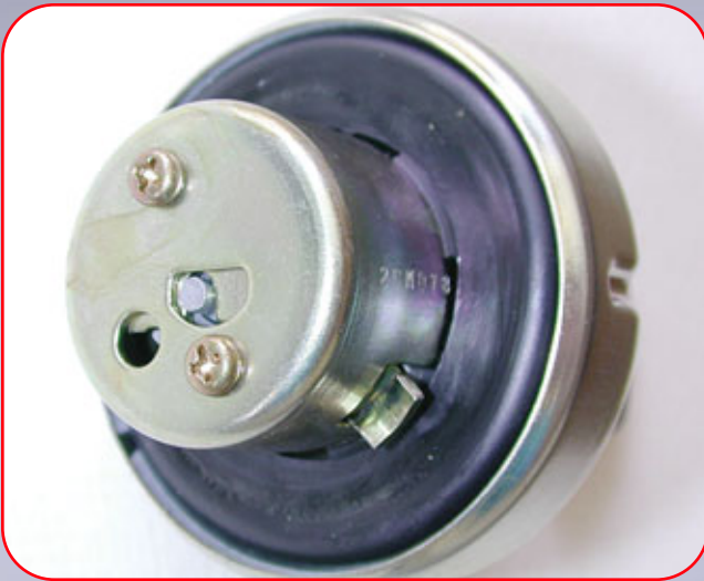
7 The code is located on the side of the gas lock housing.
