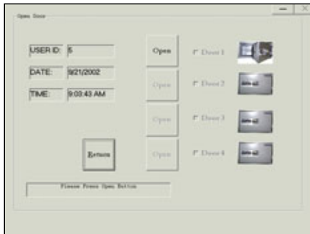
4. The “open door” option allows a user to open one of up to four safe doors.
