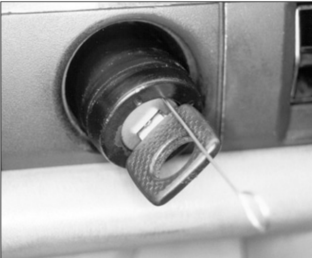
5. When the security cup is unscrewed you can remove the lock cylinder and security cup together.
