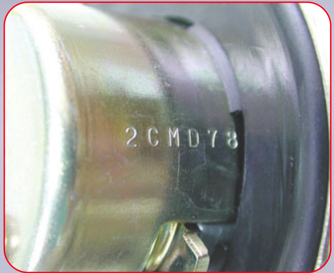
8 The code is the last three characters so in this case the code is D78.
