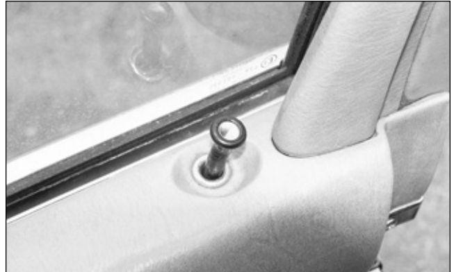
40. This model has the old style door lock button that will unscrew to remove it.
