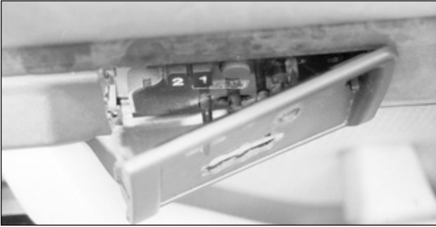
35. You will now be able to remove the seat control trim faceplate.
