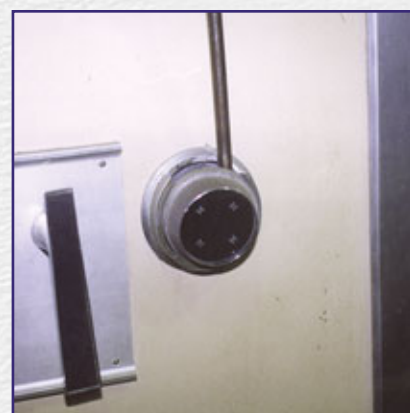
3. Easy dial removal with sharpened screwdriver and hammer.
