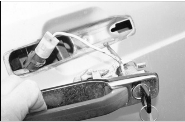
23. This model has a factory alarm system. The white alarm wire is attached to the lock cylinder in the handle.
