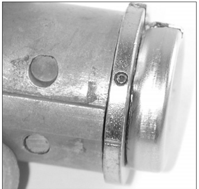
9. The silver hardened steel facecap for the cylinder plug is held in place by a single roll pin.
