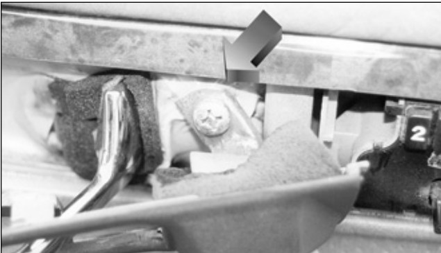
37. Under the inside handle release trim plate will be the armrest bolt. The bolt will need to be removed. You can always tell if someone has been there before you because there is a piece of foam that sits over the armrest bolt from the factory. If the foam is missing, then most likely someone else has had that door apart before.
