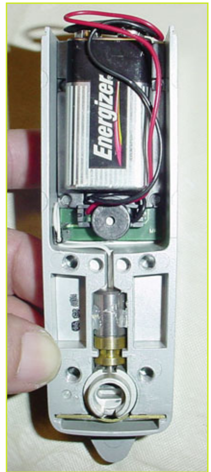
13. Inside the GardLok with the weather seal removed.
