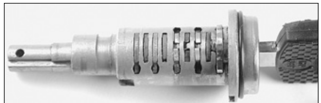
59. The door lock cylinder plug contains 11 tumblers. There are five solid tumblers and six split tumblers.
