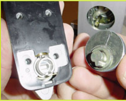
4. The disk that will interact with the lock.
