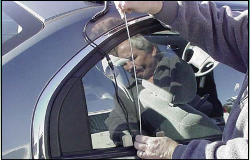
4. Once you have a firm grip on the linkage rod, lever the linkage forward in order to unlock the door.
