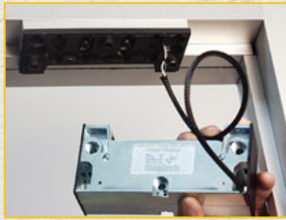
10. Thread the wiring harness through the mounting and filler plates.
