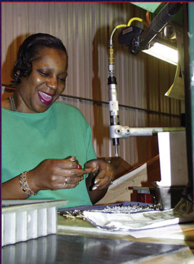
7. Corrie Brown assembling keyed cylinders into aluminum body lockout padlocks.
