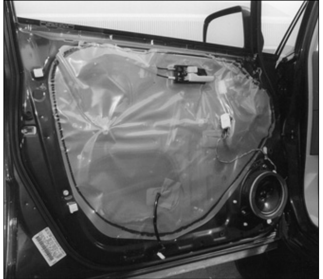
18. Once you have removed the door panel, you will see the plastic door liner.
