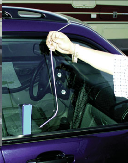
2. Inserting a wedge and opening tool is no problem.
