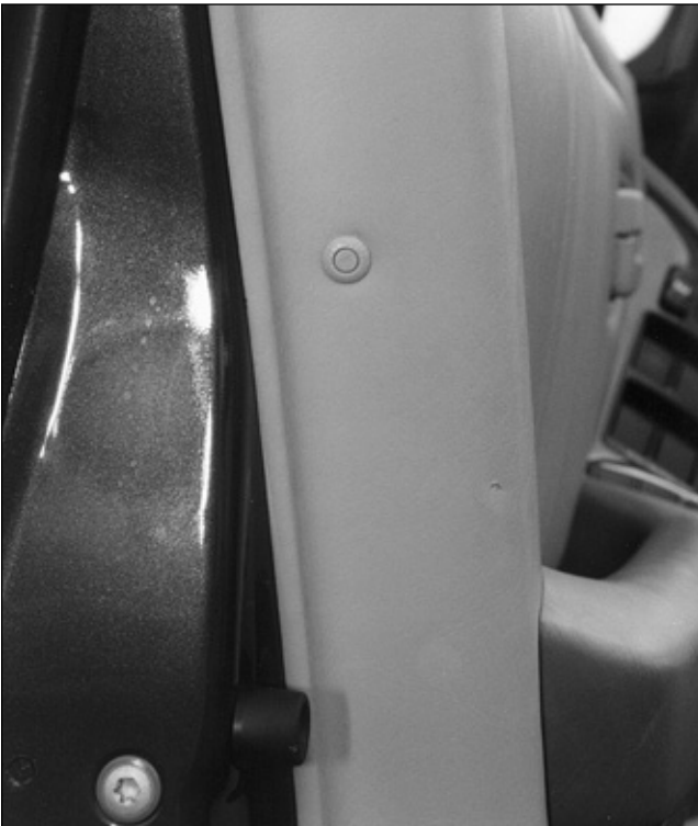
7. On the rear edge of the panel are 2 plastic fasteners. To remove these fasteners, push into the center of the fastener about a quarter inch. Do not push it all the way through. Once the center is pushed in, the whole fastener can be pulled off the panel.
