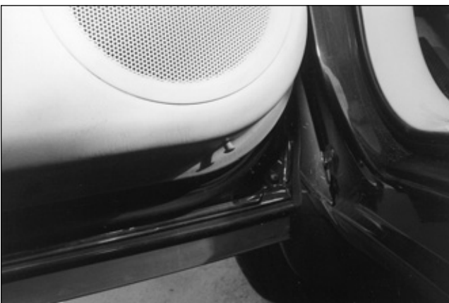
9. There are also Phillips head screws that must be removed.
