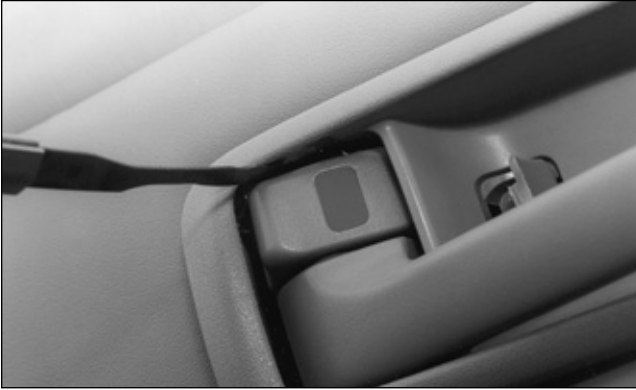
5. The rear portion of the trim snaps onto 2 posts, upper and lower, that must be removed.
