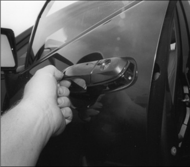
23. Disconnect the linkage rods and tilt the handle out and remove.
