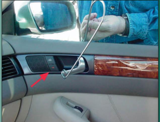
10. On the Audi vehicles you will have to pull the handle twice to unlock the door.
