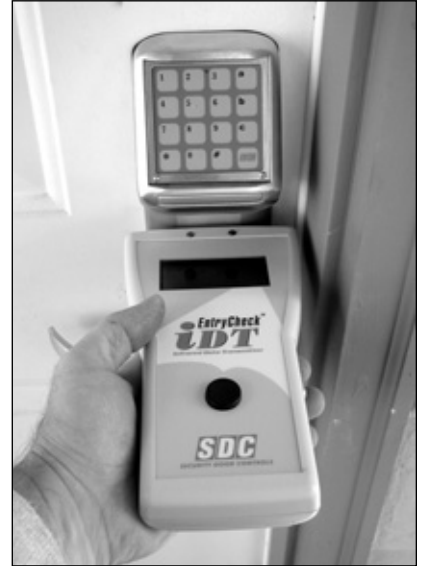
14. Programming the lock can be done with an Infrared handheld device or simply by pressing buttons on the keypad.
