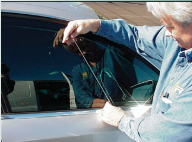
7. Always remove the wedges before pulling the tool up.
