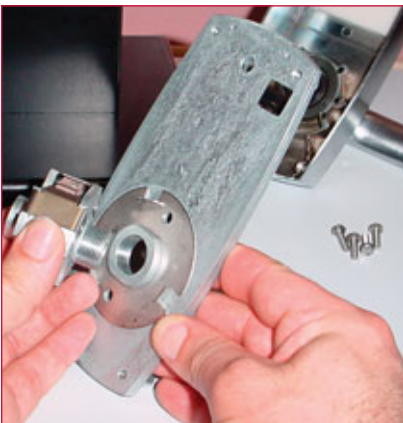
4. The external threads of the retractor unit ready for attachment.
