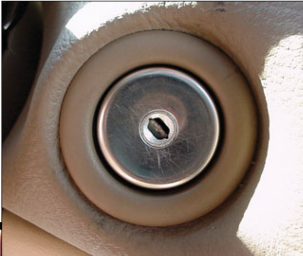
5. The ignition lock on the S Type is part of the dash assembly.
