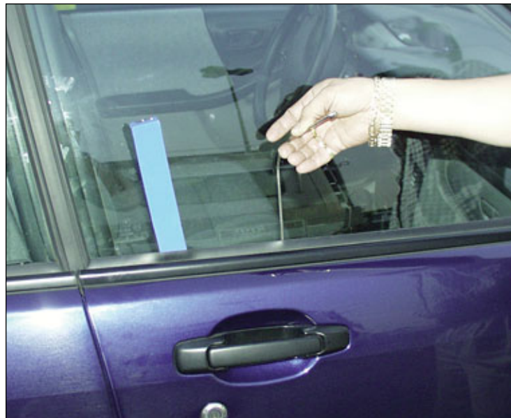
3. Insert the 47 tool about half way.
