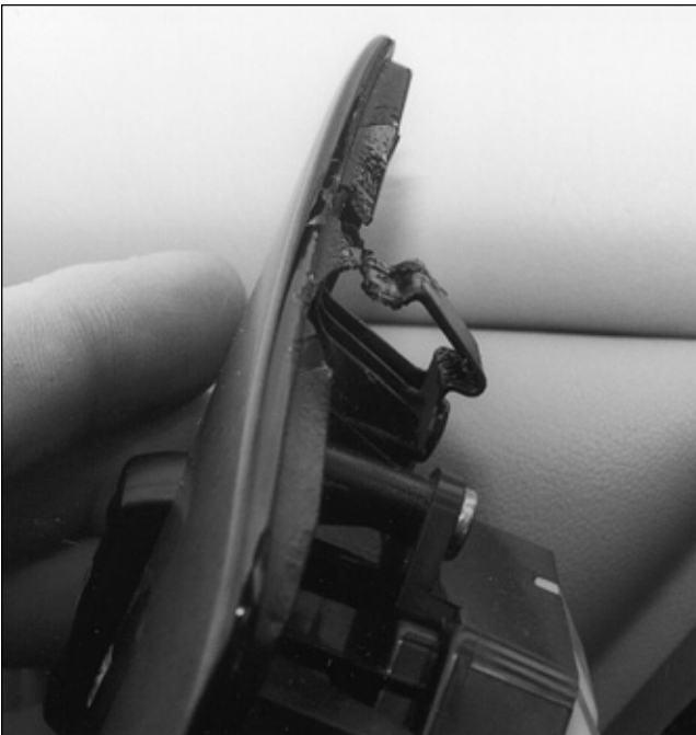
13. Here is a look at the front door control trim fastener. If you try and remove the rear section first, the plastic lever will snap off and break.
