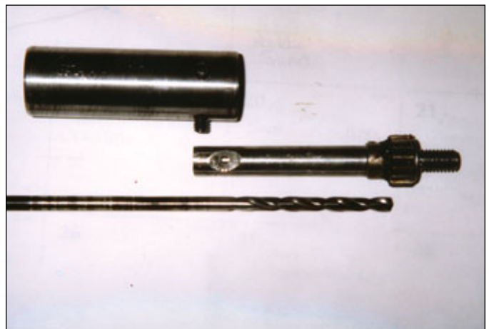
2. The drill guide is then drilled and tapped for two setscrews.
