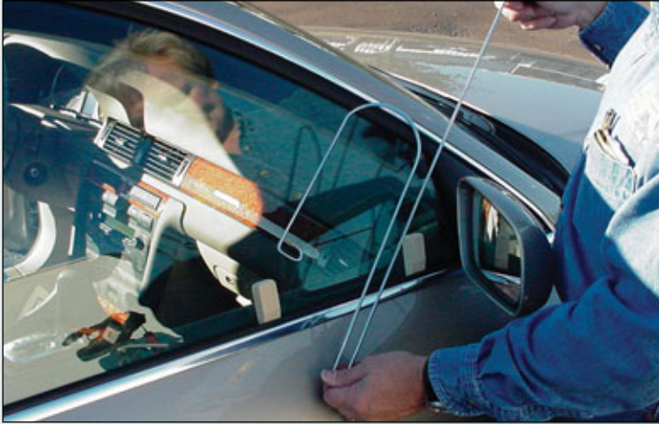
5. The TT-1015 tool is inserted near the front of the door.
