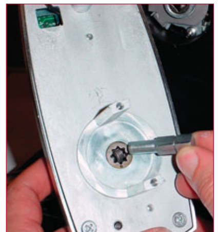
9. An Allen head screw is accessible inside the spindle hole.
