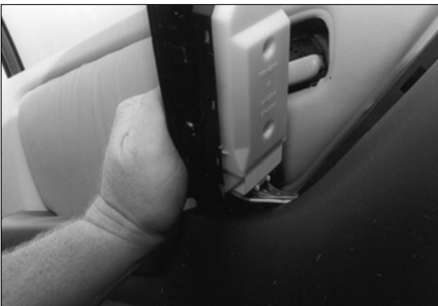
14. You must disconnect the electronics and then completely remove the door control unit.
