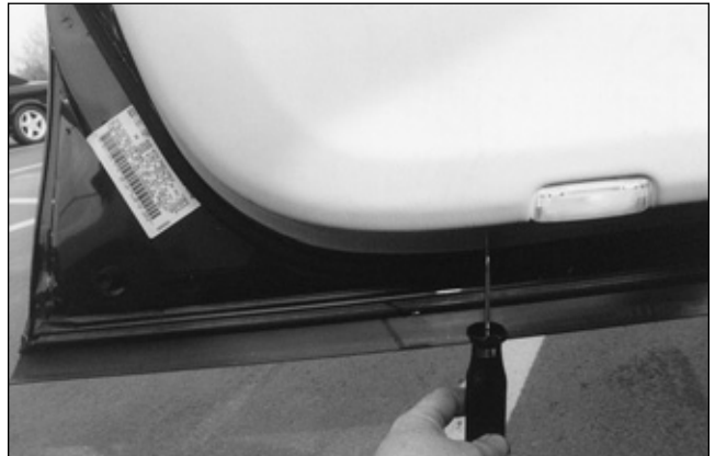
8. On the bottom of the door panel are more fasteners that must be removed.
