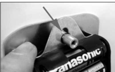
7. The battery holder slides over the stud at the top of the interior backplate.
