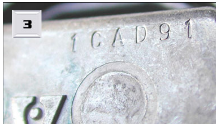
The code is stamped on the bottom of the gas cap in very small characters. The last three characters are the code, so in this case the code is D91.
