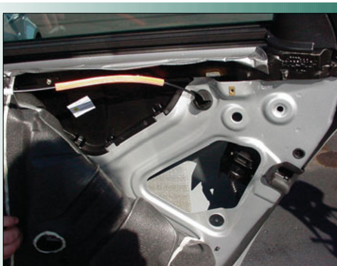
4. The interior of the door showing the bicycle-style cable.
