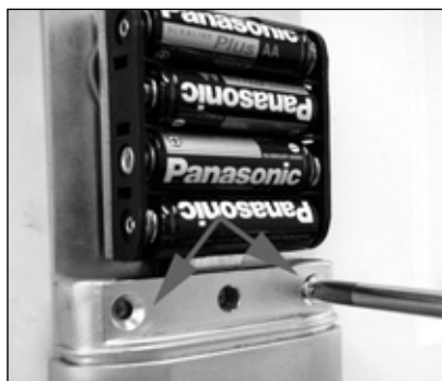
9. The lower cover is slid into place and attached with two brass screws located at the top and a finished screw that is located at the bottom of the assembly.
