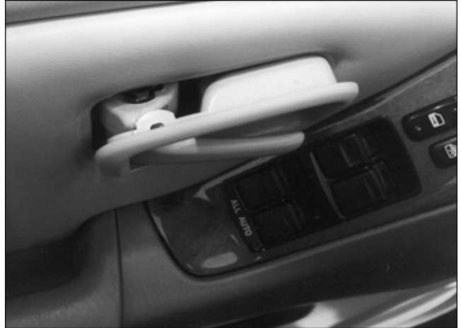
6. Use a small screwdriver or other object that will slide in place and lift the trim off the upper post and then do the same to the lower post.
