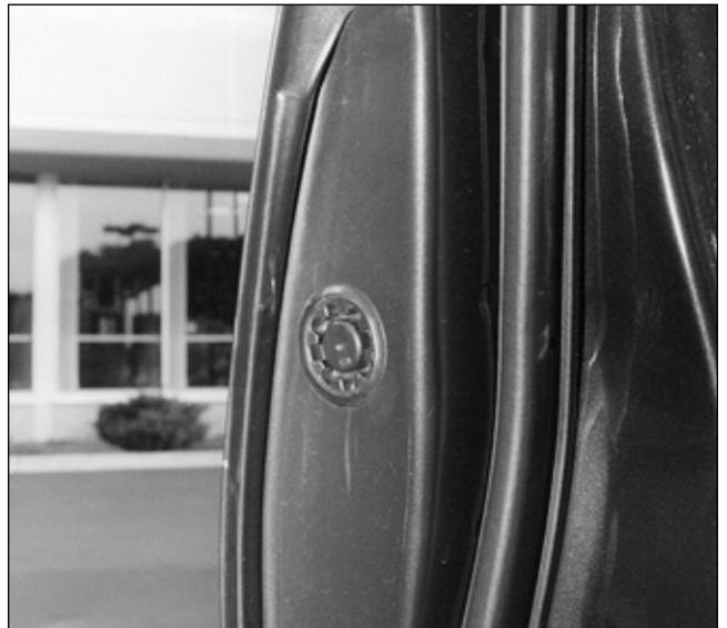
20. Remove the plug and then you can get a socket wrench in there to unscrew the 10mm bolt holding the rear section of the handle.
