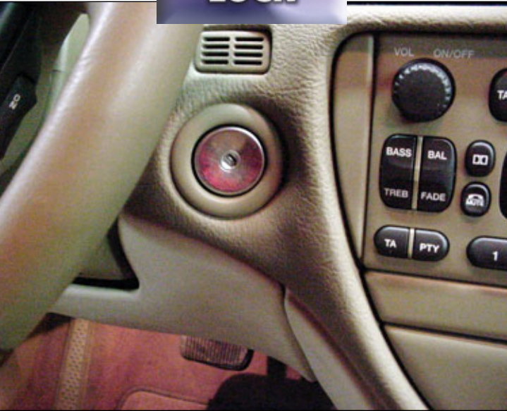
5. The ignition lock on the S Type is part of the dash assembly.
