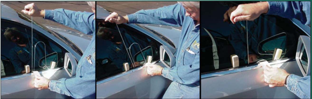
6. A plastic card is used to prevent rolling the lower layers of the weather-stripping.
