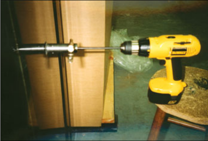
3. The drill guide installed.
