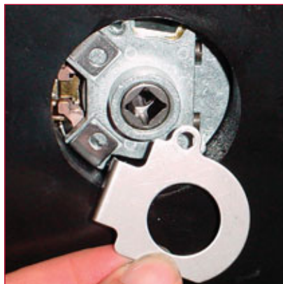
7. A metal plate will act to block attempted manipulation.
