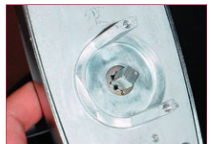
10. Either a plug or I-Core must be installed.
