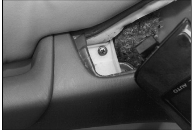
15. Under the rear section of the door control unit housing is a Phillips head screw that must be removed.
