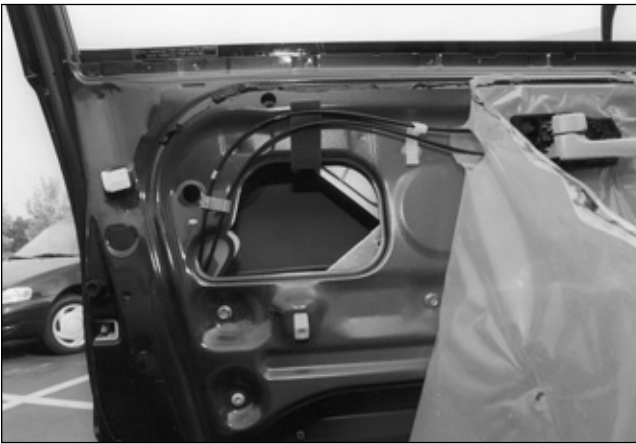
19. The liner is actually there for a reason and not just to annoy us and get in our way. Take care and gently pull the liner out the way without ripping it.
