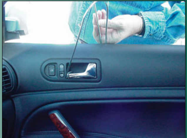
8. Use the looped end of the tool to pull the door handle before pulling the tool up.
