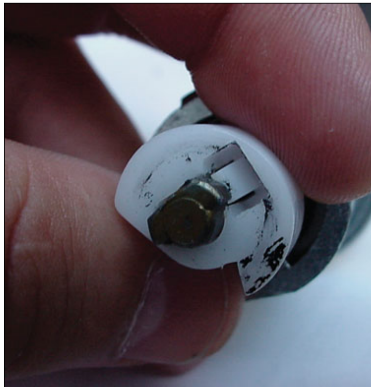
13. Turning the lock over, a large plastic cam is present.
