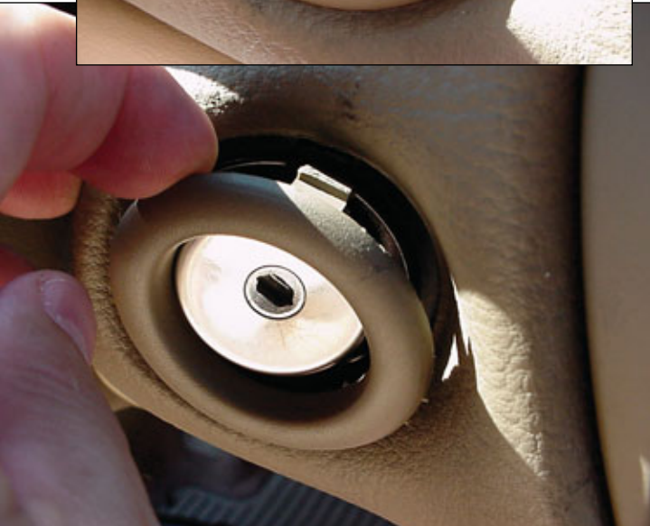
6. Despite its location, in most instances, the lock can be removed without dash disassembly. Start by removing the plastic trim ring from around the lock.
