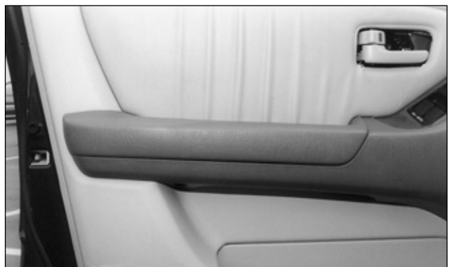
10. The inside door armrest has a Phillips head screw that must be removed.
