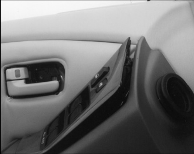
12. The next item to remove is the door controls. Lift it up from the front and work your way to the rear.
