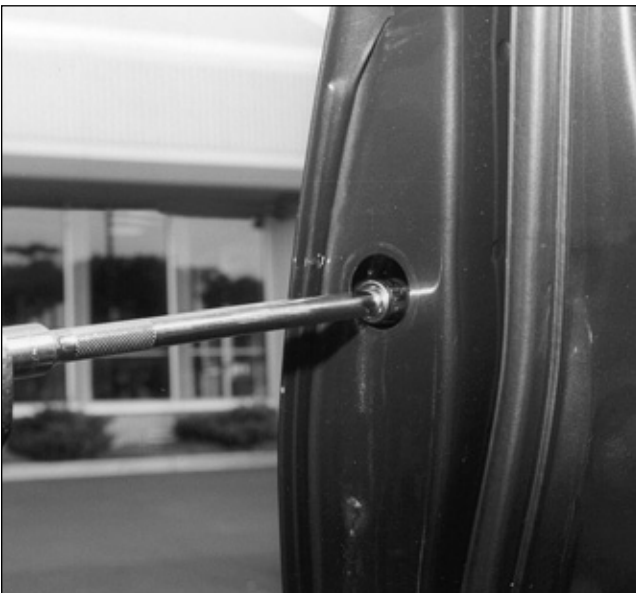
21. On the edge of the door is a plastic access plug.
