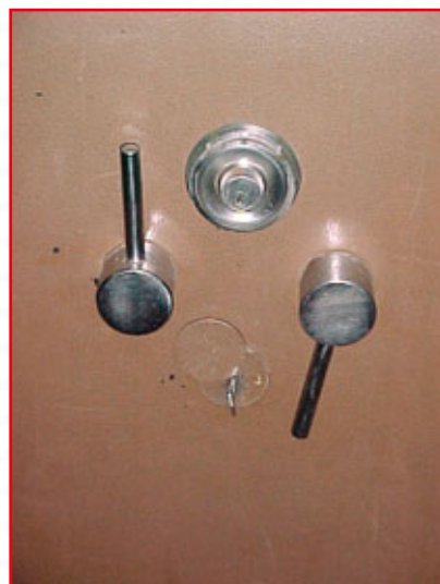
3. One handle operates the opening and bottom bolts. The other operates the top and hinge side boltwork.
