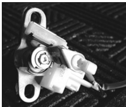
25. The tailpiece is held on with a "C" clip.
