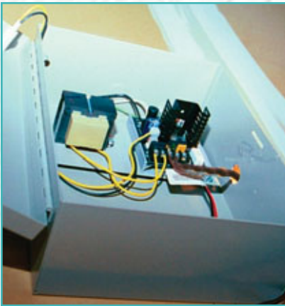
23. In this pizza delivery store installation, I used a SEBPS-24-2A battery backup unit. I ran my normal AC power source to this box (there are no batteries in this one, yet) and then run to the CPU board off the DC leg in the Power Supply. The batteries are there to provide operating power in the event of a power failure since this installation is a fail-safe install. That is, when the power goes off, the locks automatically release. Since that could pose a security risk during operating hours, I used the extra power supply.
