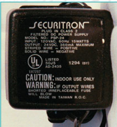
11. The model PSP-24 transformer for the DK-26 and the MAG lock.
