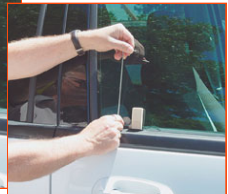
3. Lower the tool until it contacts the horizontal frame member inside the door.
