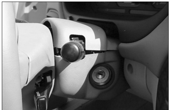
9. The column shroud halves can now be separated and removed.
