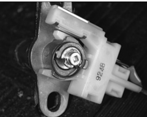
26. The rear of the lock cylinder has an electronic connector on the backside. You can leave it on or remove it if it gets in your way.
