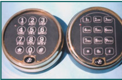
6. The two battery keypad on left and the newer single battery keypad on right. Both use 9-volt alkaline batteries.
