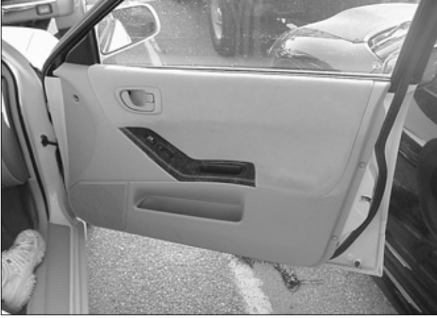
14. Although it is not necessary to remove the entire door handle, the door handle does have to be removed to access the door lock.
