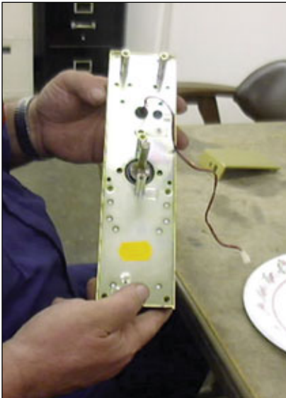
28. Install back cover carefully. Feed wire through the case to keep from binding or pinching, or pulling out rubber gasket.
