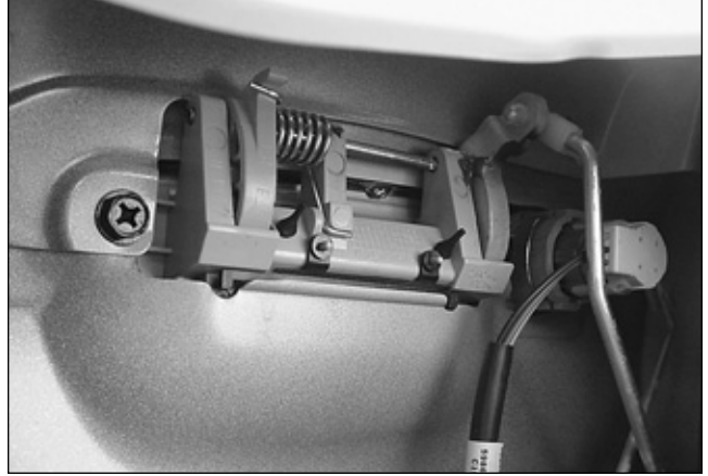
22. The lock is easily accessed. Removing the lock rod makes removal easier.
