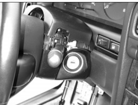
12. The upper section of the plastic shroud will unsnap after the screws are removed.
