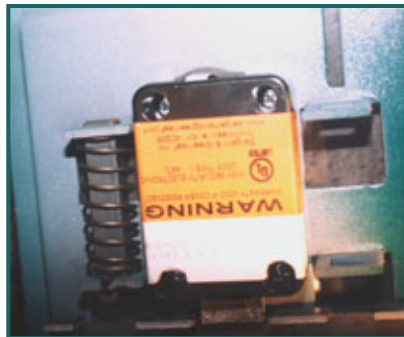
5. New 6123 lock mounted on safe.
