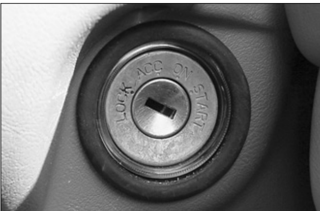
6. The Galant ignition lock is typical of all Mitsubishi push-button retained locks.
