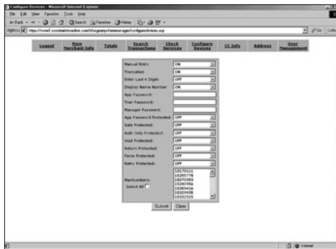
G. The RIM devices can be configured wirelessly. If a change has to be made with a device, it can be done almost instantly.
