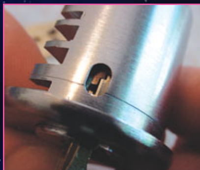
18. The change key side bitting engages the change step to position the slider.
