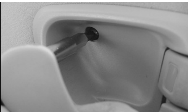
16. Remove the door handle mounting screw....
