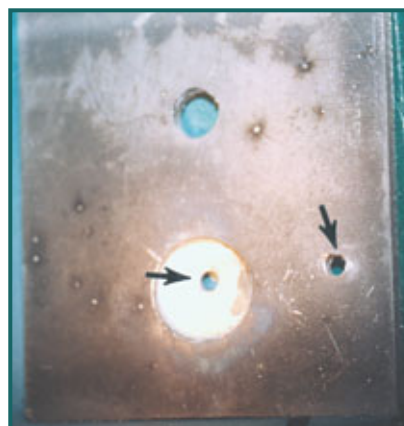
2. Diabolical Diamond Dusted Disk of Death (D5) on large hardplate. Arrows point to holes I drilled for bolt and relocker.
