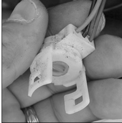
26. The two tabs on this switch hold it to the lock. Carefully pry these tabs up to remove it from the lock.
