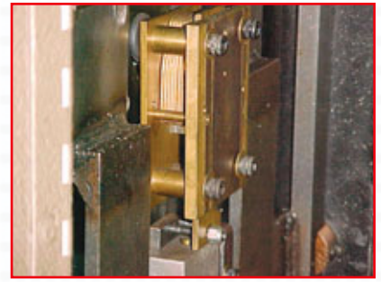
10. The DeBuse key lock mounted Vertical Down (VD).
