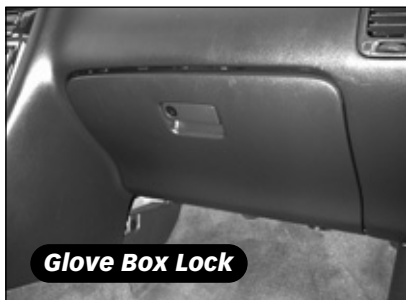
30. The glove box door has a locking cylinder in it.
