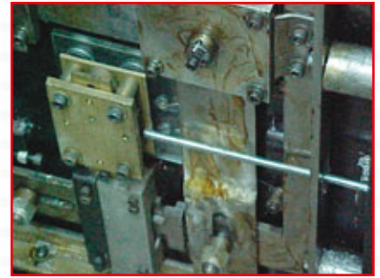
11. The punch used to knock off the stump.
