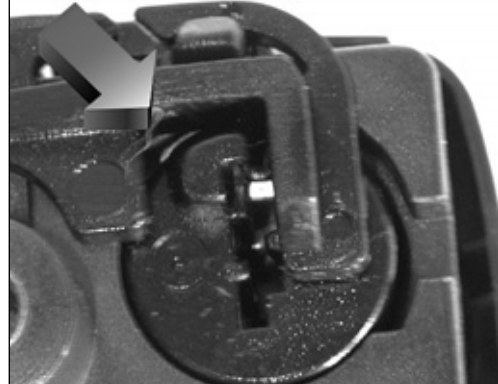
32. There is a small opening to reach in with a pick and push down the retaining tumbler to slide out the cylinder plug.
