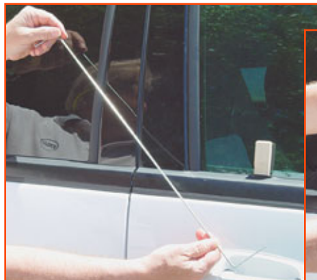
2. The long end of the TT-1000 tool is inserted as far to the rear as possible.
