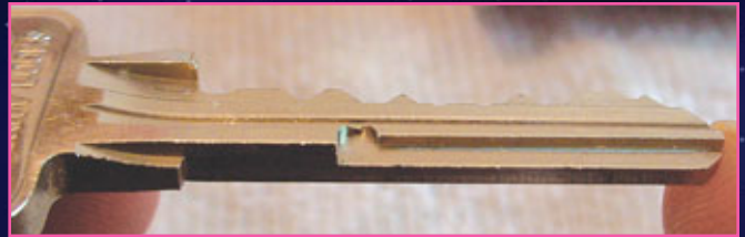
15. A master key has the change key side bittings milled back.
