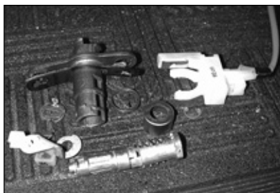
28. The trunk lock disassembled.
