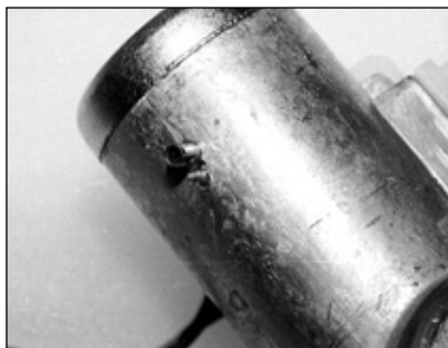
17. Drill into the lock housing approx 1/4" directly next to the roll pin with a 7/16" or smaller drill bit. Make sure you are slightly drilling right up against the roll pin. This will ensure the roll pin coming out easily.
