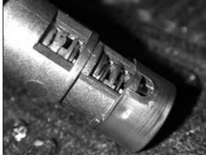
27. The face cap is easily removed and must be re-used.
