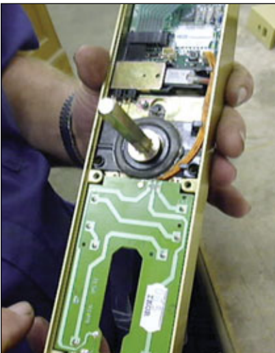
5. Lock back plate removed showing wiring and battery circuit board. Note wire path and plug.
