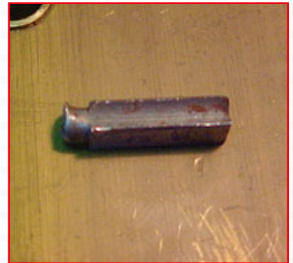
12. The stump is in good enough condition to be reinstalled and reused.
