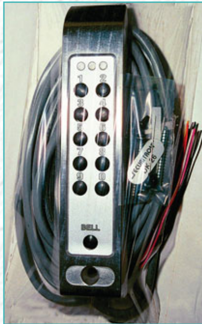
18. The DK-26, weatherproof touchpad with its 16-foot, 10 conductor, color-coded cable. This cable wires into the CPU board. Simply match the color-coded wire to the color designated at the terminals, as shown in photograph 14.
