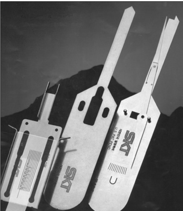
5. Using the SKT Wafer Reader is another lock reading device designed specifically for fast and easy key generation.
