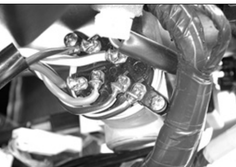
15. There are 2 screws that hold the electrical connector to the rear of the lock housing.
