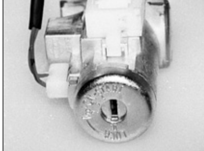
16. The ignition lock face cap is secured with 2 opposing solid roll pins that must be removed to release the ignition lock cylinder plug.
