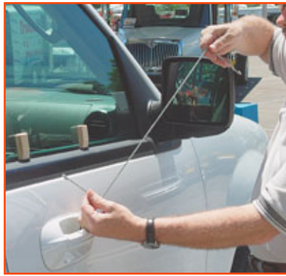
6. The TT-1017 tool is inserted at the rear of the door.
