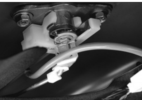
23. There are two 10mm bolts that secure the trunk lock cylinder.
