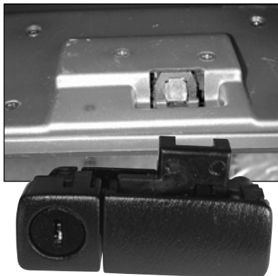
31. The lock handle assembly can be easily removed by taking out the 2 screws that secure it to the glove box door.
