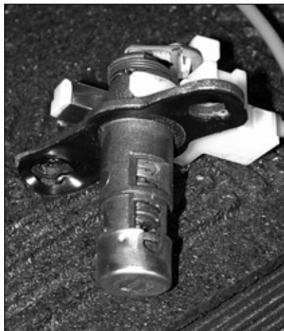
24. The trunk lock cylinder removed from the car.
