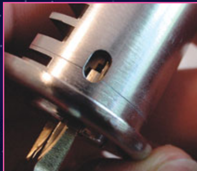
16. The master key side bitting engages the master step to position the slider.
