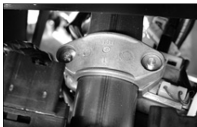
14. The ignition lock assembly is secured with 2 shear-head bolts. These are easy to remove by means of a couple different methods. One of the most common methods is to Dremel a groove in the head of the bolts and unscrews them. Another is to use a scratch Awl and by tapping on the outside edge of the bolt counter-clockwise. It will also loosen the bolt.
