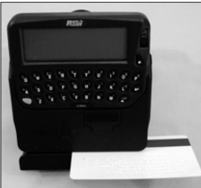
3. Swiping the credit card and punching a few buttons will complete a point of sale (POS) transaction.
