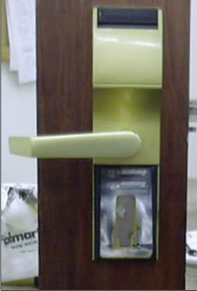
3. Battery cover removed. Uses torx tip driver #15 (screw on bottom of case on the outside). Access to batteries if lock is dead, requires four AA batteries. Also jack plug on bottom for portable module.
