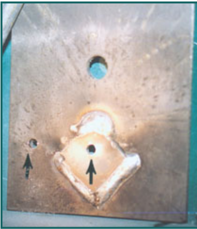
3. Back side of hardplate showing how the D5 was welded onto the hardplate over the disk hole.
