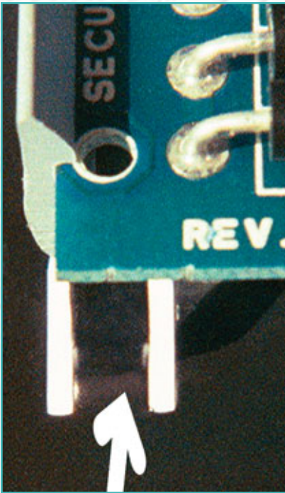
17. The white arrow points to the tab (there are four) that slips over the circuit board to hold the board in place in the can, or housing, which attaches to the wall or ceiling.
