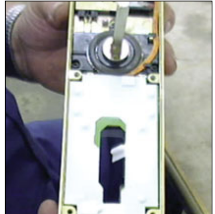
26. Install shield over circuit board. This protects the circuit board from the back case cover.
