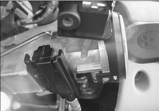
11. Insert a mechanical key or pick the lock to the ON or RUN position and depress the lock's retainer.
