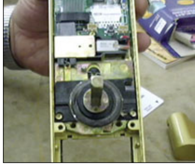
6. Lock back plate removed showing cover and spindle shaft rubber gasket (2 torx screws are under gasket to remove cover). Gasket has self-stick on one side; set aside to reuse. It is not in the replacement parts. You can see the lever spring from this point in disassembly.
