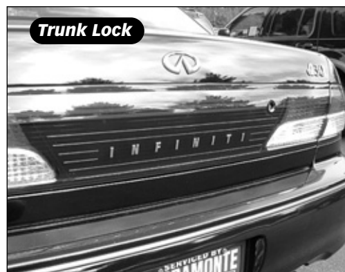
21. The trunk lock cylinder is easy to remove. It is not necessary to remove the taillight assembly.
