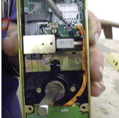
23. Lock reset button. Don't touch it. This will reset the lock and you will need to reprogram the lock with the desktop and portable hand held module to get it working again. It erases the memory of the lock so the cards will not work. Will not recognize the master or the room card keys. Does not reset any faults as far as I have been able to determine.
