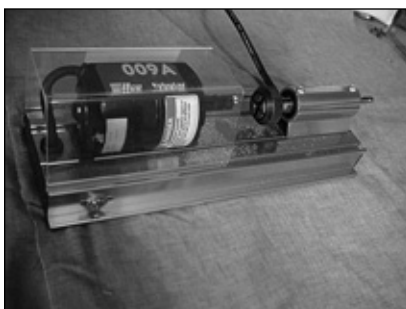
2. Ilco 009A Tubular key machine.
