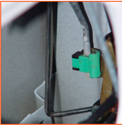
5. The tip of the TT-1000 in position lifting the bellcrank to unlock the door.
