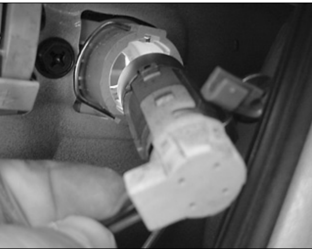
24. The lock is easily slid out of the handle.
