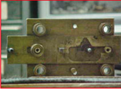
6. With all the levers removed you can see that stump is attached to the locking plate.
