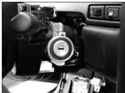
13. The lower section of the shroud can be removed.
