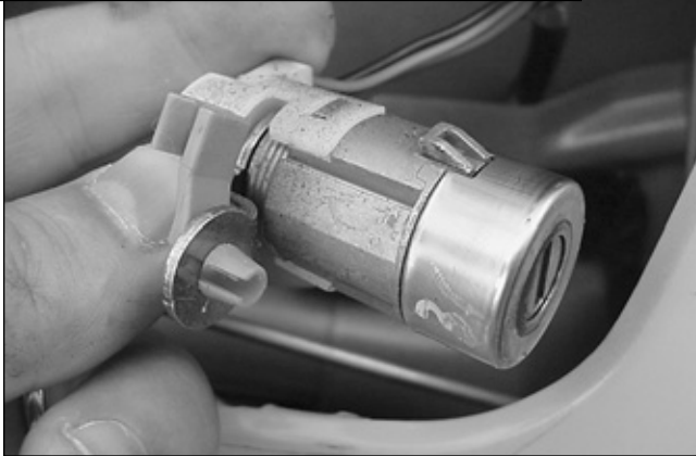
25. A micro switch is attached to the back of the lock, and must be removed before lock disassembly can be performed.
