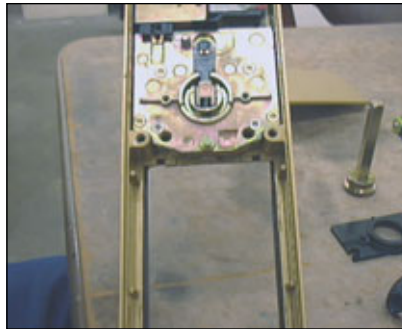
7. Drive gear, springs clutch and back plate. Note six torx screws (only 4 need to be removed). Note position of lever spring on post. If put in reversed it will not operate. When in locked position, driver pushes into clutch against the compression spring and keeps spindle from operating shaft. Be very careful of springs, they like to bounce out and hide in the hardest place to get to. The driver is made of plastic, the clutch is pot metal. Look very closely for wear and save all old parts to be reused in an emergency.
