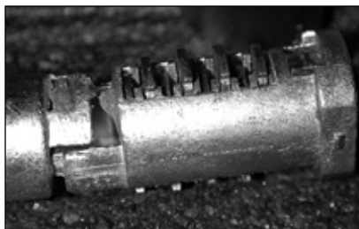
29. The trunk lock cylinder has all eight tumblers in it.
