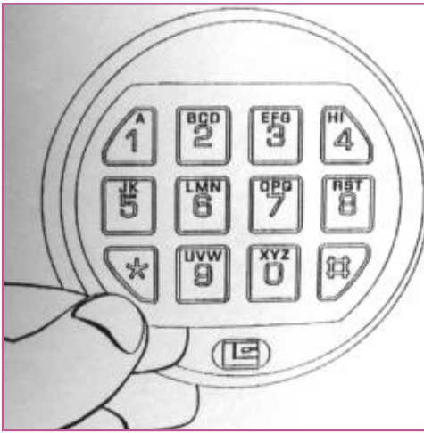
A. Peel the membrane keypad by lifting one of the bottom corners.
