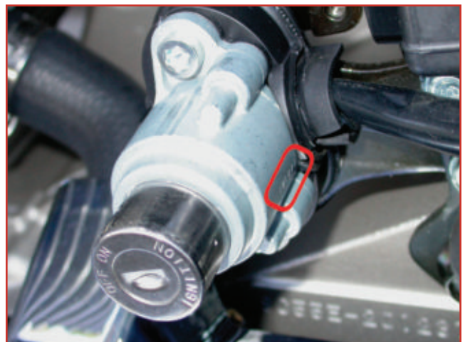
13. The code is located on the right side of the ignition lock. It is circled in the photo.
