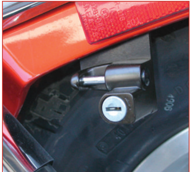
15. The helmet lock is located on the left side of the bike and to the rear of the shock absorber. You need to turn it 45-degrees counter-clockwise to unlock it.
