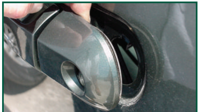
38. As stated earlier, the lock is not actually a part of the handle. Instead the lock is used to hold the handle to the outside of the door.
