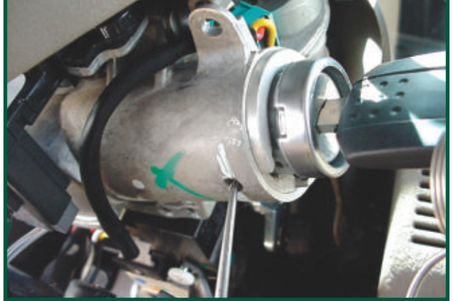
16. With the transceiver ring removed, the lock's retainer can be depressed for lock removal. Insert a key, drill or pick the lock to the ON or RUN position and depress the retainer.
