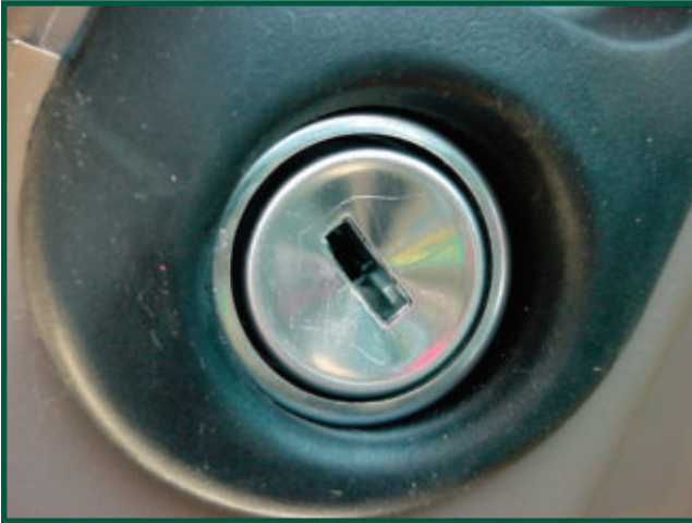
5. Originally, this ignition lock was introduced as the STRATTEC 706229 and included a sidebar. In September/October 2002, this design was changed to a non-sidebar version of the same lock, STRATTEC 707592.
