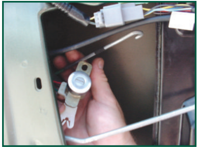
35. The lock is now free to be removed.
