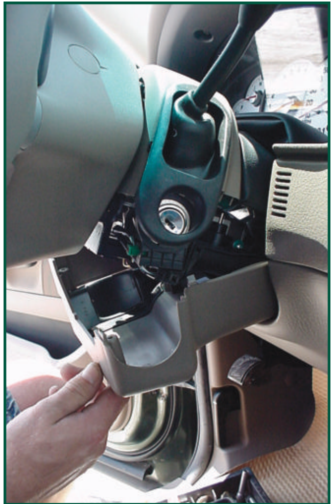
7. Remove the lower shroud and move aside the large rubber grommet or bezel surrounding the lock and the shift lever.
