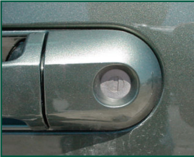
20. The door lock of the Mountaineer appears to part of the handle. However, handle removal is not required for removing and servicing the lock.
