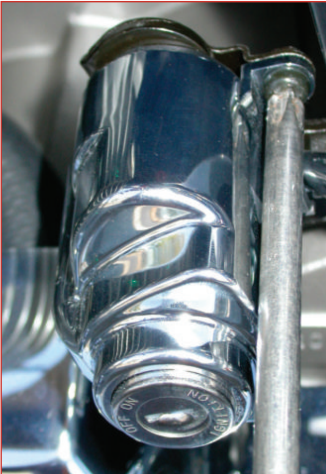
11. Remove the large Phillips screw that holds the ignition lock cover on. The ignition lock only has positions for OFF & ON.
