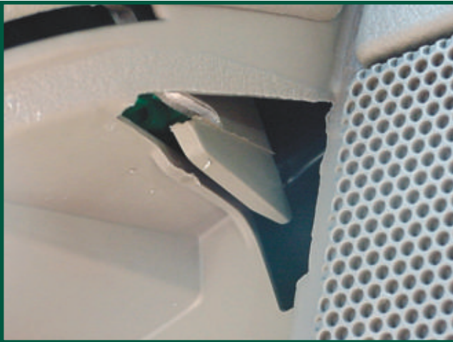
26. Be careful to release the small retaining tab that holds the panel in place.
