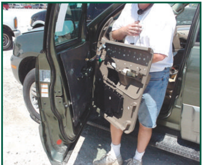
31. Large hooks on the panel hold it to the door. To avoid permanently damaging the panel, DO NOT try to pry the panel off of the door.
