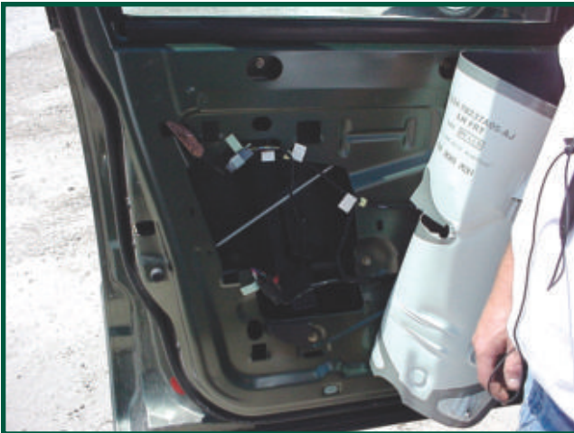
33. A vapor or environment barrier covers the inside of the door. To give us open access to the lock, carefully peel back the edge of the barrier, making sure not to rip or tear it.
