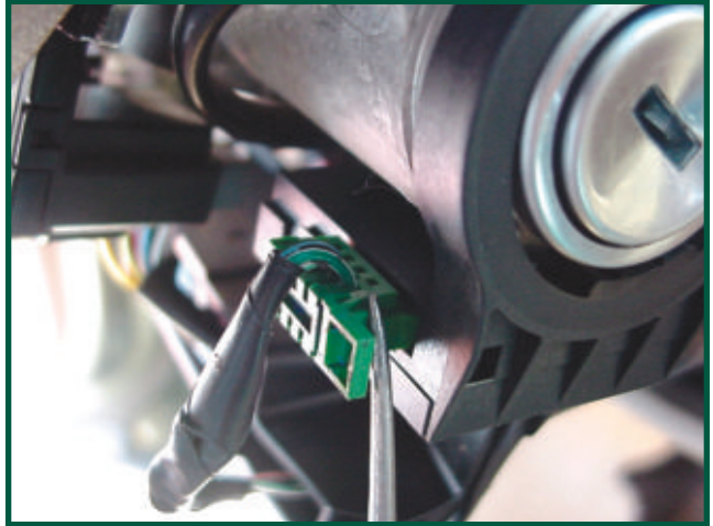
12. Using a small screwdriver, gently depress the locking tab of the transceiver connector.
