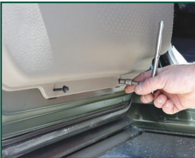
22. Three screws can be found along the bottom of the panel. Use a small socket to remove the screws.
