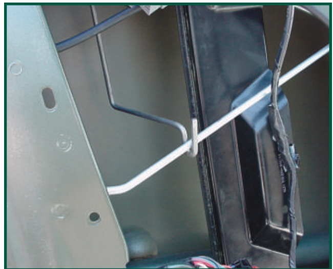
3. Grasp the interior lock rod and slide to unlock the door.
