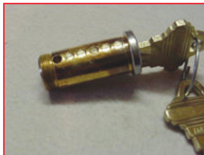
3. Pins at shear line.
