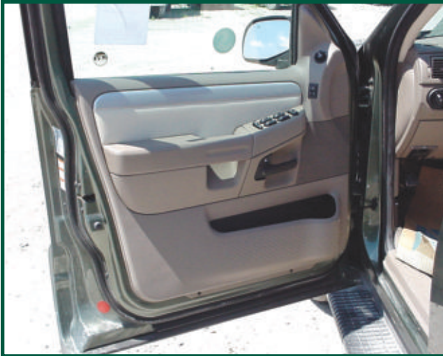
21. Begin door lock removal by first tearing down the door panel.
