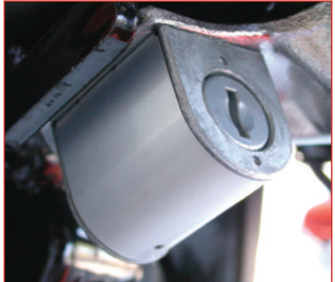
17. The steering lock is located on the right side near the front forks. You need to turn it 180-degrees clockwise to lock it. The steering has to be turned all the way to the left or right before the bolt will extend. It is secured by two large Phillips screws from the top, but the front-end assembly needs to be removed before you can gain access to them.
