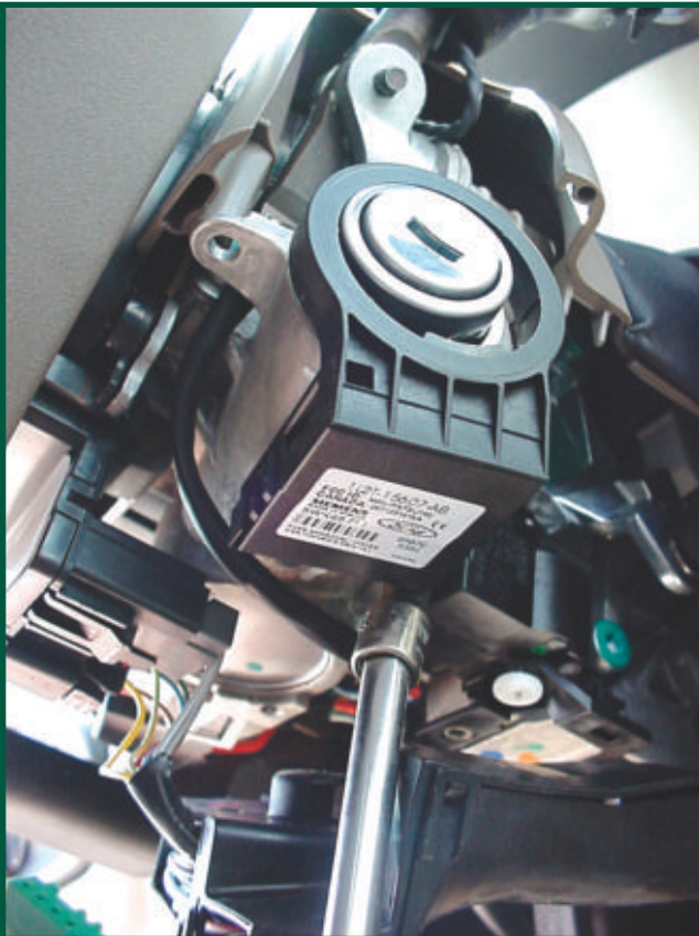
14. With the connector separated, locate and remove the one bolt fastening the transceiver ring to the column.
