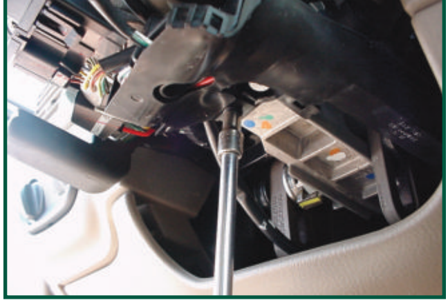
11. Remove the final bolt holding the harness to the column.
