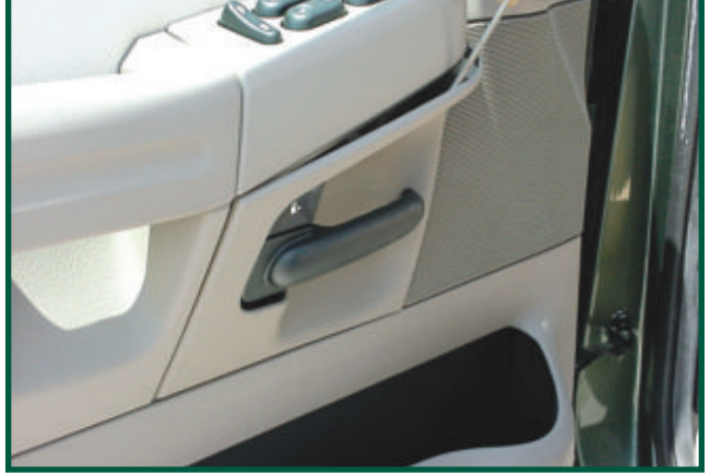
23. Using a trim and panel tool to separate the trim.
