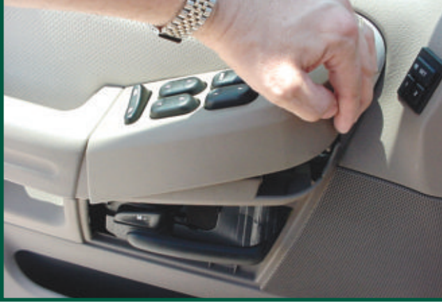
25. Next, grasp the top of the window switch panel on the armrest and lift.
