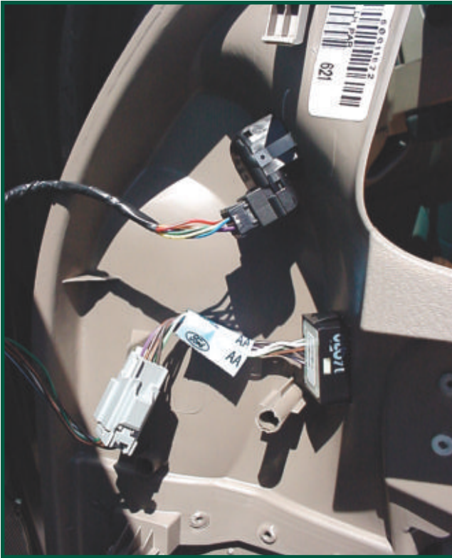
32. Once the panel has been separated from the door, disconnect the various connectors attached to the trim panel.
