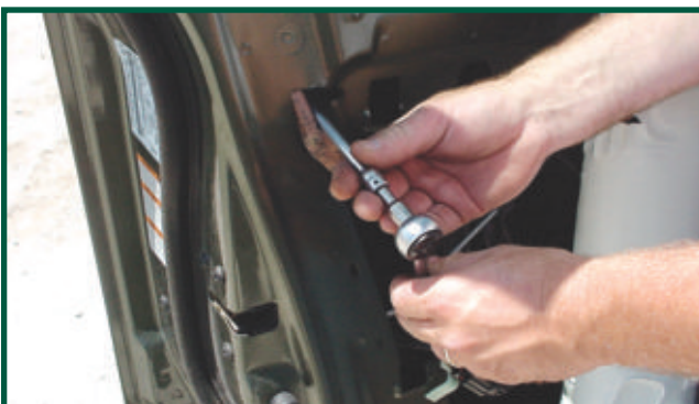
34. To complete lock removal, use a 12mm socket to remove the nut holding the lock in place.
