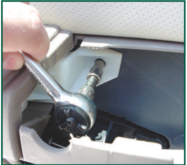
29. With the panel removed, a small bolt is visible. Use a socket to remove the bolt.
