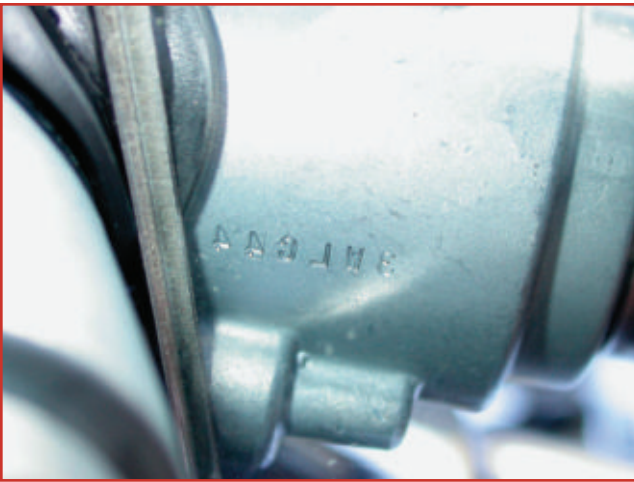
14. You can read the code without a mirror but it was the only way I could get a good photo of it. There are six characters but the code is the last three. It is in mirror language but you can see that the code is C44. The codes are sometimes stamped on the bottom of the lock and the mirror helps in those situations.
