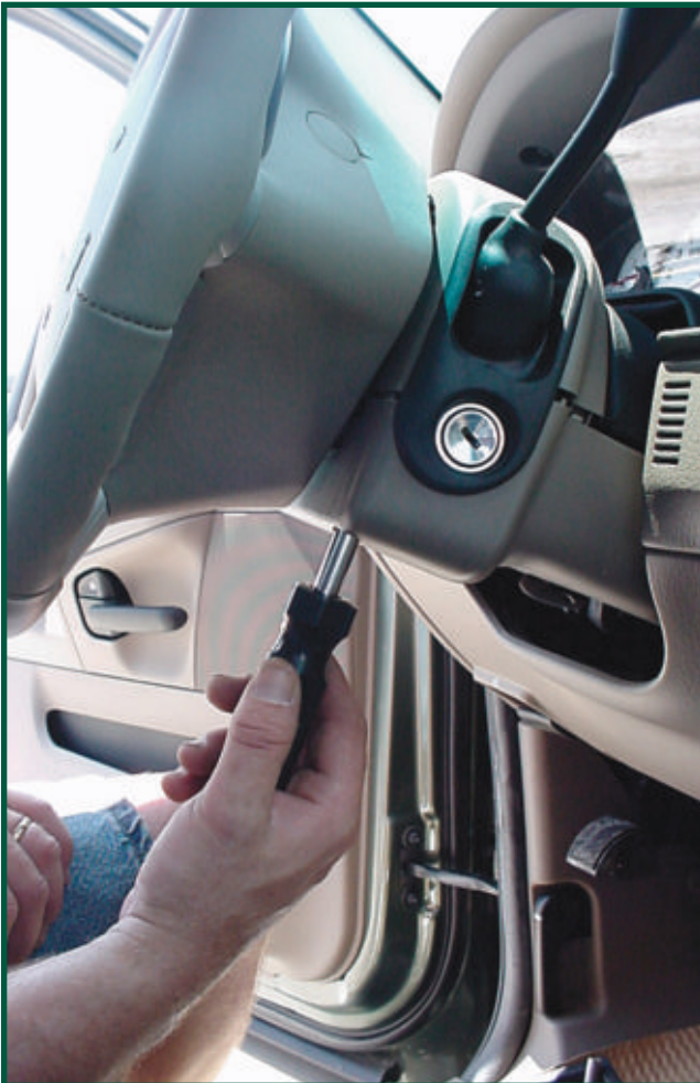
6. Removing this lock is a little more difficult than the locks used in previous year models. Gone is an access hole in the lower shroud, allowing access to the lock's retainer button. As such, it is necessary to first remove the lower shroud on this column to gain access to the lock's retainer. Use a standard Phillips head screwdriver to remove the lower shroud's mounting screws.
