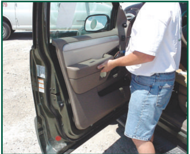
30. The door panel is now ready for removing. Grasp the panel and lift straight up.
