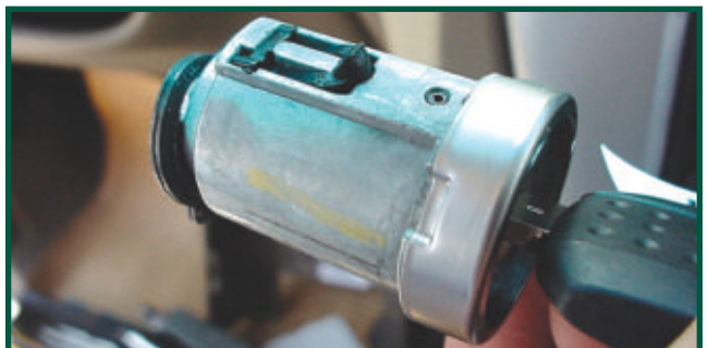
19. Needless to say, this retainer is simply a secondary retainer, holding the lock in place when the key is in the ON and START positions. To secure the lock in the housing, the snap ring at the back of the lock keys into the lock housing when the lock is in the OFF position.
