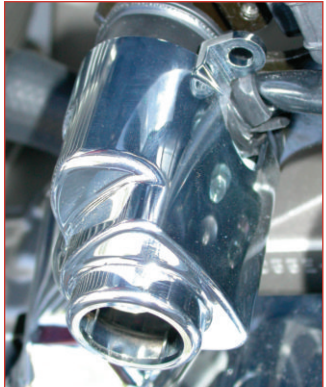
12. Pull the ignition lock cover off with a firm pull.
