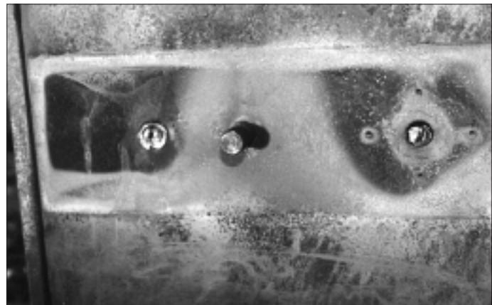
2. The melted dial and handle were removed, notice that the key lock has also melted.
