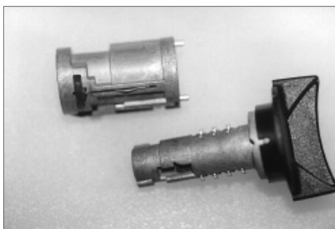
7. A disassembled ignition lock.
