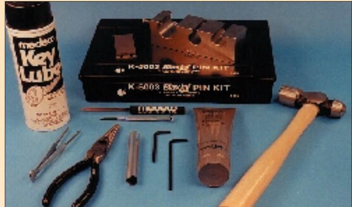
3. Tools needed for servicing the Medeco System Series padlock.
