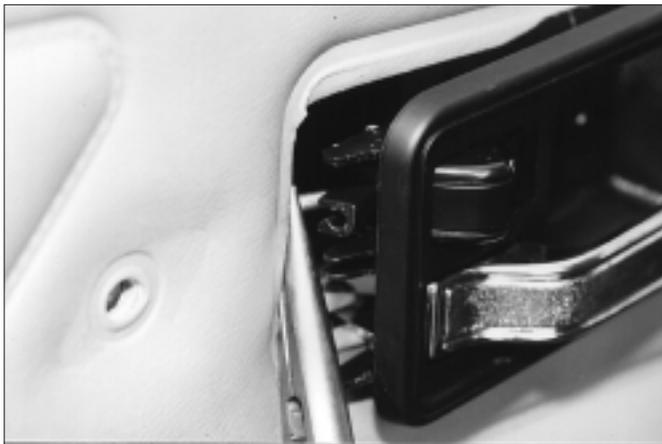
10. Remove the inside release/lock assembly.
