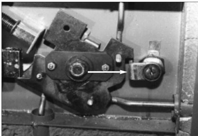
3. Interior configuration showing cam lock in the locked position.
