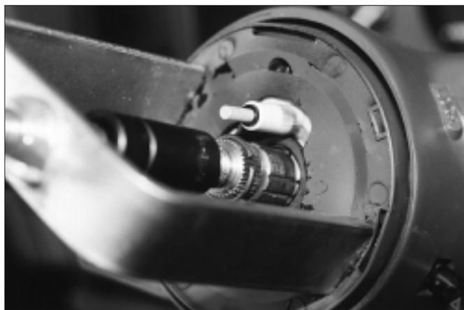
4. Removing the steering wheel lock plate.
