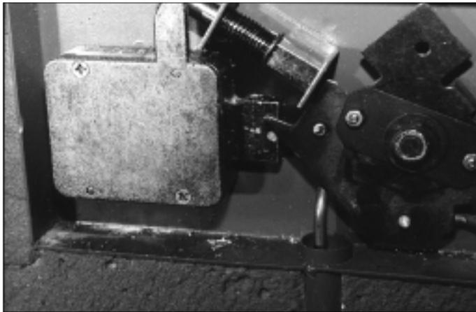
5. Locking plate bypassing the lock bolt opening safe door.
