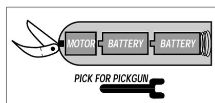
5. After removing the non moving blade, prepare the other blade for mounting the pick.
