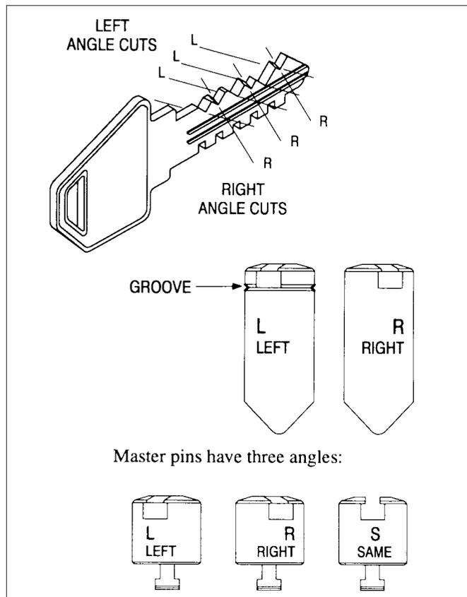
If Emhart High Security cylinders are to be incorporated into a master key system with conventional Corbin Russwin cylinders, it is best to create the master key plan with high security keys and cylinders in mind. Emhart High Security keys must have a minimum depth of 2. Remember, the high security bottom pins have chiseled points and must skew 20° right or left. A number 1 cut will not provide the necessary key slope to skew a pin tumbler. Thus, only five depths are available on a high security
