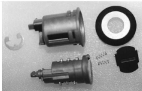
12. The disassembled door lock.
