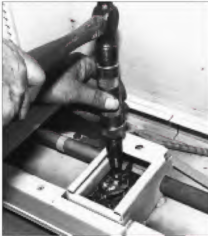
14. Some mounting screws must be removed with an impact driver.
