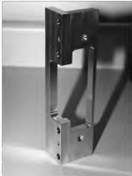
9. This template by Major Manufacturing allows you to cleanly cut frames for electric strike installation.
