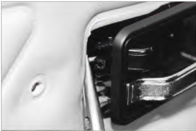
10. Remove the inside release/lock assembly.
