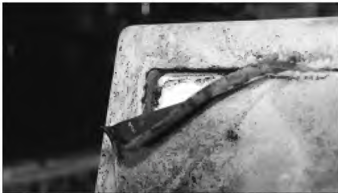
11. Corner Pried off safe door to exposed melted plastic door edge.
