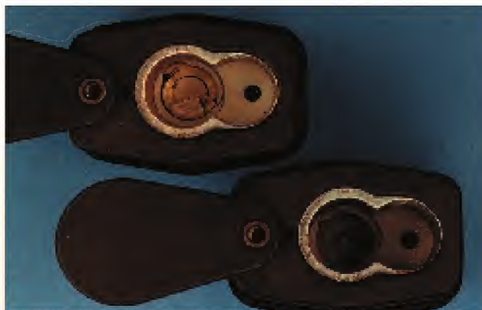
6. Looking into the bottom of the Medeco® padlock after the shackle, ball bearings and actuator are in place.
