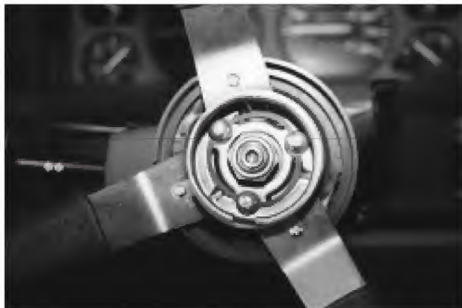
3. Remove the horn actuator assembly. Be careful not to damage the plastic insulating ring.
