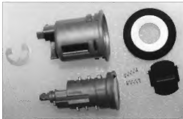
12. The disassembled door lock.
