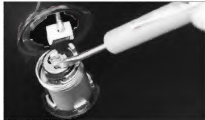
11. Instead of separating the linkage rod from the lock pawl, it is easier to remove the C-clip from the back of the lock and remove the lock from the pawl.
