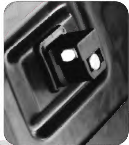
17. The glove box lock plug is removed after pulling back the two retaining tabs and sliding the plug out the front of the lock.
