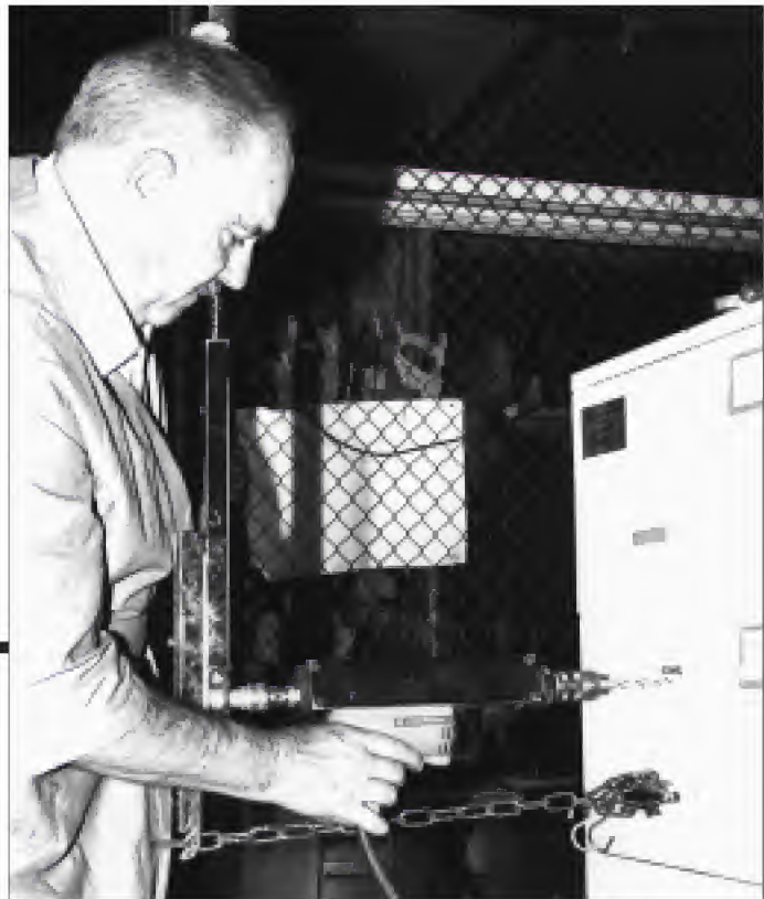
1. Drilling the hard plate with a pressure bar rig.
