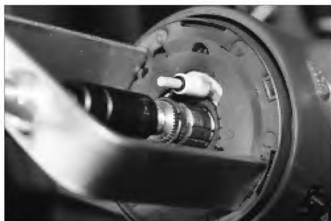
4. Removing the steering wheel lock plate.
