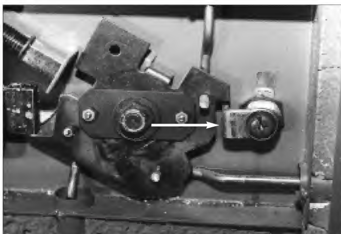
3. Interior configuration showing cam lock in the locked position.
