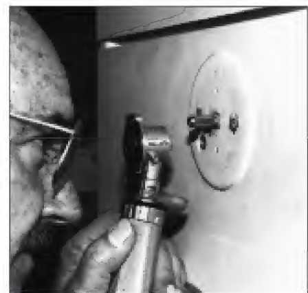
3. An otoscope helps to see into the hole. A simple pen light will do.
