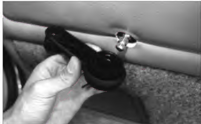
9. Unlike older version that were held on with a clip, this window crank is simply pressed on.
