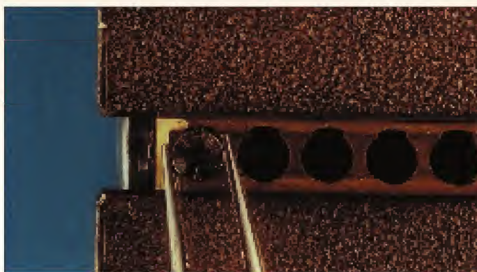
4. Drop the pin into the top of the chamber making sure the locator tab of the tumbler aligns with the locator slot of the pin chamber.
