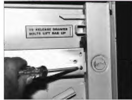
7. Two screws hold the drawer to the guide.
