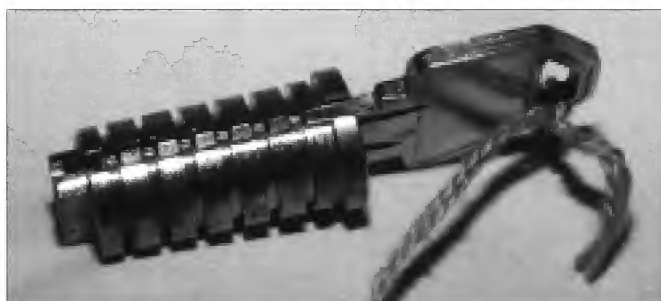
6. The grooves in the plug and the notches at the bottom of the key's blade are necessary to allow the interlocking tumblers to operate.
