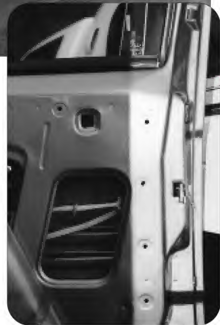
2. The inside of the door showing linkage and tool placement.
