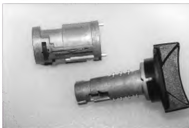
7. A disassembled ignition lock.
