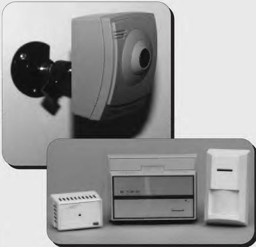
The CCD camera comes in various sizes and shapes. Its compact nature allows it to be stored in false thermostat and alarm device packages for covert recording.
