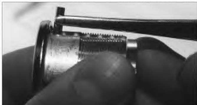
9. After interconnecting the pins, load them into the cylinder.
