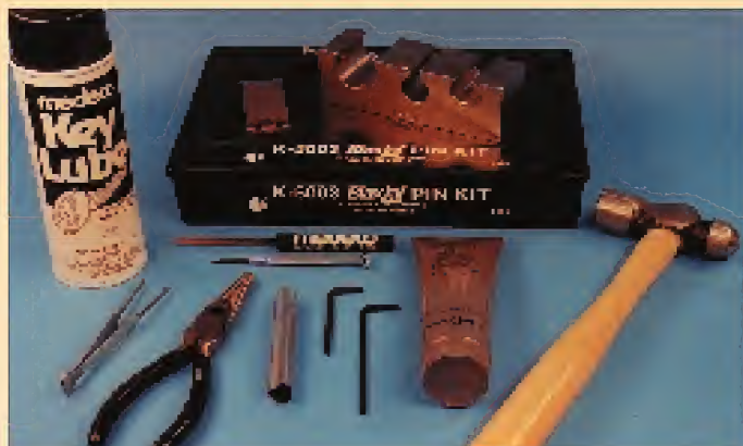
3. Tools needed for servicing the Medeco System Series padlock.
