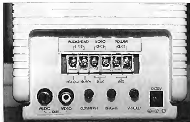
9. The back of the monitor is clearly marked for wire connection.
