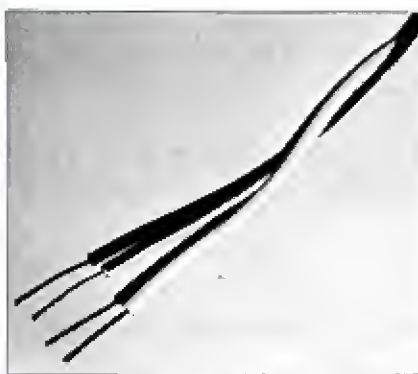
3. Twisted pair is a common wire for alarm and access control use. The twisting of the wires reduced problems caused by RFI or radio frequency interference.
