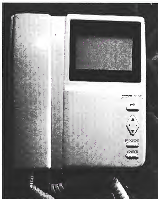
2. The MY-1CD control station includes a monitor and controls to pan/tilt the camera, activate the intercom and unlock a remote lock.
