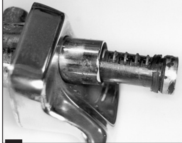
20. The cylinder plug will now slide out the front of the handle.
