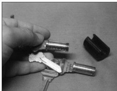
2. The high security Primus cylinders always had 6 conventional pin chambers.
