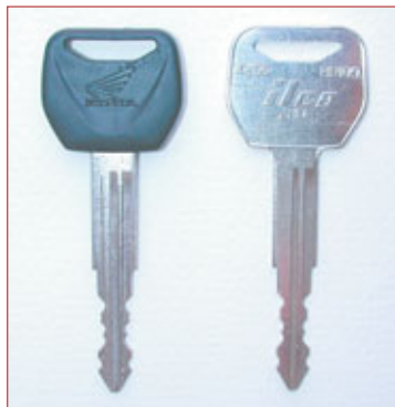
6. The original key is on the left with the duplicate on the right. A code cut X265 key blank with cuts of 1 1 3 2 3 3 1 2 operates all three locks on this motorcycle.
