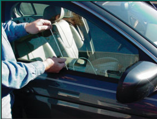
4. Pull the tool up until the tip is free of the weather-stripping.
