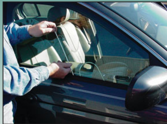
5. Lever the handle out to unlock the door.
