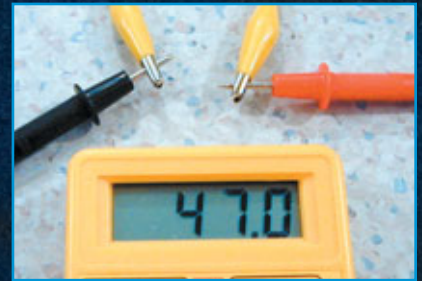
7. These are even worse. They have a resistance of 47 ohms.
