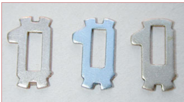
21. From left to right are ignition lock wafers with depths of 1, 2 & 3. These are unique wafers and I am unable to find a keying kit for them. The gas cap and seat locks use the ASP A-19-101 keying kit, which is also used on Honda automobile door and trunk locks throughout the 80's.
