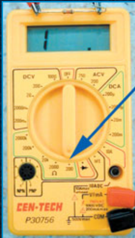
17. When measuring 12,000 ohms while in the 200 scale, the display shows infinite.
