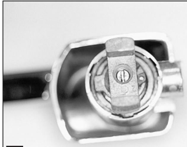
18. The tailpiece is set to a particular position so it can interact with the latch mechanism in the door. To remove the tailpiece you will need to turn the stud bolt in the center of the tailpiece. Turn the stud bolt counter-clockwise. This is the important part: count exactly how many turns you make when unscrewing the stud bolt. If you don't put the tailpiece back in the same position it will not line up with the latch correctly and will have to be reset.
