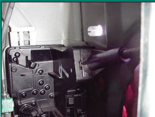
2. The latch and the attachment point for the single cable is totally shielded.
