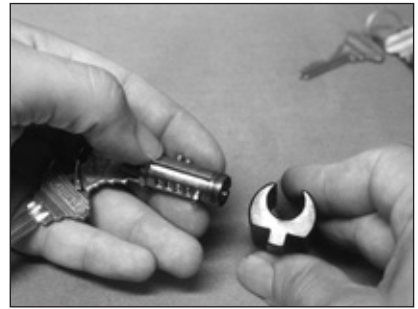
5. The fifth finger pin is coming out of the Primus plug.
