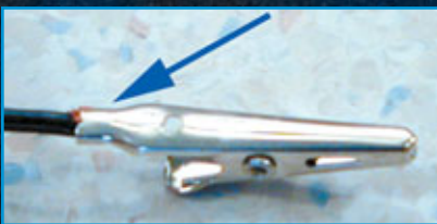
8. The alligator clips had bad crimped connections from the factory.
