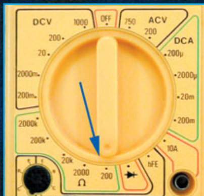
1. Before you can start measuring stuff, you need to test your multimeter.
