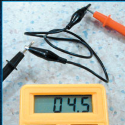
6. This pair of alligator clips is not in very good condition. They read 4.5 ohms.
