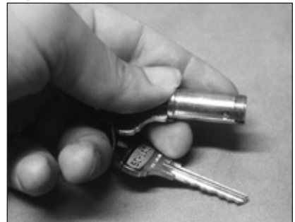
7. An Everest key holding the check pin inward.
