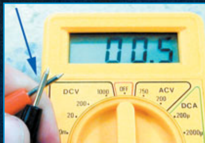
3. Something in the area of 0 to 2 ohms is OK when the test leads are touching. Here we have .5 ohms.
