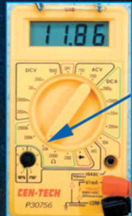
19. On the 20K scale, we get a reading of 11.86 which when multiplied by 1000 is equal to 11,860.
