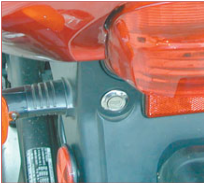
4. The seat lock is located on the back of the rear fender by the taillight. It contains five wafer tumblers in spaces 2-6.
