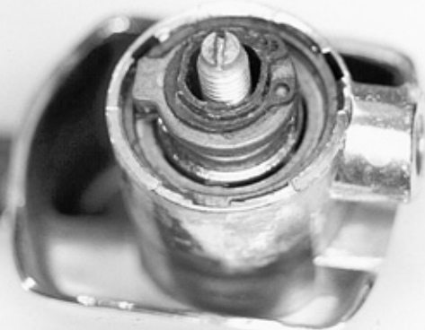
19. The plug and plug spring are held in place by a "tru-arc" ring that must be removed.
