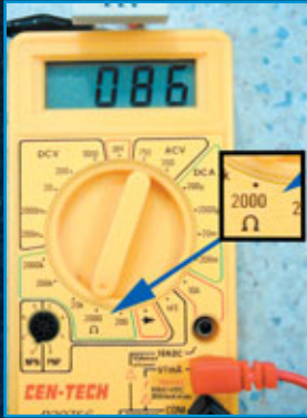
14. Doing the same test but on the 2000 ohm scale we get 86 ohms of resistance.
