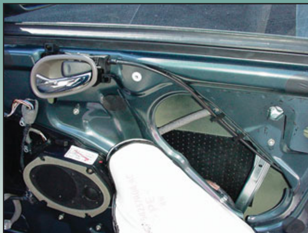
3. A bicycle-style cable connects the inside handle to the latch mechanism.
