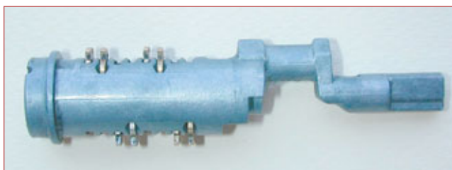
20. The ignition lock contains all 8 wafer tumblers staggered in pairs.
