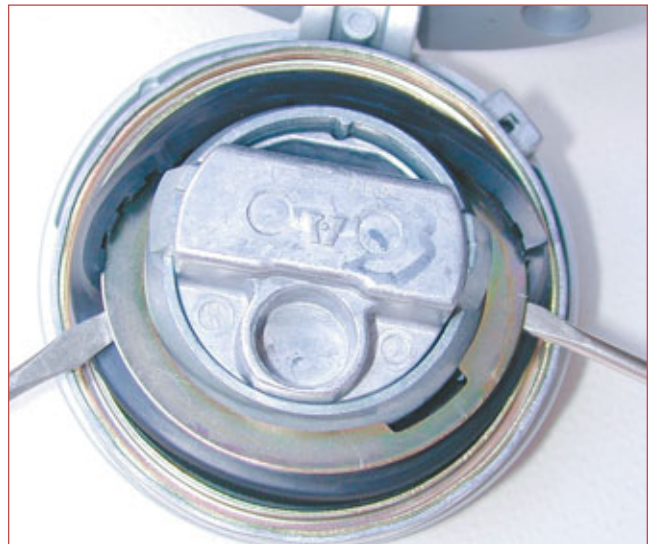
8. Remove the gasket backing ring using two small screw-drivers as shown in the photograph. It is similar to removing a bicycle tire from its rim. It is tricky to replace the ring behind the gasket during reassembly but it can be done. There is a cutout on the inside of the backing ring that is visible in the photograph at the 5 o'clock position. The purpose of this cutout is to allow the ring to slide over the locking bolt if the bolt is extended in the locked position.
