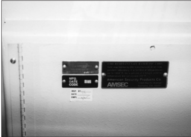
3. Piano hinge on the inside access door with screws removed to allow access.
