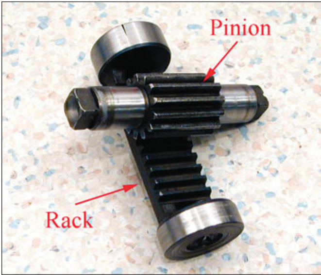
5. The piston and shaft or "rack and pinion" are the two parts used to convert the rotary movement of the arm to the spring compressing force of the piston.
