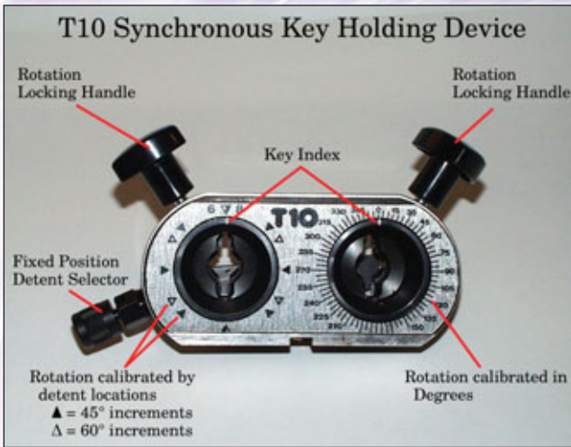
7. The T10 Synchronous Key Holding Fixture.
