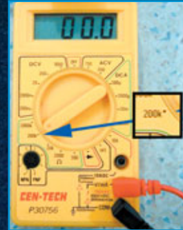
16. The 82 ohms is too small to see when using the 200K scale. The display reads 0 ohms.
