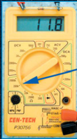
20. The 200K scale shows a reading of 11.8 which converts to 11,800.
