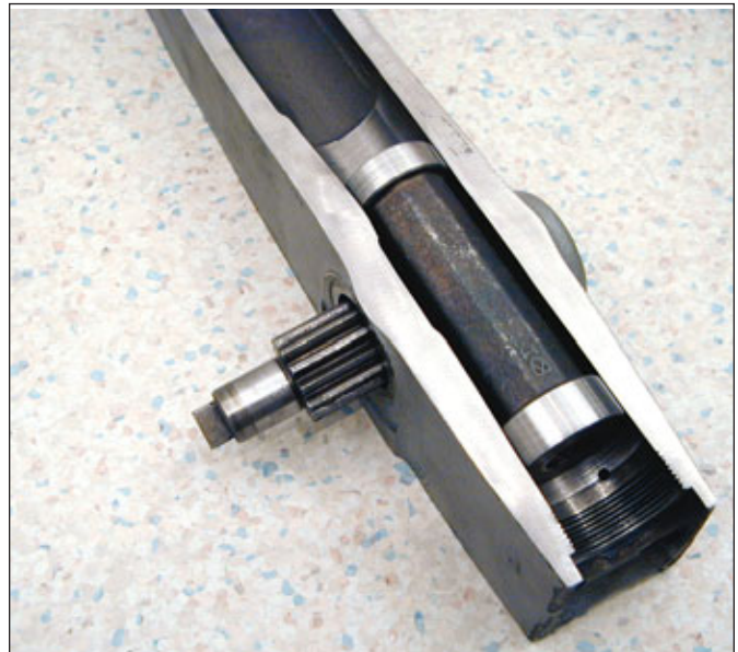
6. The piston and shaft are mated in the closer body.
