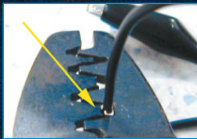
9. Re-crimping the connections should fix the problem.
