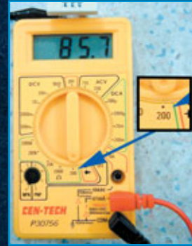
13. The 200 ohm scale is used first. We get 85.7 ohms.
