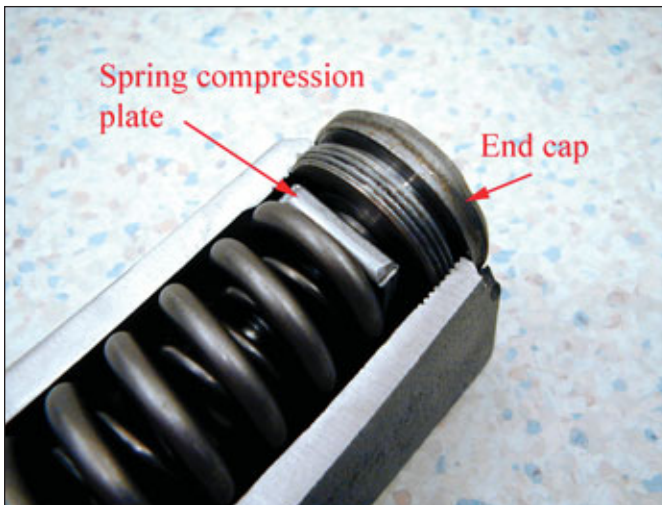
9. The spring adjuster set to provide the least amount of power.
