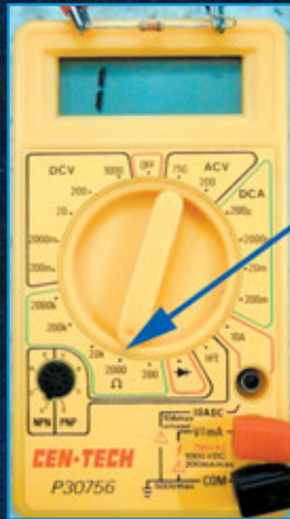
18. Infinite is also displayed in the 2000 scale.
