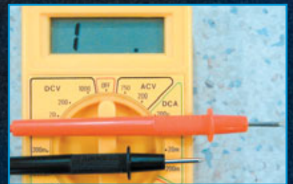
2. An infinite indication on the display is what you should get if the test leads are not touching.
