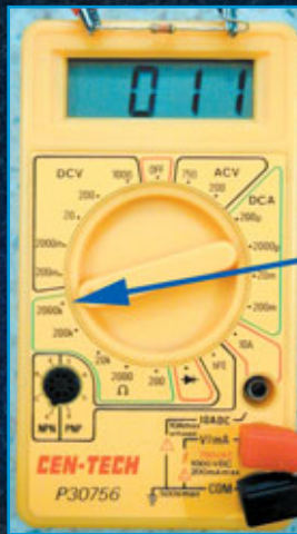
21. The largest scale is the least accurate when measuring a small amount. The 2000K is meant to measure 2,000,000 ohms or less.
