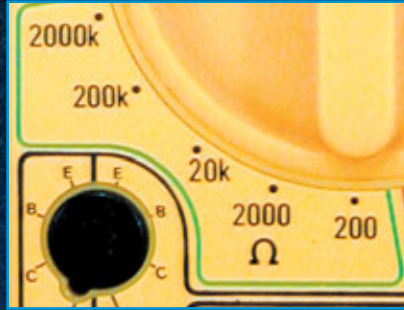
12. There are several scales to choose from when checking resistance. This multimeter has five different scales.
