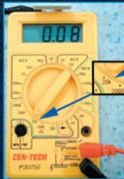
15. Things make a big change when using the 20K scale. The reading has to be multiplied by 1000. The .08 is the same as 80 ohms.
