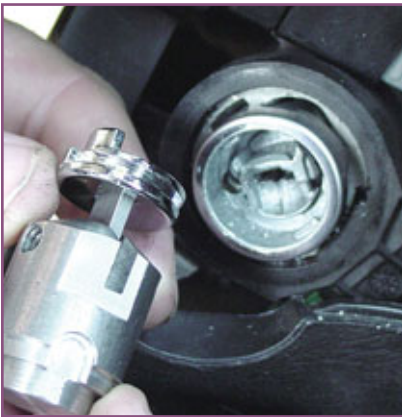
11. Use the thick key blade guide to remove the face of the plug.
