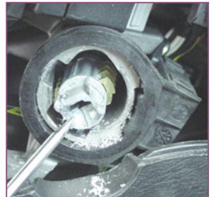
16. This action will leave the plug intact within the ignition housing itself.
