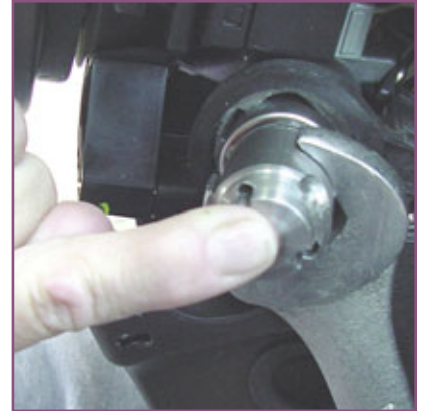
10. With a 7/8" or adjustable wrench, apply a firm and steady "clockwise" turning pressure.
