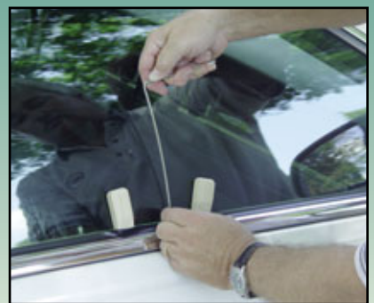
7. Pull up and forward at the same time in order to unlock the door.
