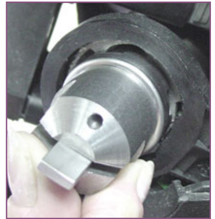
13. The force tool/drill guide is inserted into the cavity.
