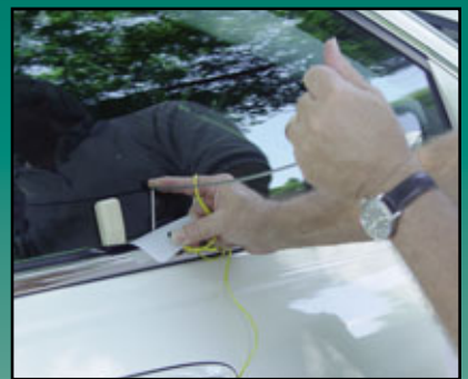
5. Carefully insert the hooked end of the tool into the door using the plastic card to protect the weather-stripping.
