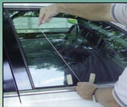
6. Rotate the tool and lower the hooked end of the tool into the door to grasp the vertical linkage rod.
