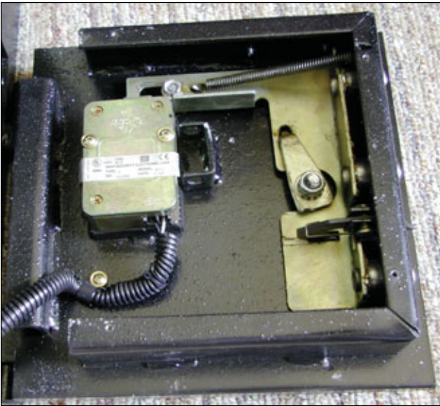
3. Because this is a cash control system and not a high security system, you will not find a relocker inside the door.
