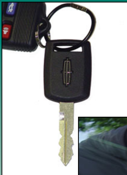
2. The Strattec 691259 E-PATS key that is used on the 2003 Lincoln Town Car.
