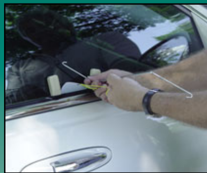
4. Wedge open the door above the forward end of the outside door handle.
