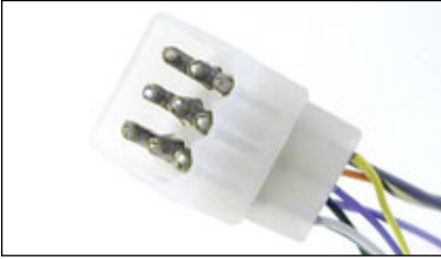
10. The circuit card is connected to the wiring harness through a molex style connector.
