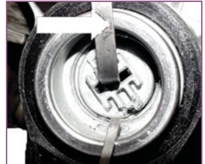
19. Once picked, apply the same turning tension as on the other examples and slowly remove the sidebar pressure tool.
