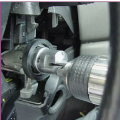
14. Drill through the 3/16" guide hole with arbor #2, until the arbor hits the block.
