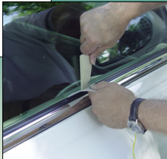
3. Use a plastic card inserted between the weather-stripping and the glass to protect the weather-stripping from damage as you insert the wedge and the tool.
