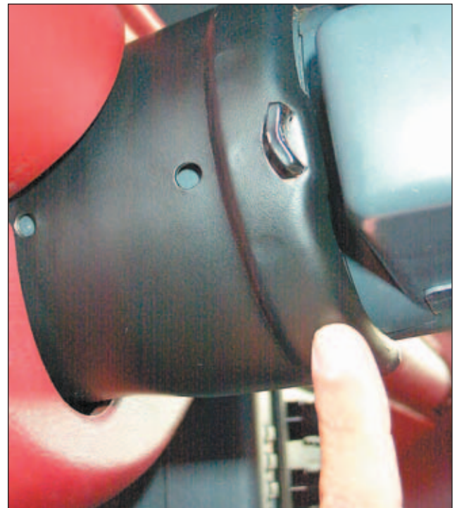
7. Rotate the shield clockwise.
