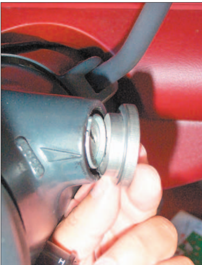
14. Install the alignment ring.
