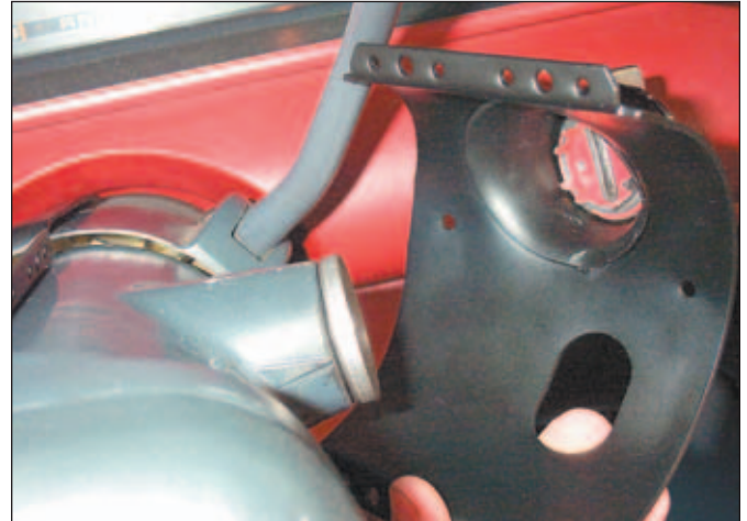
15. Install the right housing.
