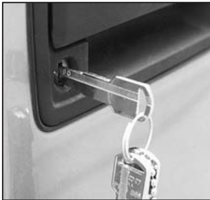
12. The key trapped on tumbler position #8.
