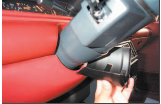
6. Insert the shield between the dash.
