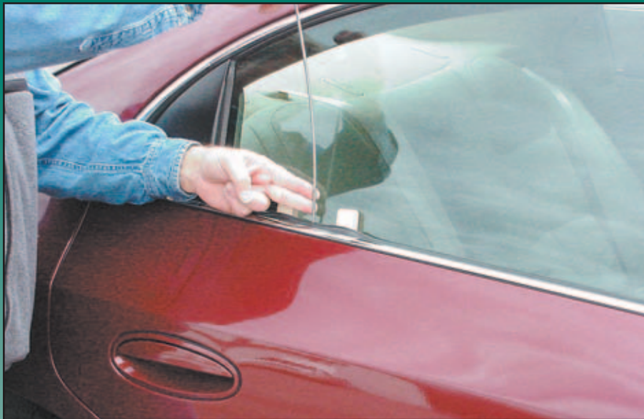
3. Once the tool is on the linkage rod, lever the linkage toward the front of the car to unlock the door.
