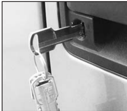
14. The key is trapped on the tumbler in position #9.
