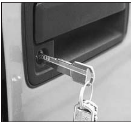
13. The key trapped on tumbler position #6.
