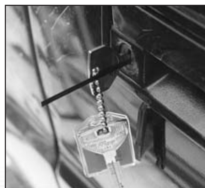
7. The spring steel slide tool dislodges the trapped tumbler.
