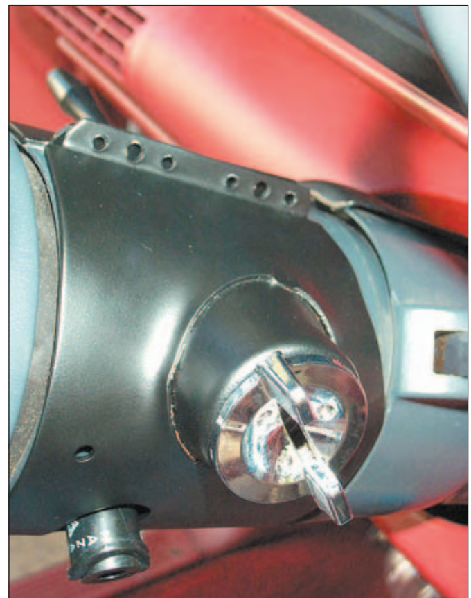
16. Rotated to the "lock" position.
