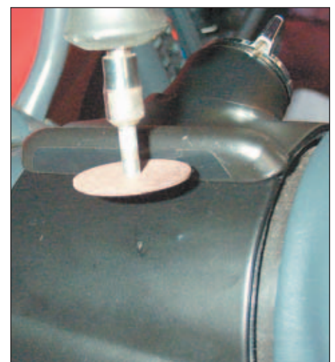
22. Grind away the cap.
