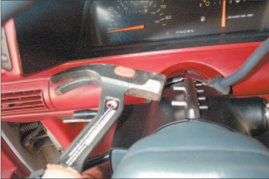
17. Two large alignment pins.
