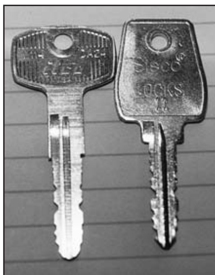
5. X114 (DA24) duplicate and original Sisco #11 bypass key.
