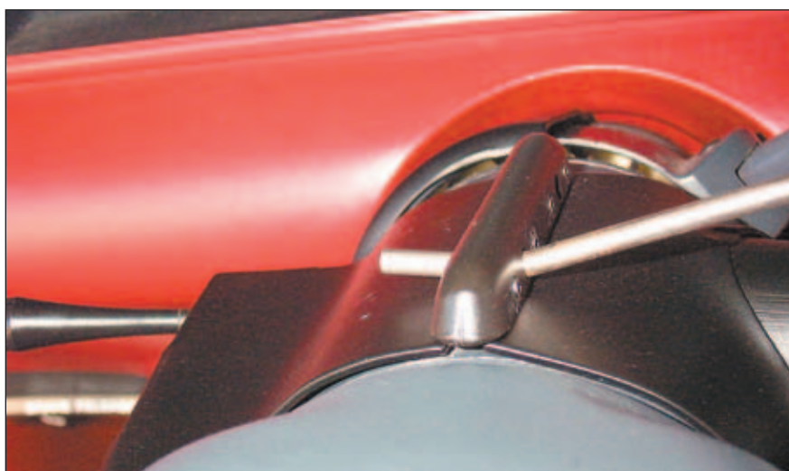
19. Hammer in the roll pins on the cap.
