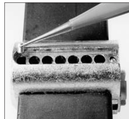
3. Installing patent bottom pin.
