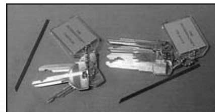
2. Decoder keys known as The Determinator.
