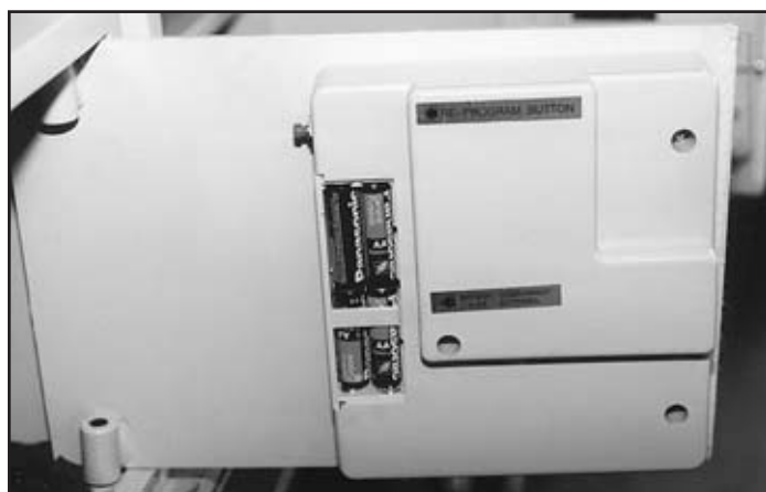
4. Four AA battery compartment and combo reset button.
