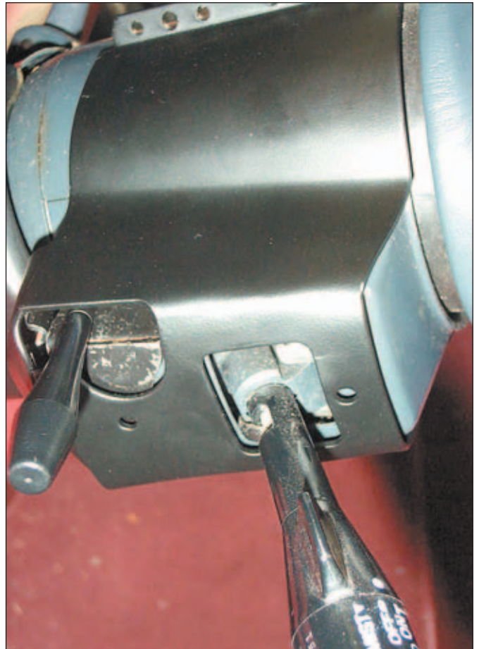
11. The housing installed on the column.
