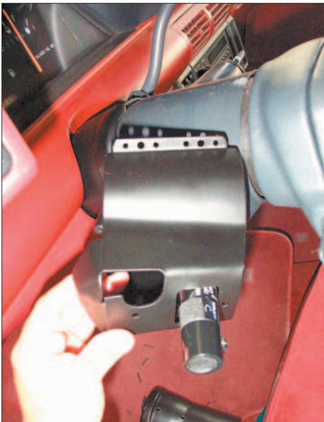
10. Install the left housing.
