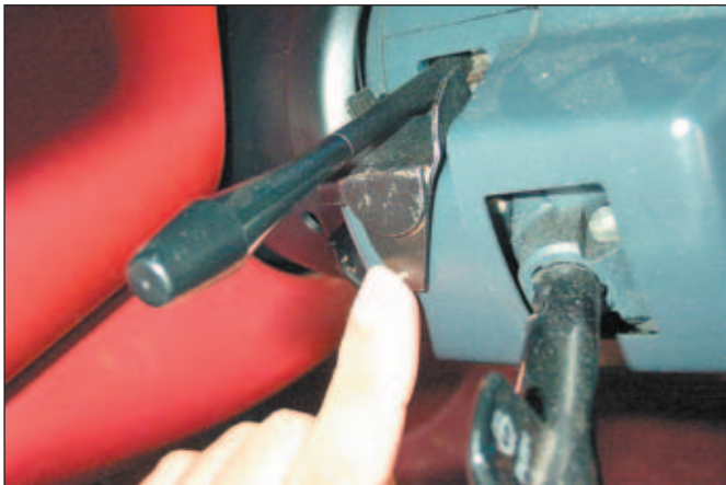
9. The bracket installed.
