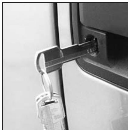
15. The key is trapped on the tumbler in position #7.
